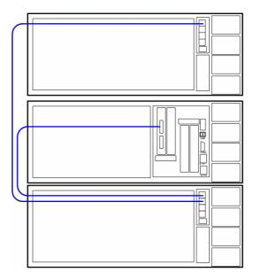
Figure 1-28 Cable Guide – Single Server with two JBODs daisy-chained
