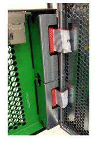
3. Plug the ribbon cable(s) into their corresponding control panel socket (Figure 1-4).
