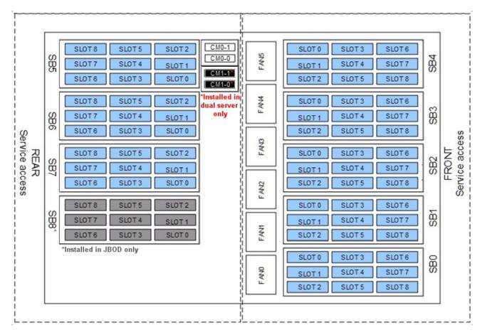
Figure 1-23 System Layout Diagram – Drive & Fan Placement
