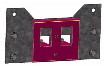
Figure 1-8 D-Rack Stiffener Adjustment Plate
