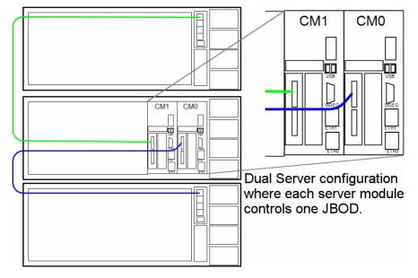
Figure 1-37 Cable Guide – Dual Server with two JBODs
