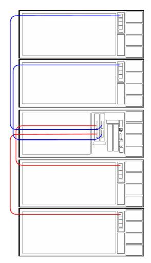
Figure 1-33 Cable Guide – Single Server, Dual HBA, four JBODs
