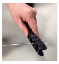
Figure 1-46 Pry the Joint Apart
