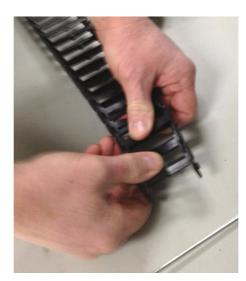
Figure 1-47Pull the Segments from the Arm
