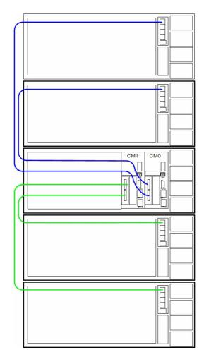
**Figure 1-40** Cabling Guide – Dual Server with four JBOD split
