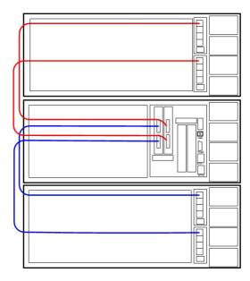
Figure 1-30 Cable Guide – Single Server with 2 HBAs, 2 JBODs with Dual I/O, split
