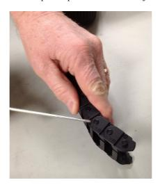
For the first method, segments are removed from the *end* of the arm. Use the flat-head screwdriver and slip it between the plastic pieces that form the joint of the arm (Figure 1-45).
