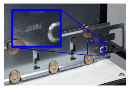
Figure 1-17 Align Rails to Front
