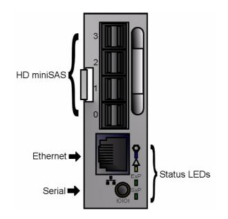
Figure 1-25 JBOD I/O Module Port Diagram
