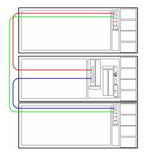
Figure 1-27 Cable Guide – Single Server with two JBODs Shared
