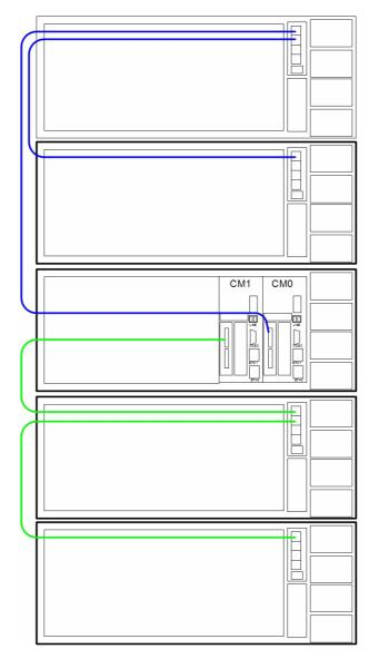
Figure 1-39 Cable Guide — Dual Server with four JBODs
