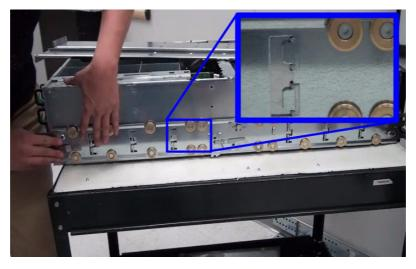
Figure 1-19 Lock on to Support Tabs
