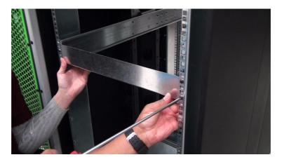
Figure 1-14 Adjustment Using the Alignment Tool
