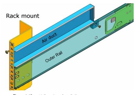
Figure 1-16 Air Duct above Outer Rail
