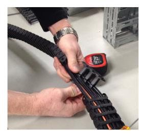
Once complete, separate the section of unwanted segments from the cables by twisting the section off (Figure 1-53).
