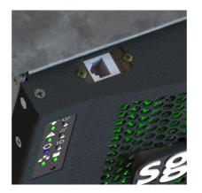
Figure 1-60 MIS-S9D Proprietary Network Interface
