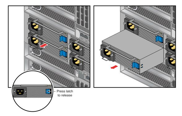
Figure 7-1 Removing an Enclosure Power Supply
