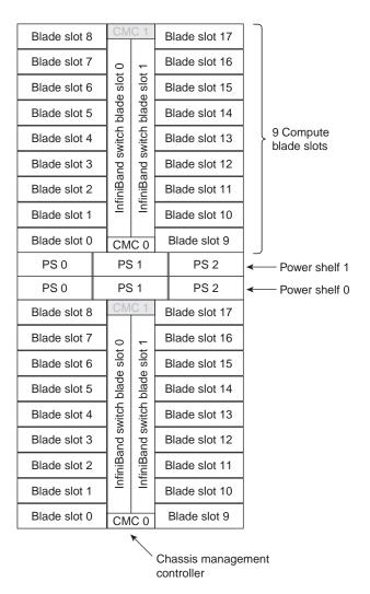
Figure 3-9 Single-node D-Rack Blade Enclosure Pair Component Front Diagram
