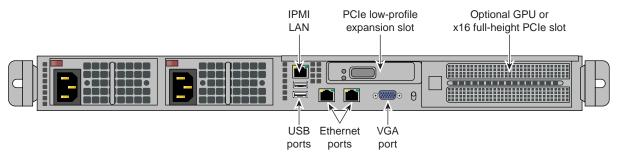
Figure 5-3 SGI Rackable C1104G-RP5 1U Service Node Front and Rear Panels
