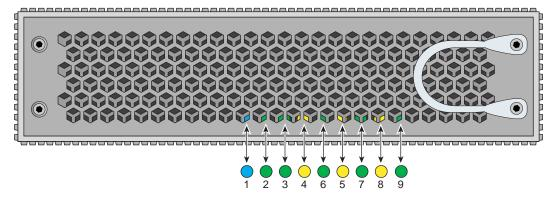
Figure 6-2 IP113 Compute Blade Status LED Locations Example
