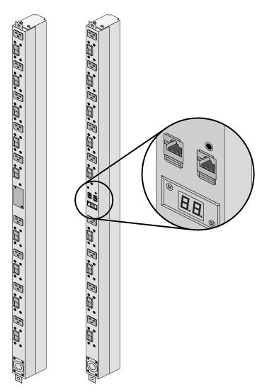
Figure 1-5 Three-Phase PDU Examples
