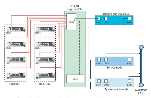
Figure 2-3 Non-redundant Chassis Manager Interconnection Diagram Example
