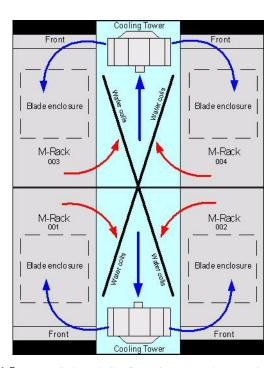
**Figure 4-5** M-Cell Rack Configuration Example (Top View)
