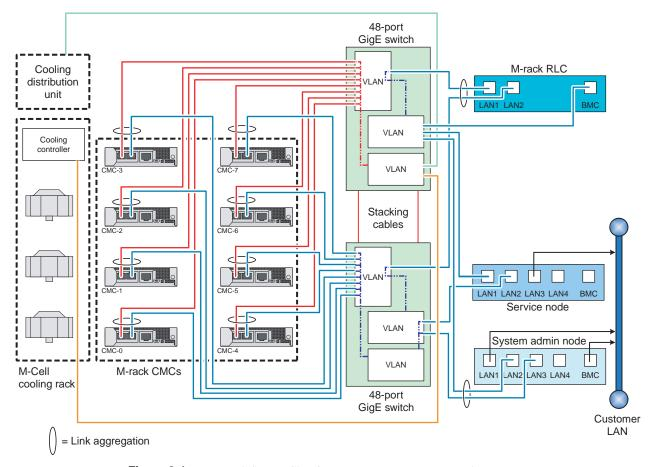
Figure 2-4 M-rack System Chassis Manager Interconnect Example
