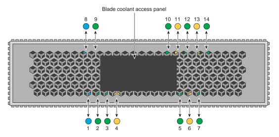
Figure 6-3 IP115 Compute Blade Status LEDs Example
