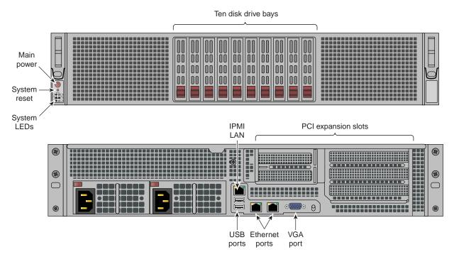
**Figure 5-8** Front and Rear Views of the SGI Rackable C2110G-RP5 2U Service Node
