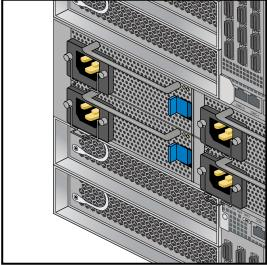
**Figure 7-2** Replacing an Enclosure Power Supply
