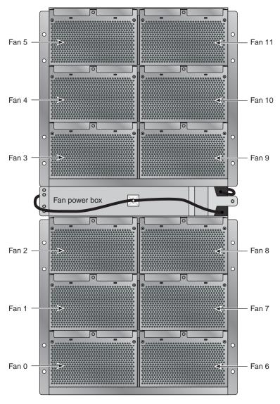
Figure 7-3 Enclosure-Pair Rear Fan Assembly (Blowers)
