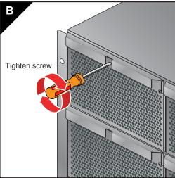
Figure 7-5 Replacing an Enclosure Fan
