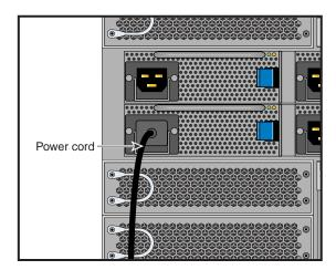
Figure 1-3 Blade Enclosure Power Supply Cable Example
