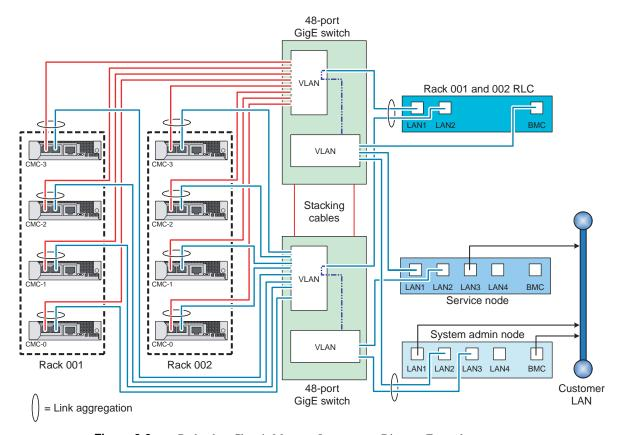
Figure 2-2 Redundant Chassis Manager Interconnect Diagram Example
