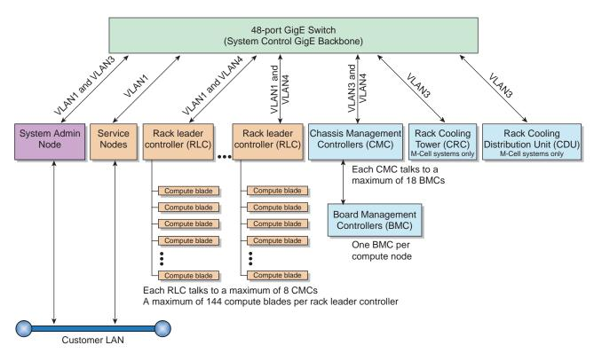
Figure 5-1 SGI ICE X System Administration Hierarchy Example Diagram
