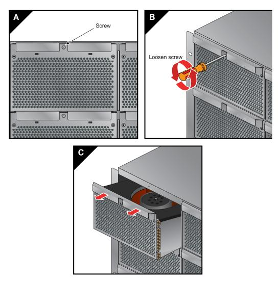
**Figure 7-4** Removing a Fan From the Rear Assembly
