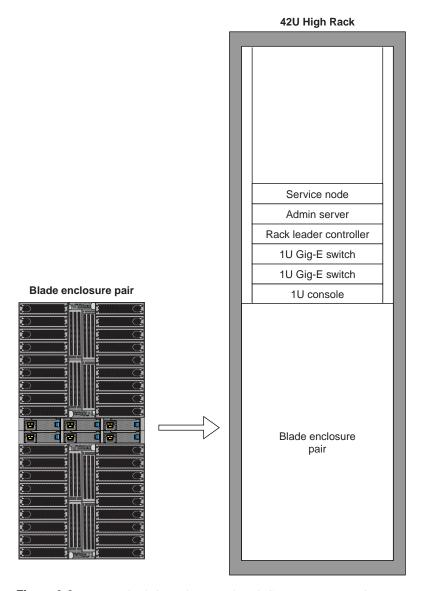
Figure 3-2 D-rack Blade Enclosure and Rack Components Example
