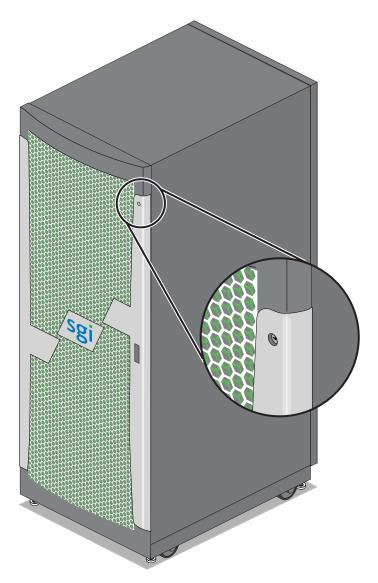
Figure 4-2 Front Lock on Tall (42U) D-Rack
