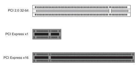
Figure 7-8 Comparison of PCI/PCI-X Connector with PCI Express Connectors
