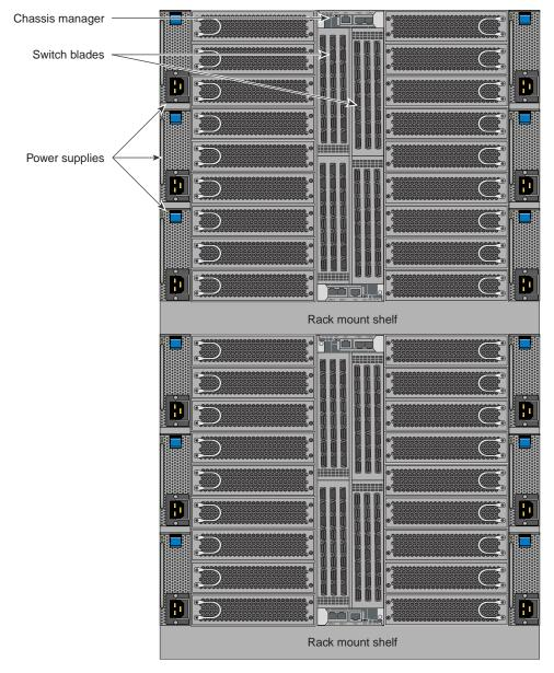
**Figure 3-10** M-Rack Blade Enclosure Pair Components Example
