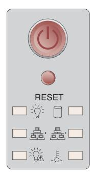
Figure 5-9 SGI Rackable C2110G-RP5 2U Service Node Control Panel Diagram
