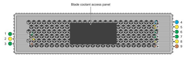
Figure 6-4 IP119 Blade Status LEDs Example
