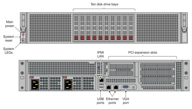
Figure 3-7 2U Service Node Front and Rear Panel Example
