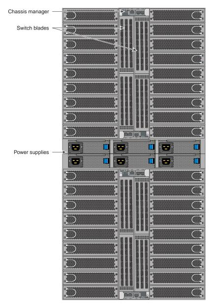
Figure 3-8 SGI ICE X Series D-Rack Blade Enclosure Pair Components Example
