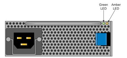
Figure 6-1 Power Supply Status LED Indicator Locations
