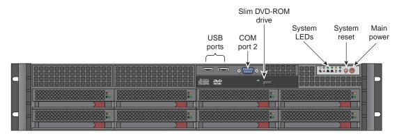
Figure 5-3 Front View of 2U Service Node
