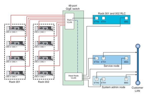
Figure 3-4 Administration and RLC Cabling to Chassis Managers Via Ethernet Switch
