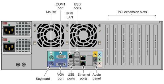
Figure 3-7 3U Service Node Rear Panel Example
