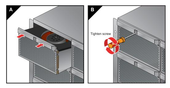
Figure 7-5 Replacing an Enclosure Fan
