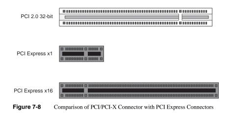
PCI Express technology uses two pairs of wires for each transmit and receive connection (4 wires total). These four wires are generally referred to as a lane or x1 connection (also called "by 1"). SGI administrative node PCIe technology uses x16, x8 and x4 connector technology in the PCI Express card slots (see Figure 1-2 on page 4 for an example). The PCIe technology will support PCIe boards that use connectors up to x16 in size. Table 7-2 shows this concept.
