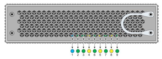
Figure 6-2 Compute Blade Status LED Locations Example
