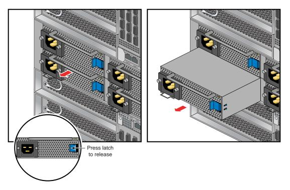
Figure 7-1 Removing an Enclosure Power Supply
