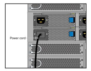
Figure 1-3 Blade Enclosure Power Supply Cable Example
