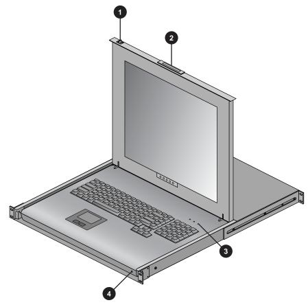
Figure 1-1 Flat Panel Rackmount Console Option
