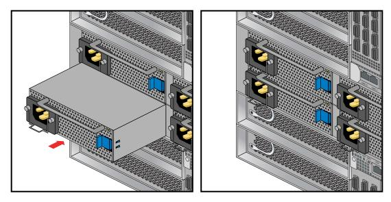
Figure 7-2Replacing an Enclosure Power Supply
