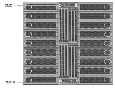
Figure 1-6 Blade Enclosure Chassis Management Board Locations
