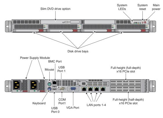
Figure 5-2 1U Rack Leader Controller (RLC) Server Front and Rear Panels
