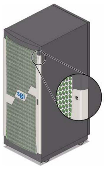
Figure 4-2 Front Lock on Tall (42U) Rack
