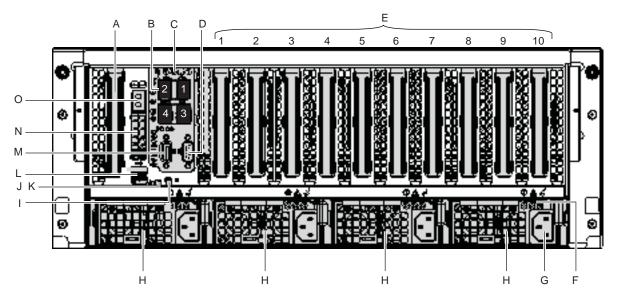
Figure 3-84U Service Node Rear Panel Example
