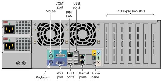
Figure 5-7 SGI 3U Service Node Rear View
