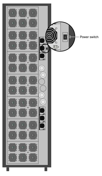
Finally, press the enable power switch to On (|) on the rear of the enclosure, see Figure 2-2 for an example.
