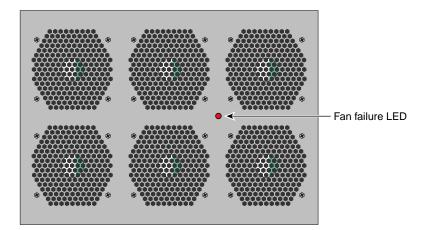
Figure 2-5Fan Failure LED Location Example
