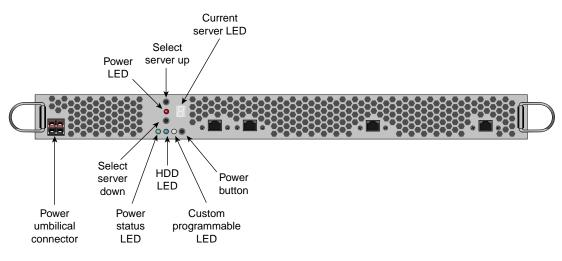
Figure 2-4 Example Compute Tray Status LEDs and Switches
