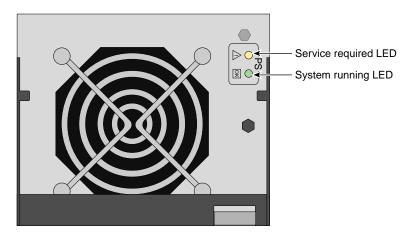
Figure 2-3 System Power Supply Status LED Locations
