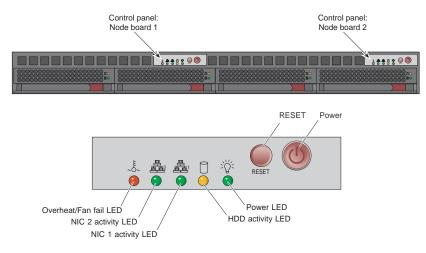
Figure 1-2 SGI Altix XE320/XE340 Compute Node Controls and Indicators
