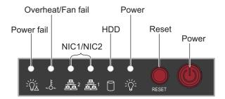
Figure 1-1 SGI Altix XE250 or XE270 Front Control Panel
