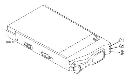
Figure 1-10 Disk Drive Indicator LEDs
