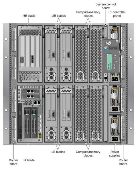
Figure 1-1 Compute Appliance Front Panel Components Example
