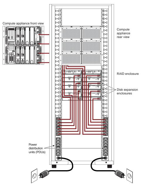
Figure 1-4 Connection Example of a Racked System to Power
