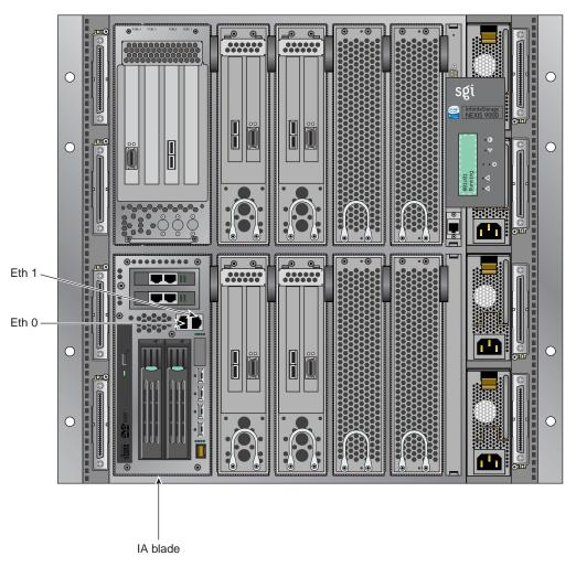
Figure 1-5 Ethernet Connection to Compute Appliance
