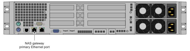
Figure 1-5 Primary Ethernet Connection to NAS Gateway
