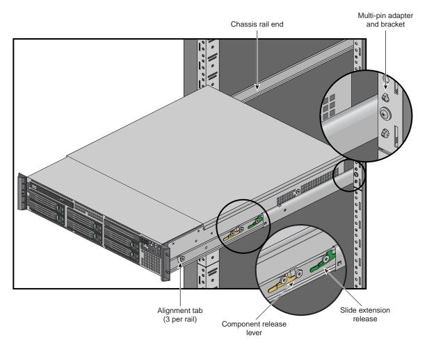
Figure 1-9 NAS Gateway Slide Rails
