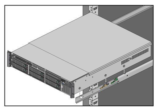
Figure 1-8 NAS Gateway Slide Rail Mounting Stud Positions
