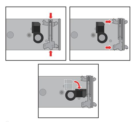
Figure 1-7 Reversing the Rail Pin Adapter
