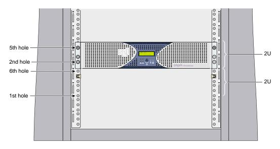
Figure C-4 Mounting-hole Pattern of Rack Vertical Rails
