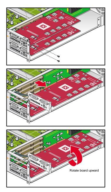
**Figure A-16** Removing the Graphics Card Assembly
