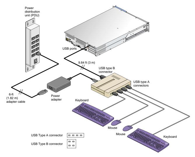
Figure 3-8 Using a USB Hub to Connect Multiple Keyboards and Mice to Host System (USB Hub May Differ From Illustration)
