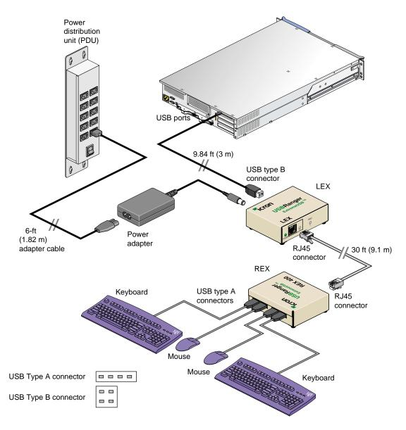
Figure 3-9 Using a USB Extender to Connect Keyboards and Mice
