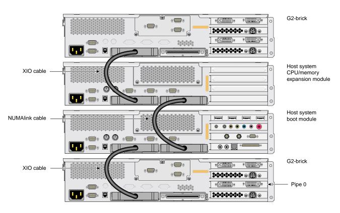
Figure 2-6 shows a configuration containing two host bricks and two G2-bricks.
