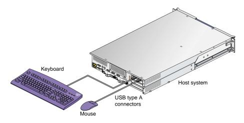
Figure 3-7 Connecting a USB Keyboard and Mouse to a Host System
