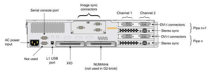
Figure 1-2 SGI Onyx4 G2-brick and G2N-brick Rear Panel
