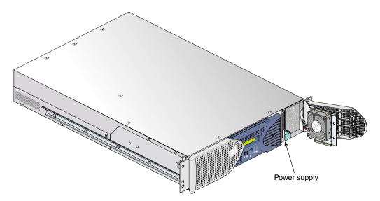
Figure A-2 Power Supply Location
