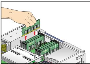
Figure A-10 Removing a DIMM
