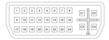
Figure B-3 DVI-I Connector Pinout
