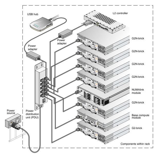
Figure 2-12 Connecting an Onyx4 Racked System to Power
