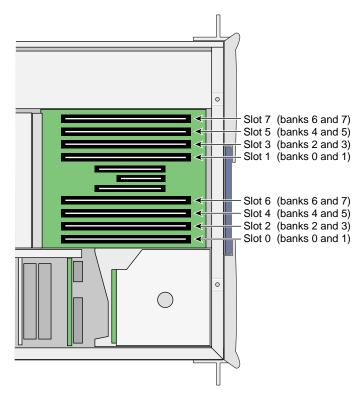
Figure A-6 Layout of DIMM Slots and Local Memory Banks
