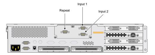
Figure 2-9 ImageSync Connectors on G2-brick and G2N-brick
