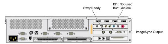
Figure 3-12 ImageSync Card Connectors
