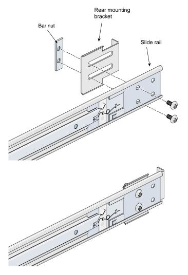
Figure C-2 Attaching the Rear Mounting Bracket to the Slide Rail
