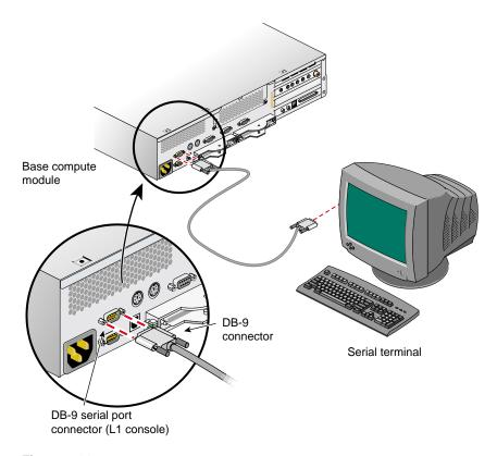
Figure 2-14 Connecting a Serial Terminal to an L1 Controller
