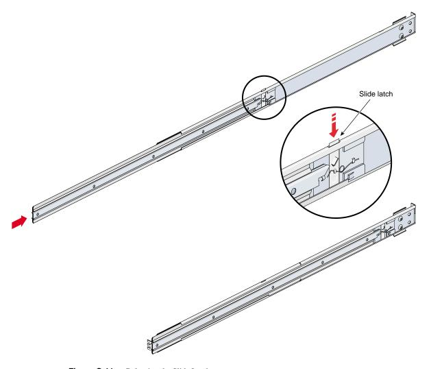
Figure C-11 Releasing the Slide Latches
