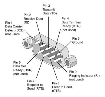
Figure B-1 DB9 Connector Pin Assignments
