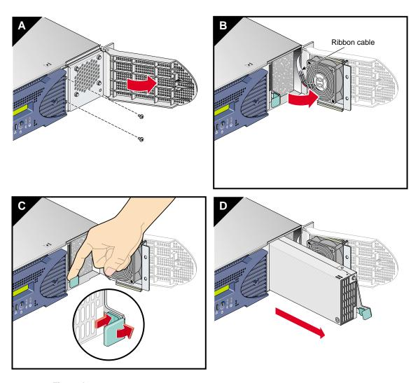
Figure A-3 Removing the Power Supply
