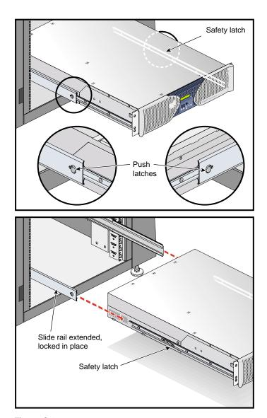
Figure C-10 Releasing the Safety Latches
