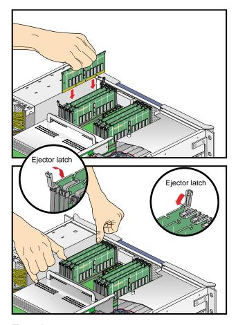
Figure A-8 Inserting a DIMM
