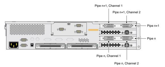
Figure 3-4 Monitor Connections on G2-bricks and G2N-bricks
