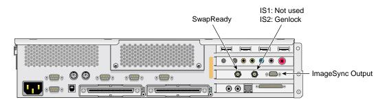
Figure 2-8 SGI ImageSync Card Connectors (Genlock on IS2 Card Only)
