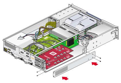
Figure A-19 Replacing the PCI/PCI-X Support Bracket
