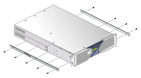
Figure C-3 Attaching Chassis Rails to the Brick
