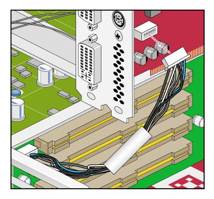
Figure A-17 Synchronization Cable Connection on Underside of Graphics Card
