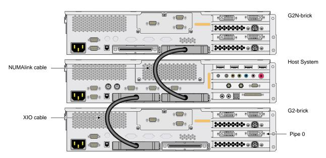
Figure 2-4 shows a configuration containing one host brick, one G2-brick, and one G2N-brick.
