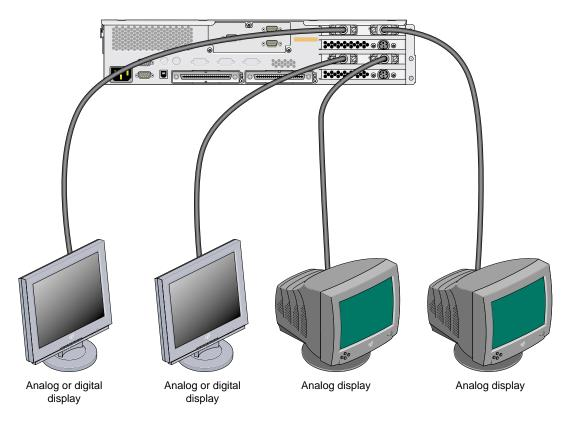
Figure 3-5 Connecting Monitors to a G2-brick or G2N-brick (SG2 Graphics Cards)
