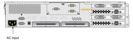
Figure 2-11 SGI Onyx4 G2-brick and G2N-brick AC Input
