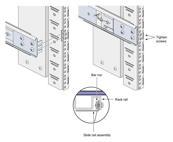
**Figure C-6** Attaching the Slide Rail to the Rack
