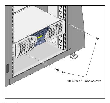
Figure C-9 Securing the Brick to the Rack
