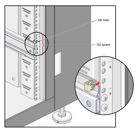
Figure C-7 Installing Clip Nuts in Rack Rails
