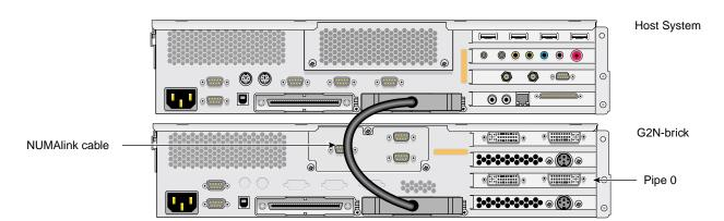
Figure 2-3 shows a configuration containing one host brick and one G2N-brick.
