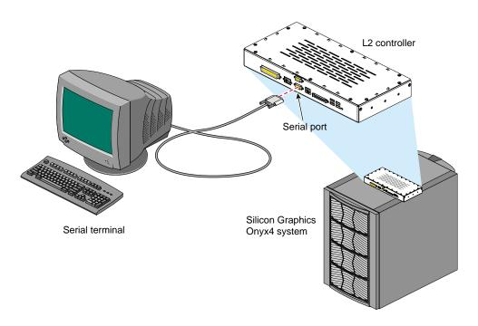
Figure 2-13 Connecting a Serial Terminal to an L2 Controller
