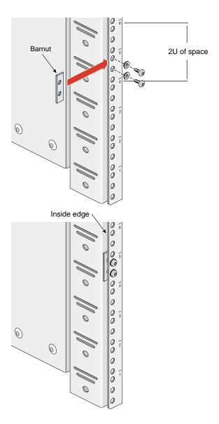
Figure C-5 Placing the Bar Nuts on the Rack Rails
