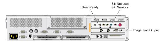
Figure 3-11 ImageSync Card Connectors
