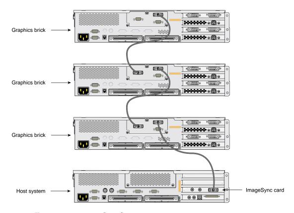
Figure 2-10 Cabling an ImageSync card to G2-bricks and G2N-bricks
