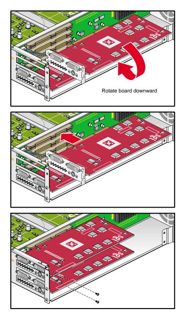
Figure A-18 Installing the Graphics Card and Retaining Screws
