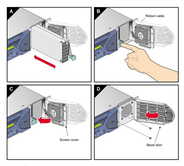
Figure A-4 Installing the Power Supply
