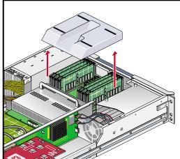
**Figure A-9** Removing the Plastic Air Baffle
