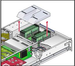
**Figure A-7** Removing the Plastic Air Baffle
