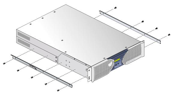
Figure A-14 Removing Chassis Rails from the Brick
