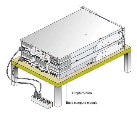
Figure 2-1 Positioning a Non-Racked Onyx4 System
