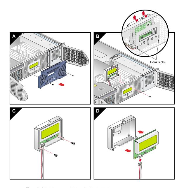
Figure A-12 Removing an L1 Controller Display Panel
