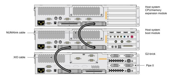
Figure 2-5 shows a configuration containing two host bricks and one G2-brick.
