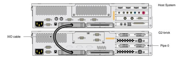
Figure 2-2 One Host Brick with One G2-brick
