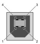
Figure B-2 USB Type B Connector Pin Number Locations
