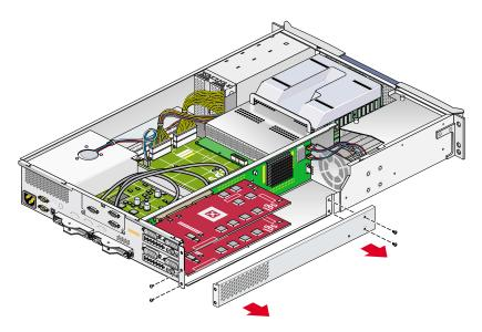
Figure A-15 Removing the PCI/PCI-X Support Bracket
