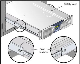
Figure C-8 Pressing the Safety Latches
