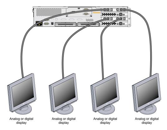
Figure 3-6 Connecting Monitors to a G2-brick or G2N-brick (SG2.1 Graphics Cards)
