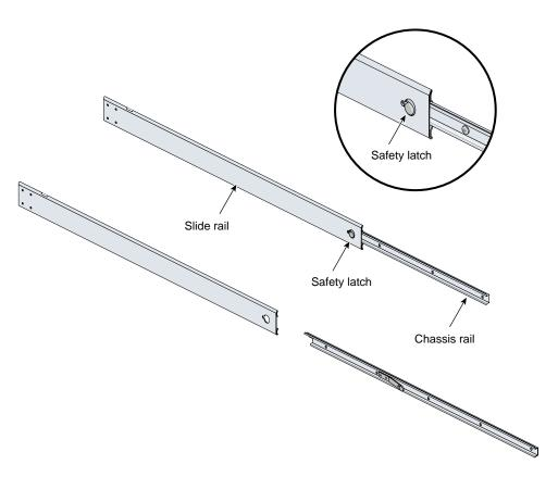
Figure C-1 Removing the Chassis Rail from the Slide Rail
