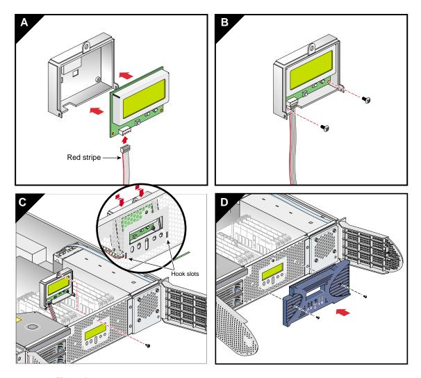
Figure A-13 Installing an L1 Controller Display Panel
