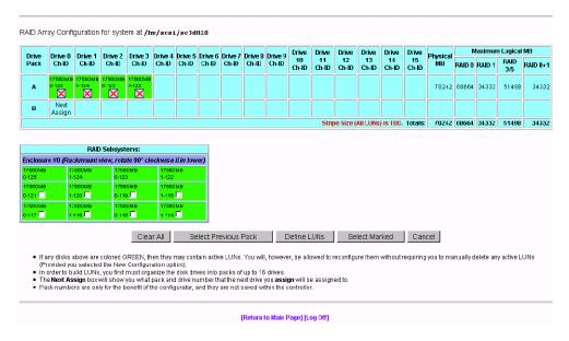
Figure 3-6 Drives Assigned Into Pack A (12 drive, 1Gb TP9100 RAID Subsystem view)
