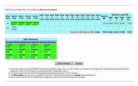
Figure 3-15 Add LUN(s) Screen (12 drive, 1Gb TP9100 RAID Subsystem view)
