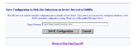
Figure 3-60 Save Current Controller Configuration
