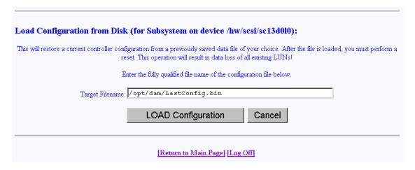
Figure 3-61 Load Controller Configuration
