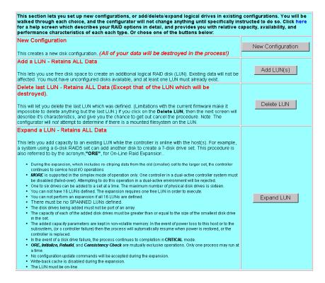
Figure 3-19 Create/Destroy/Expand Logical Drives Screen
