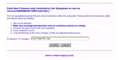
Figure 3-62 Flashing New Firmware
