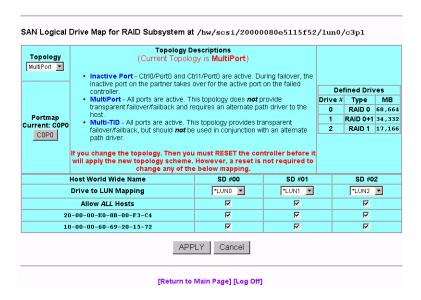
Figure 3-28 SAN Mapping Topology view - 1Gb TP9100 RAID controller
