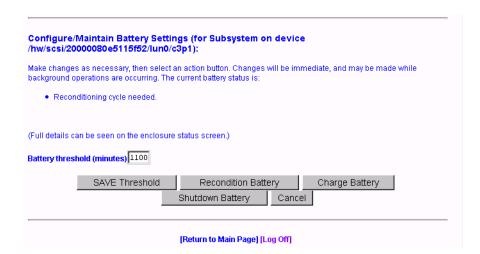
Figure 3-66 Adjust Battery Settings
