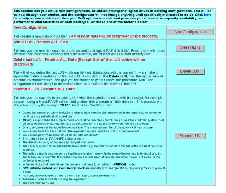
Figure 3-14 Create/Destroy/Expand Logical Drives Screen
