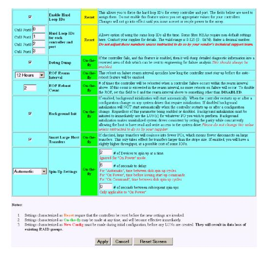
Figure 3-33 View/Modify Controller Configuration, 2Gb TP9100, 8.40 firmware (partial)
