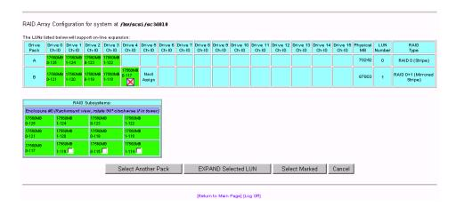
Figure 3-20 Expand LUN Screen (12 drive, 1Gb TP9100 RAID Subsystem view)
