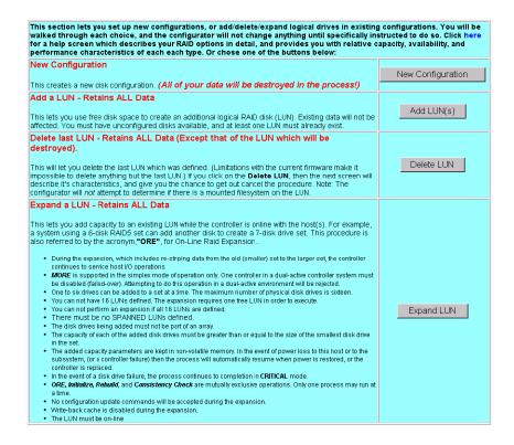
**Figure 3-4** Create/Destroy/Expand Logical Drives Dialog Box
