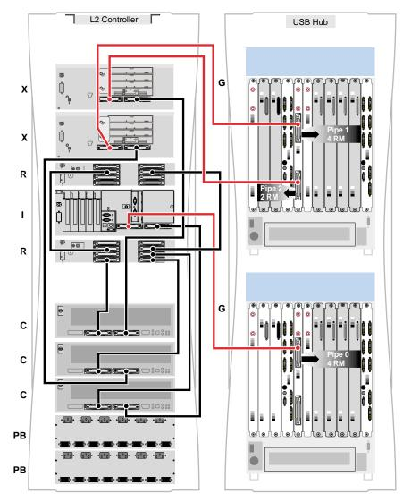
Figure 3-3 Configuration Example: Two-Racks, Two G-bricks with Three InfiniteReality Pipes
