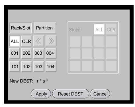
1. Select the **DEST** button to select the bricks or partition you want to power on. The destination selection window, shown in Figure 4-7, appears.
