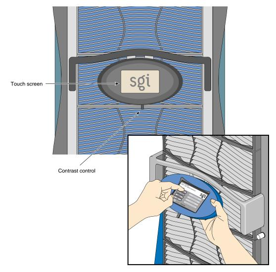
Figure 4-15L2 Controller Interface Screen
