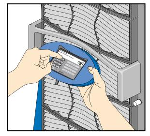
Figure 4-5 L2 Controller Touch Display
