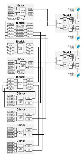
**Figure 1-6** InfiniteReality Dual-rack System with Two G-bricks, Four C-bricks, and One N-brick
