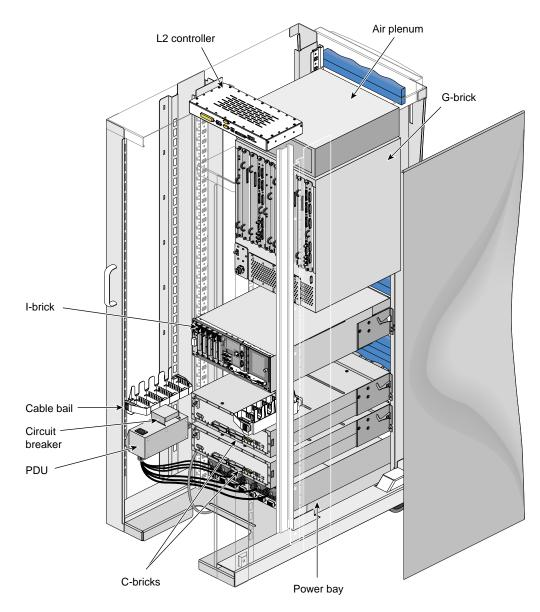
Figure 1-2 Example of SGI Onyx 3000 Graphics System (Rear View)
