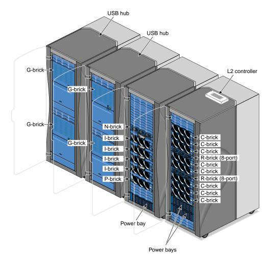
Figure 1-12SGI Onyx 3800 Graphics System with Four G-bricks (with Seven InfiniteReality<br/>Pipes in Total)
