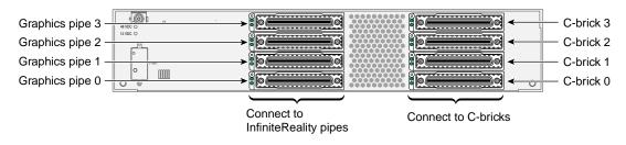
Figure 2-18 N-brick Rear View
