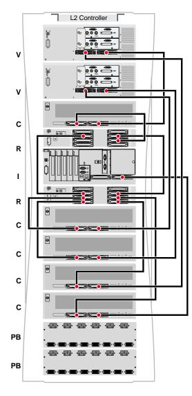
Figure 3-6 Configuration Example: One Rack with Two V-bricks (with Two Pipes Each)
