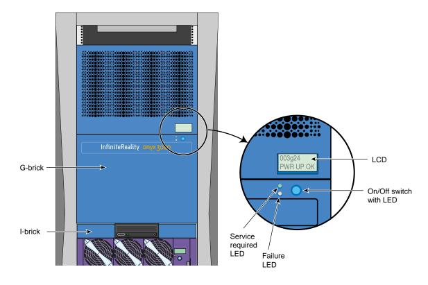
Figure 6-1 G-brick L1 System Controller Display and Controls
