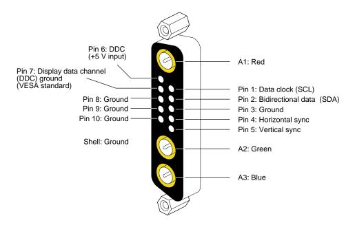
Figure 2-7 DG5 13W3 Connector Pinout
