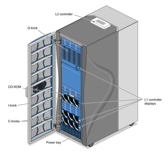
Figure 1-8SGI Onyx 3200 Graphics System with One G-brick with One InfiniteReality<br/>Graphics Pipe
