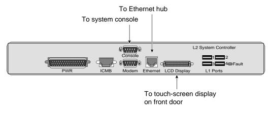
Figure 6-4 L2 Controller Connectors
