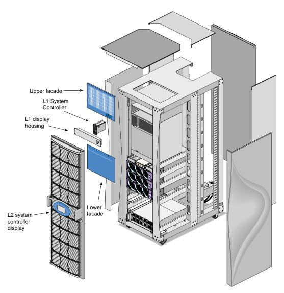
Figure 5-1 shows a rack with CRUs for an SGI Onyx 3000 series graphics system that contains a G-brick. Note that the facade on the G-brick is also removable.
