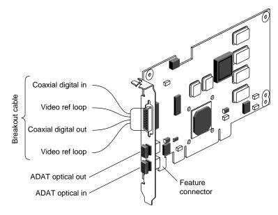
Figure 3-11 PCI Audio Board
