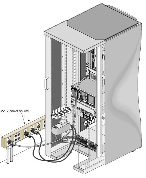
Figure 4-3 shows the connection between a PDU power cable and an external power receptacle.
