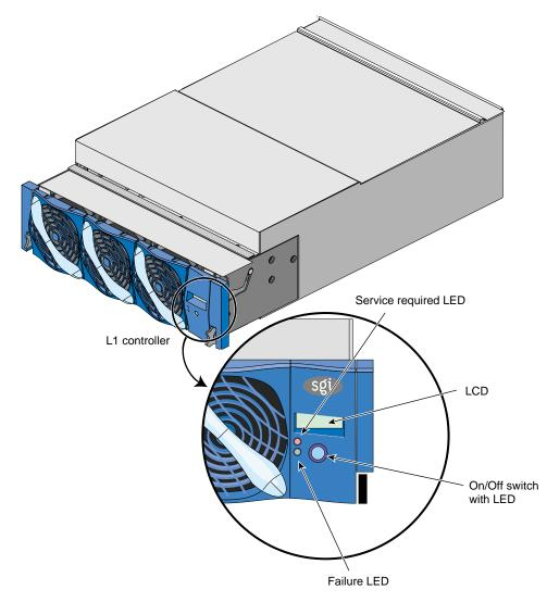
Figure 2-13 V-brick Front View
