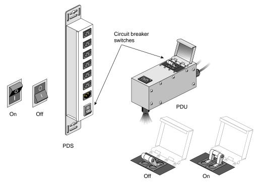
Figure 4-4 PDU or PDS Circuit Breaker Switches
