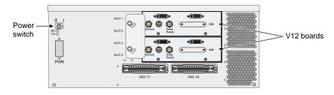
Figure 2-15 V-brick with Two V12 Boards
