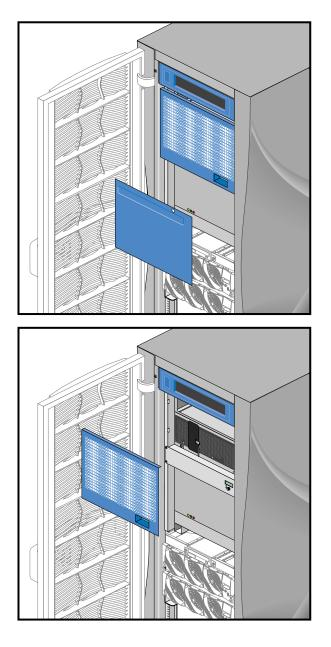
Figure 5-2Removing the G-brick Facade
