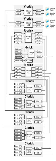
Figure 1-7 Example of Two V-brick, Single-rack Graphics Block Diagram
