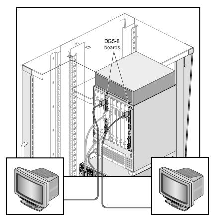
Figure 3-8 Connecting Two Monitors to Separate DG5 Boards in G-brick
