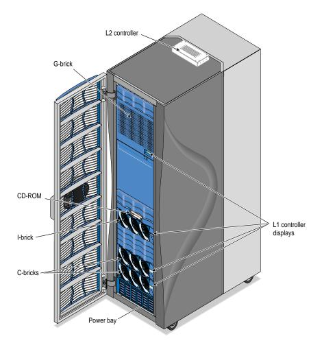
Figure 1-1Example of SGI Onyx 3000 Graphics System (Front View)
