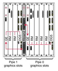
Figure 3-1 G-brick Graphics Boards and Connector Locations
