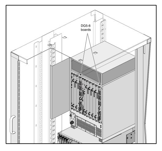
Figure 2-6 DG5-8 Board Locations in the G-brick
