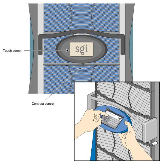
Figure 6-2L2 Controller Touch Display and Controls
