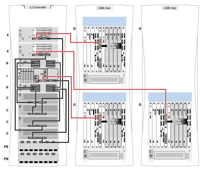
Figure 3-4 shows a configuration example of a graphics system in three racks with three InfiniteReality graphics pipes (with 4 RMs each) in three G-bricks.
