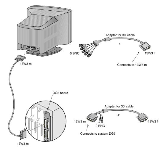
Figure 3-7 13W3 Monitor Cable and Adapters
