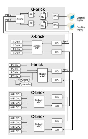
Figure 1-5 shows a configuration with a single G-brick (with two InfiniteReality pipes with two RMs each), two C-bricks, an X-brick, and an I-brick.
