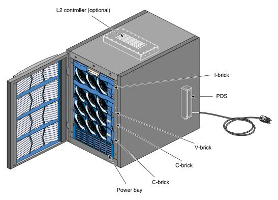
Figure 1-9SGI Onyx 3200 Graphics System with One V-brick and Support for One<br/>InfinitePerformance Graphics Pipe
