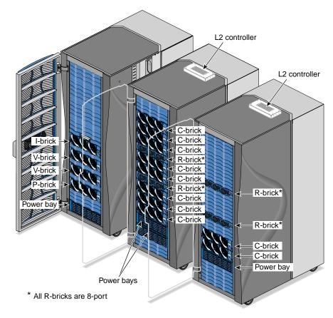
Figure 1-13SGI Onyx 3800 Graphics System with Two V-bricks (with Two InfinitePerformance<br/>Pipe Each)
