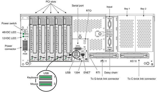
Figure 3-10 Primary I-brick Keyboard/Mouse Connectors
