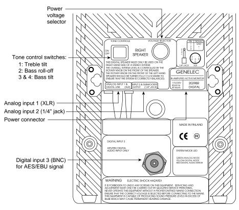
Figure 3-15 Right Speaker Rear Controls and Connectors
