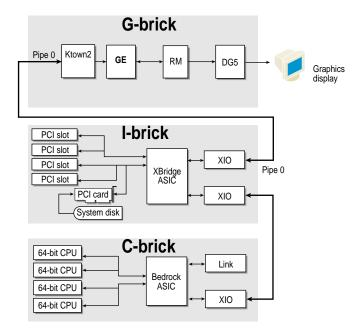
Figure 1-4 InfiniteReality Single-rack System with One Single-pipe G-brick and One C-brick
