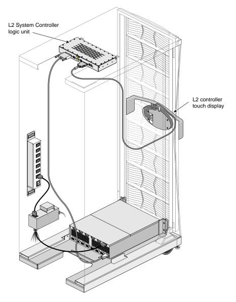
Figure 6-3 Location of L2 Controller in Rack
