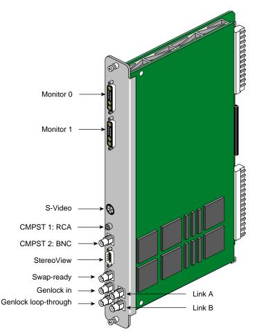
Figure 2-10 DG5-2 with Optional GVO Connectors
