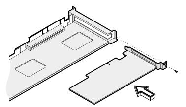
Figure 2-9 Inserting the Expansion Card into the Riser Card
