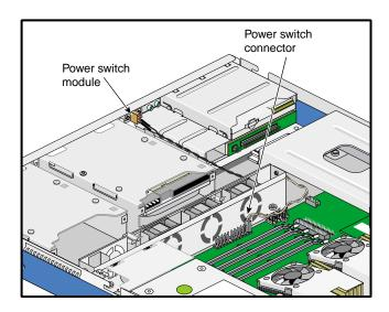
Figure 2-17 Location of the Power Switch Cable Connector
