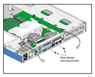
Figure 2-14 Rear System Blower Securing Screws
