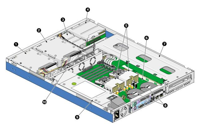
Figure 1-4 SGI 1100 Server Internal Components
