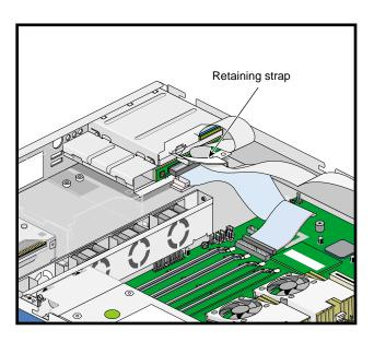
**Figure 2-26** Releasing the Signal Cable Retaining Strap
