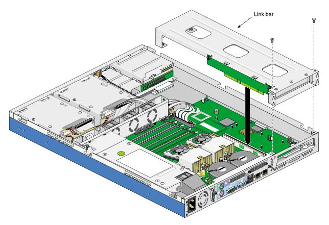
Figure 2-5 Installing the Link Bar
