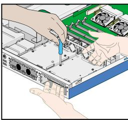
Figure 2-39 Installing the Hard Disk Drive
