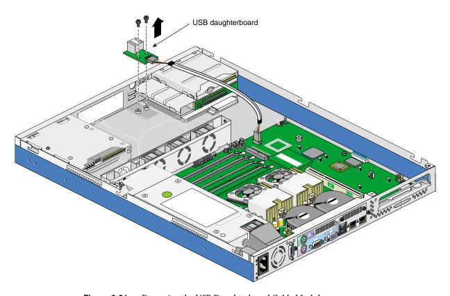
Figure 2-21 Removing the USB Daughterboard Cable Module
