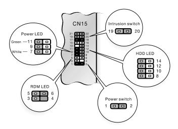
Figure A-2 illustrates the LED/switchboard CN15 connector settings.
