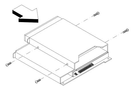
Figure 2-31 Installing the Diskette Drive into the Drive Module
