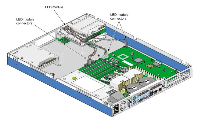
Figure 2-15 Location of the LED Cable Connectors
