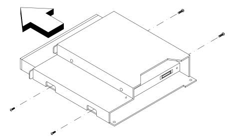
**Figure 2-33** Removing the CD-ROM Drive from the Drive Module
