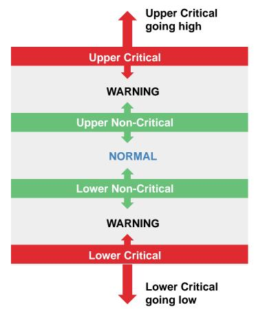
Figure 3-1 Threshold Setting Levels
