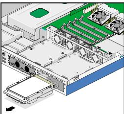
Figure 2-38 Removing the Hard Disk Drive
