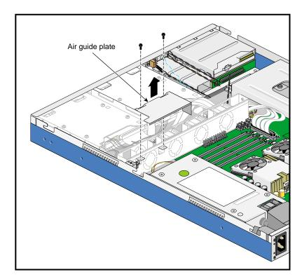
Figure 2-42 Removing the Air Guide Plate
