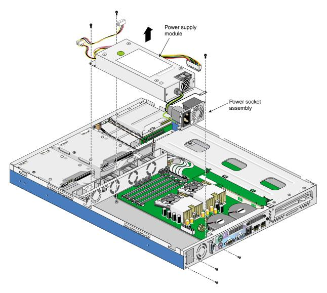
**Figure 2-44** Removing the Power Supply Module
