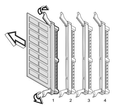
Figure 2-52 Removing a DIMM
