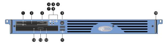
Figure 1-2 Front Controls and Indicators
