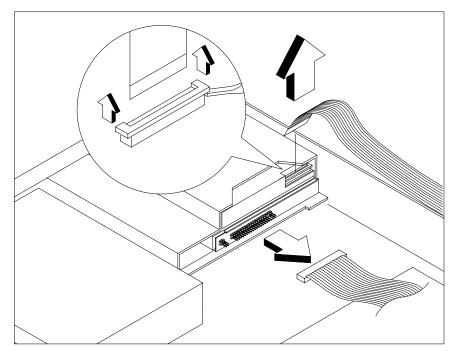
**Figure 2-27** Disconnecting the Drive Module Signal Cables
