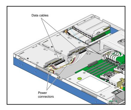
Figure 2-36 Removing Hard Drive Cables
