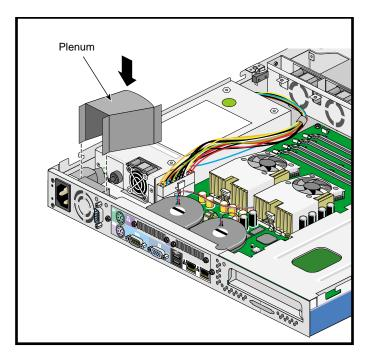
Figure 2-46 Installing the Plastic Plenum
