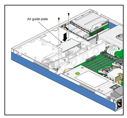
Figure 2-47 Installing the Metal Air Guide Plate
