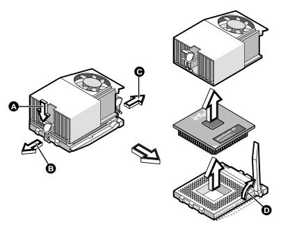
Figure 2-48 Removing a Processor
