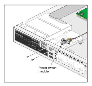
**Figure 2-18** Removing the Power Switch Cable Module
