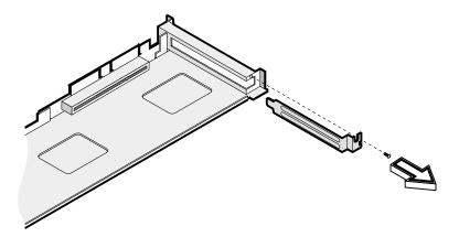
**Figure 2-8** Removing the Expansion Slot Filler Plate
