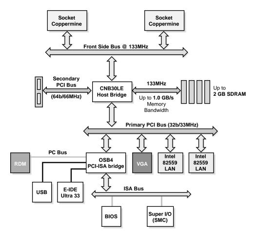
Figure 1-1 System Block Diagram
