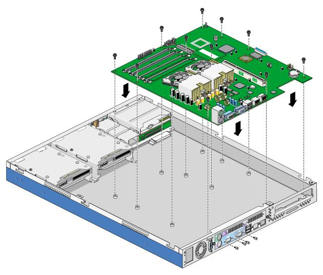
Figure 2-56 Installing the System Board
