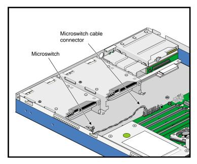
Figure 2-23 Location of the Intrusion Alert Microswitch Cable Connector
