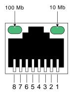
**Figure C-6** Ethernet Port Pinout
