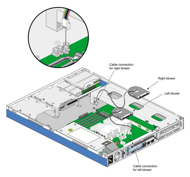
**Figure 2-13** Location of the Rear System Blower Cable Connectors
