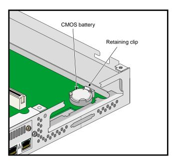
**Figure 2-54** Replacing the CMOS Battery
