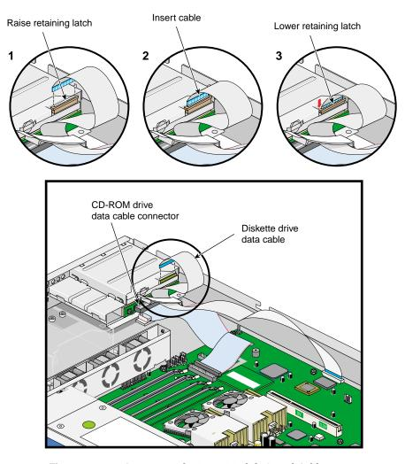
**Figure 2-29** Connecting the Drive Module Signal Cables
