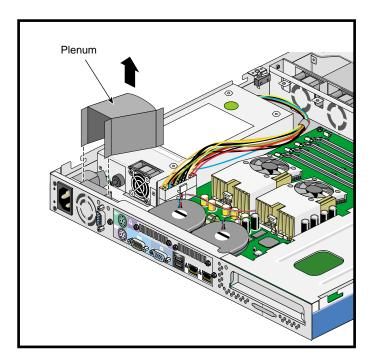
Figure 2-43 Removing the Plastic Plenum
