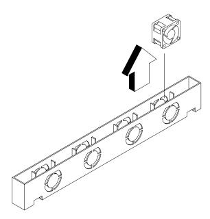
Figure 2-12 Removing the Chassis Fan
