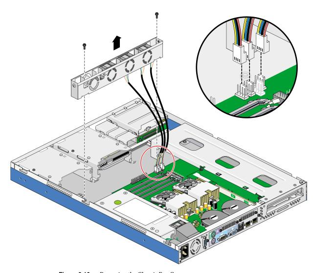
Figure 2-10 Removing the Chassis Fan Cage
