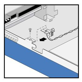
Figure 2-25 Installing the Intrusion Alert Microswitch Cable Module
