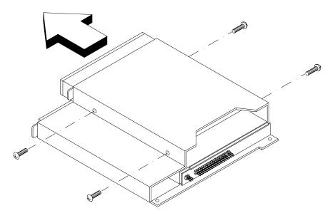
**Figure 2-30** Removing the Diskette Drive from the Drive Module
