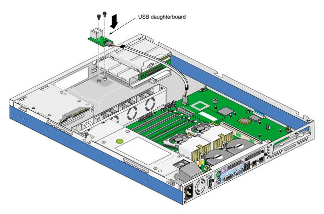
Figure 2-22 Installing the USB Daughterboard Cable Module
