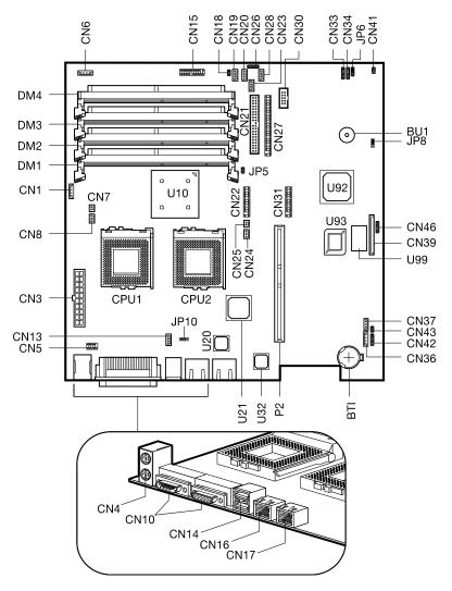
Figure A-1 System Board Layout
