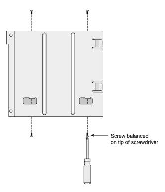
**Figure 2-35** Securing the CD-ROM drive to the Drive Module
