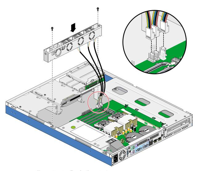
**Figure 2-11** Installing the Chassis Fan Cage
