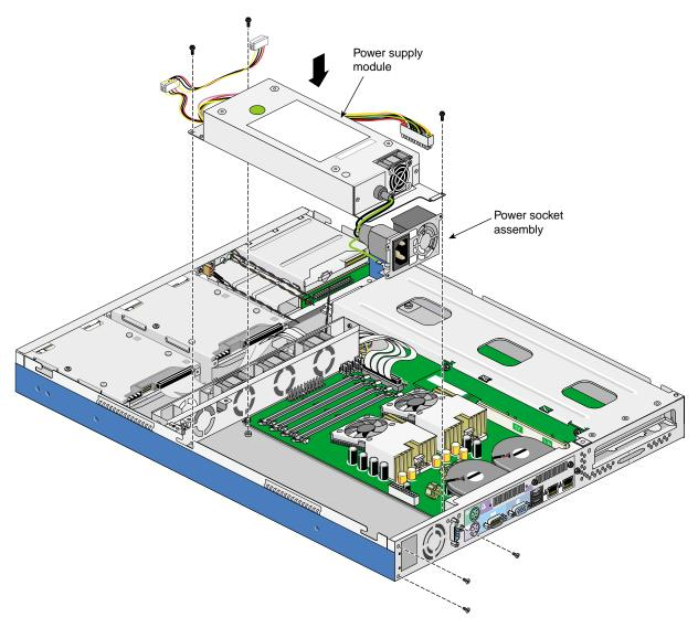
**Figure 2-45** Installing the Power Supply Module
