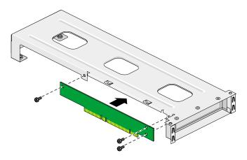
Figure 2-7 Installing the Riser Card on the Link Bar
