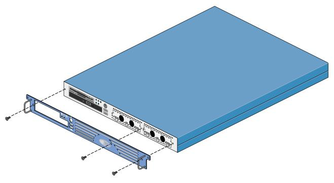
Figure 2-3 Removing the Front Panel
