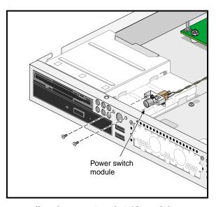
Figure 2-19 Installing the Power Switch Cable Module
