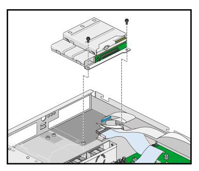
Figure 2-28 Removing the Drive Module
