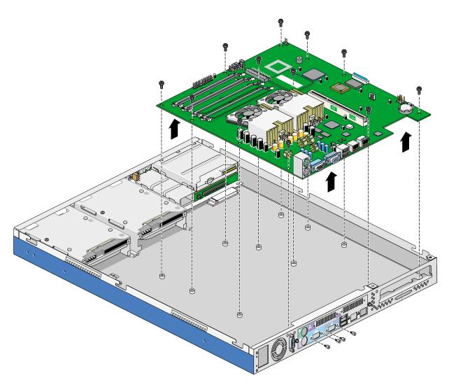
**Figure 2-55** Removing the System Board
