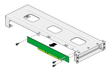
Figure 2-6 Detaching the Riser Card from the Link Bar
