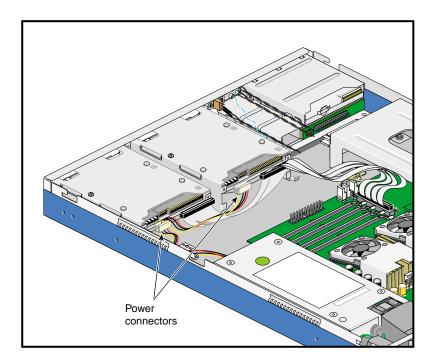
**Figure 2-41** Location of the Hard Drive Power Supply Connectors
