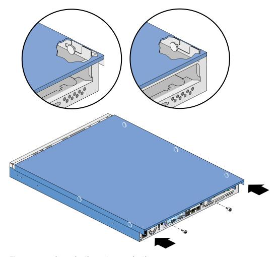
**Figure 2-2** Placing the Chassis Cover on the Chassis
