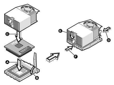
Figure 2-49 Installing the Processor
