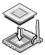
Figure 2-51 Installing a Processor Terminator Board
