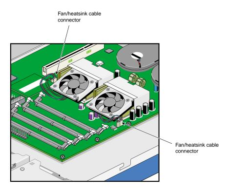
Figure 2-50 Location of the Fan/Heatsink Cable Connector
