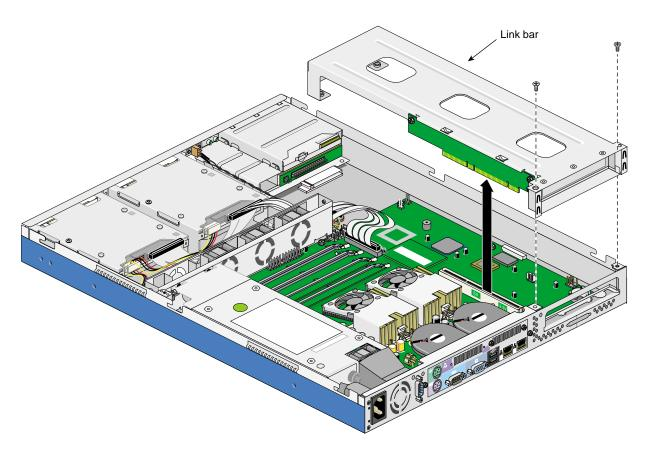
Figure 2-4 Removing the Link Bar
