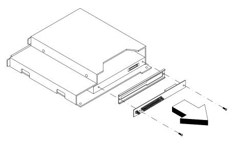
**Figure 2-32** Removing the CD-ROM Drive Converter Board
