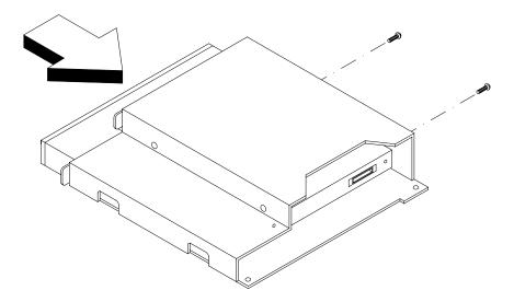
Figure 2-34 Installing the CD-ROM Drive into the Drive Module
