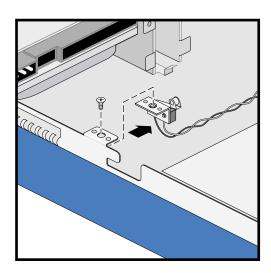
Figure 2-24 Removing the Intrusion Alert Microswitch Cable Module
