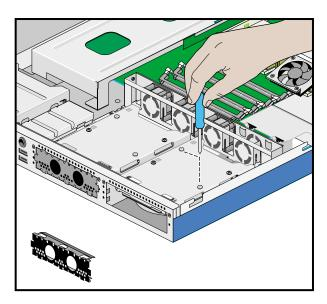
Figure 2-37 Removing Two of Four Hard Disk Drive Screws
