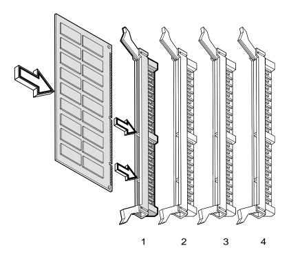
Figure 2-53 Installing a DIMM
