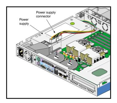
Figure 2-40 Location of the System Board Power Supply Connector
