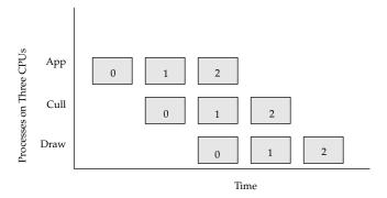
**Figure 4-4** Multiprocessing Frames in the Pipe
