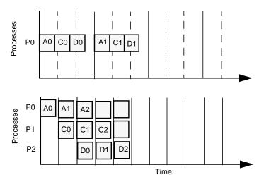
Figure 11-2 Multiprocessing in the Graphics Pipeline
