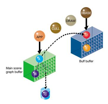
Figure 12-3 Linking and Deleting Nodes
