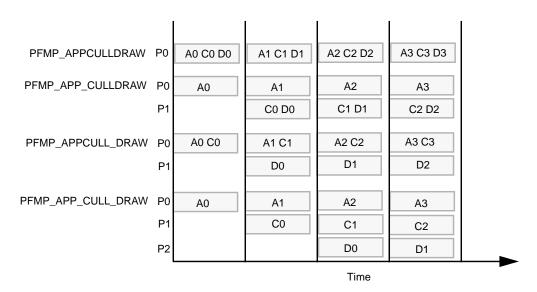
**Figure 11-5** Four Common Multiprocessing Models
