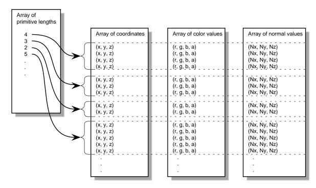
Figure 7-2 Arrays of Stripped Primitives
