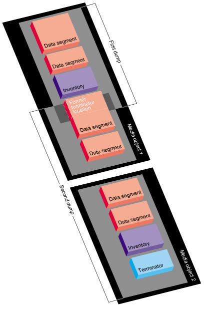
Figure 2-4 Multiple Dumps on Multiple Media Objects
