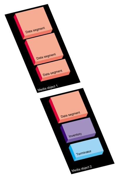
Figure 2-2 illustrates the data layout of a single dump session that requires two media objects on each of two devices.
