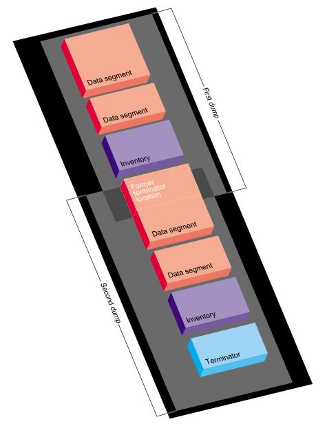
Figure 2-3 Multiple Dumps on Single Media Object
