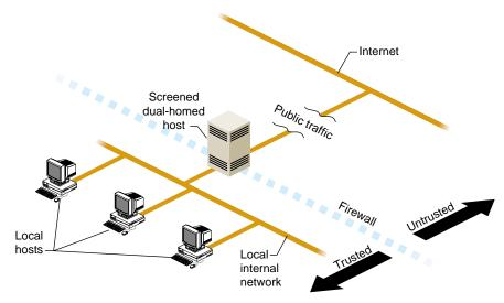
Figure 5-1 A Simple Firewall Environment
