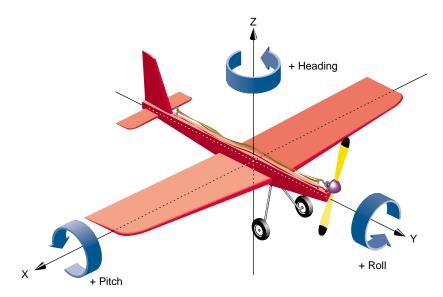
Figure 2-5 Heading, Pitch, and Roll Angles
