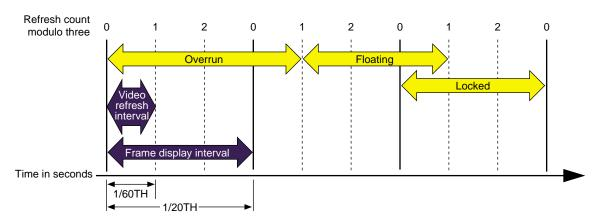
Figure 5-1 Frame Rate and Phase Control
