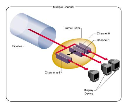
Figure 2-6 Single-Channel and Multiple-Channel Display
