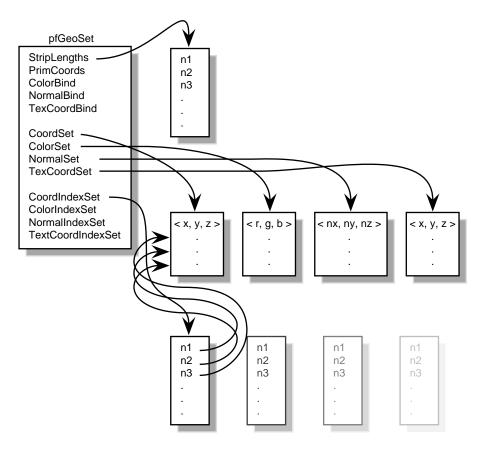
Figure 8-3 Indexing Arrays
