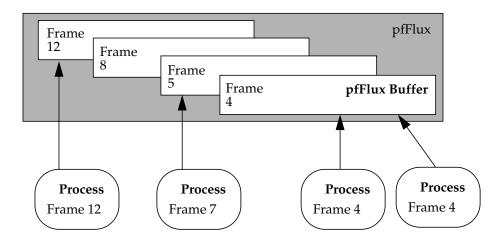
Figure 16-1 How pfFlux and Processes Use Frame Numbers
