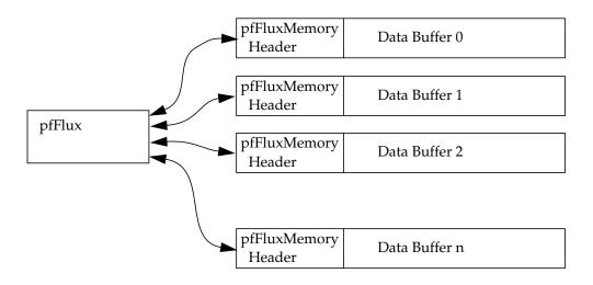
**Figure 16-2** pfFlux Buffer Structure
