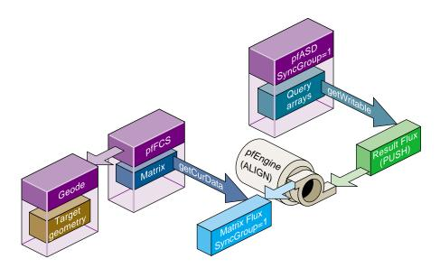
Figure 17-16 Example Setup for Geometry Alignment
