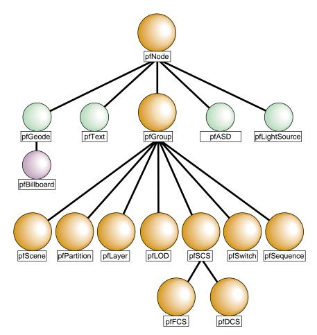
Figure 3-1 Nodes in the OpenGL Performer Hierarchy
