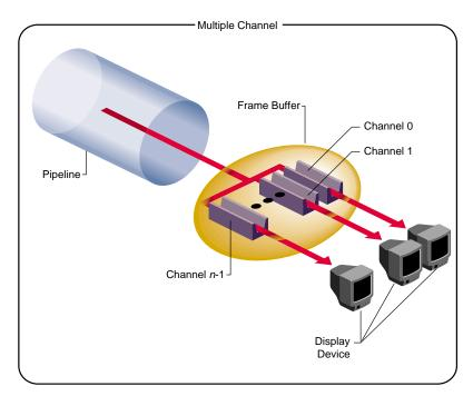
Figure 2-6 Single-Channel and Multiple-Channel Display
