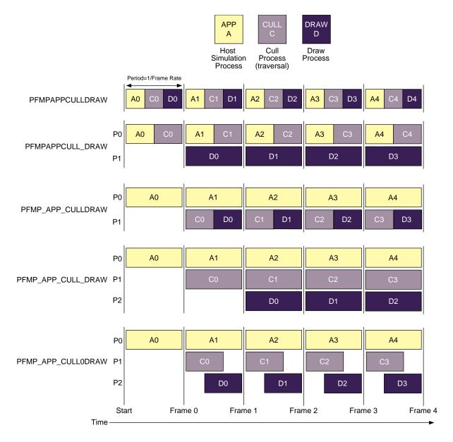
Figure 5-6 Multiprocessing Models
