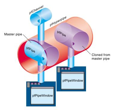
are attached to the master pfPipe. OpenGL Performer automatically clones all objects, except pfChannels, across all of the pfPipes in the pfHyperpipe, as shown in Figure 11-4.
