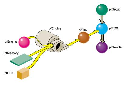
Figure 16-4 pfEngine Driving a pfFlux That Animates a pfFCS Node
