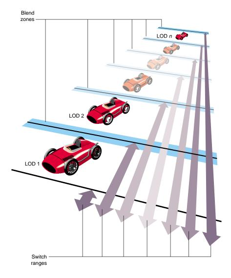
Figure 5-3 Level-of-Detail Processing
