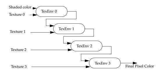
**Figure 9-2** Generating the Color of a Multi-textured Pixel
