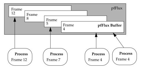
Figure 16-1 How pfFlux and Processes Use Frame Numbers
