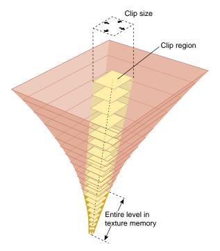
Figure 12-1 Cliptexture Components
