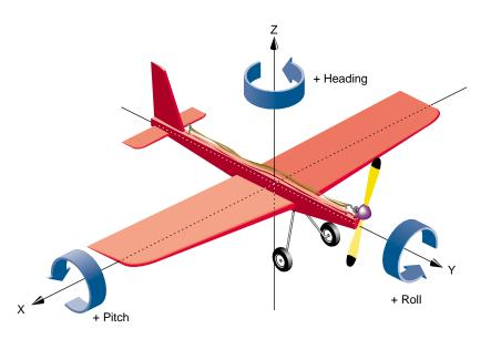
Figure 2-5 Heading, Pitch, and Roll Angles
