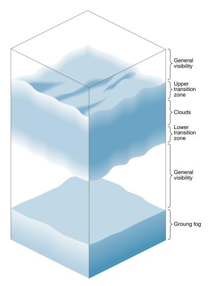
Figure 6-1 Layered Atmosphere Model
