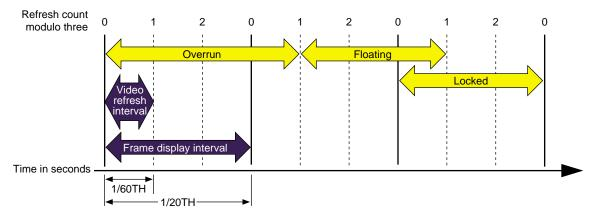
Figure 5-1 Frame Rate and Phase Control
