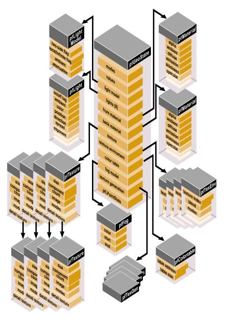
Figure 9-1 pfGeoState Structure
