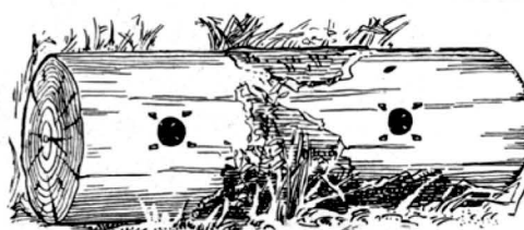
MINK, MARTEN or WEASEL TRAP. 2 inch hole. 4 horse shoe nails. Use bait.
