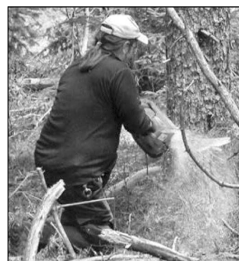
Making the final felling cut after the felling wedge has been removed from the opposite side.
