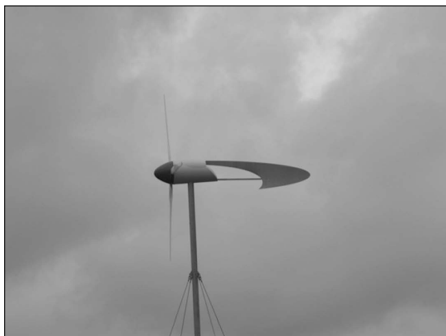
A wind turbine. The propeller is turned to face the wind. As it spins, it turns the generator of the turbine to create electricity.
