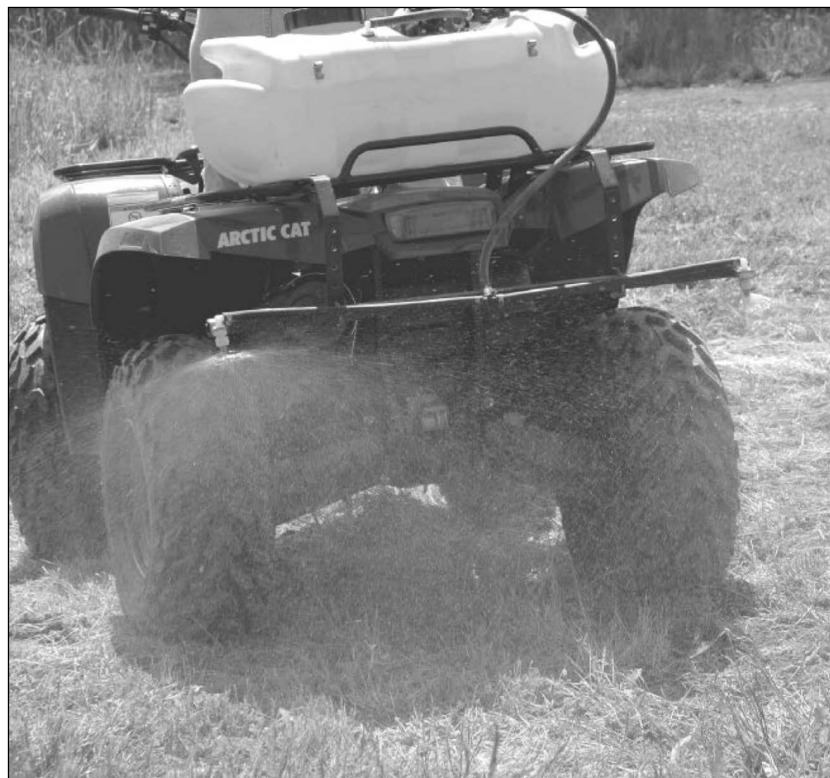
An ATV-mounted sprayer unit works well to apply herbicide on food plots 5 acres and less.
