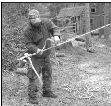
Tying off the winch that will pre-load tall tree's direction of fall to ensure that it impacts precisely where it was meant to go
