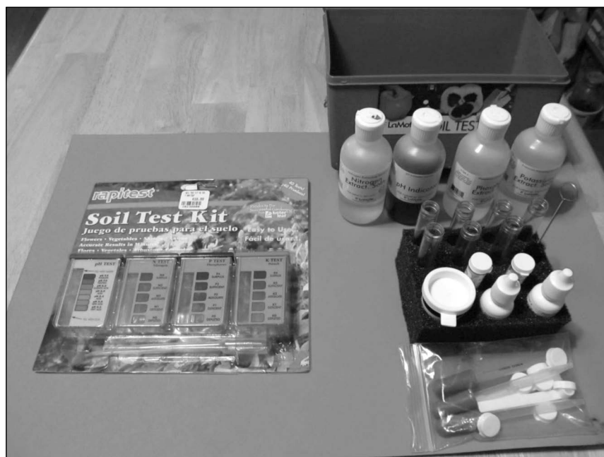
Both the Rapitest and LaMotte testing kits will provide pH, nitrogen, phosphorus, and potassium levels as well as recommendations.
