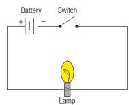
Figure 0.6 The switch is off (open) and the lamp is off, indicating a "0."
