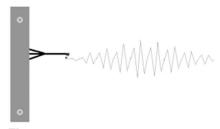
Figure 0.26 The resulting signal is not as smooth as the original (lower resolution).
