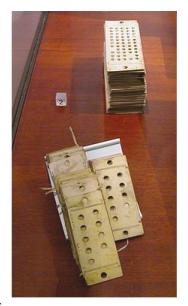
Figure 0.1 Punched cards for the analytical engine.
