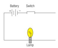
Figure 0.5 The switch is closed and the current is flowing, turning the lamp on. This is a "1."
