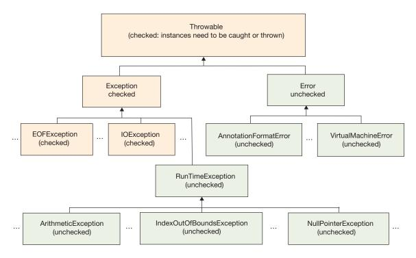
Figure 10.1 A subset of the exception classes included in the Java API and their inheritance chains.
