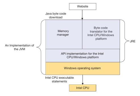
Figure 1.26 System-specific components of the Java Virtual Machine.
