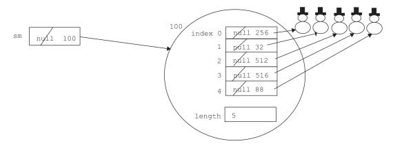
**Figure 6.7**An array of five reference variables pointing to five **Snowman** objects.
