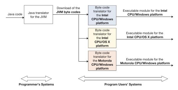
Figure 1.25 The Java multiple-platform translation process.
