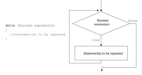
Figure 5.13 The syntax and execution path of the **while** statement.
