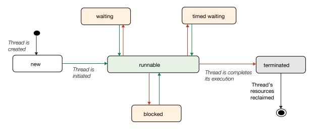
Figure 14.6 Transitions among the six states of a thread during its life.
