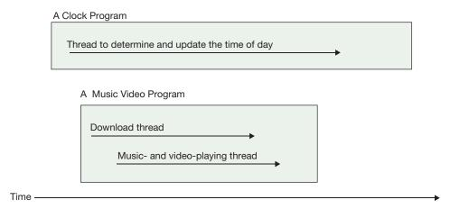
Figure 14.1 A single-thread and a double-thread process.
