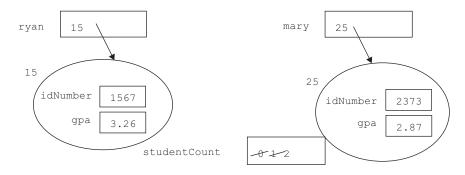
Figure 7.3 The changes to the static data member **studentCount** after two objects are created.
