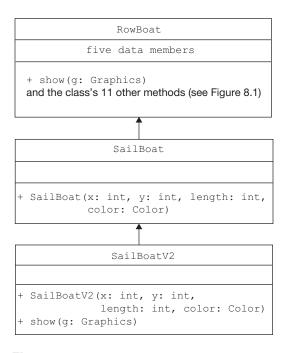
Figure 8.9 The inheritance chain of the class **SailBoatV2**.
