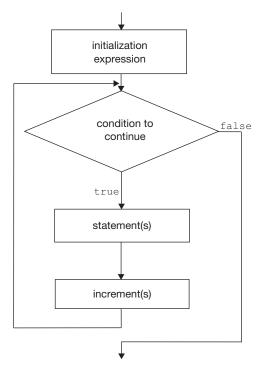
Figure 5.3 The generalized syntax of the **for** statement and its execution path.
