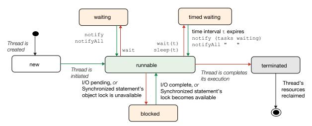
Figure 14.8 Actions and events that transition a thread from the runnable state and back again.
