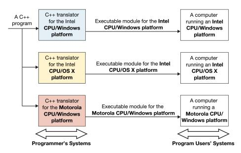
Figure 1.24 The C++ multiple-platform translation process.
