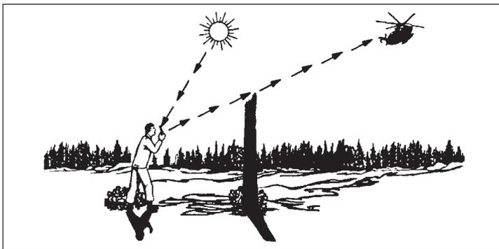
**Figure 19-5** Aiming an improvised signal mirror—stationary object.
