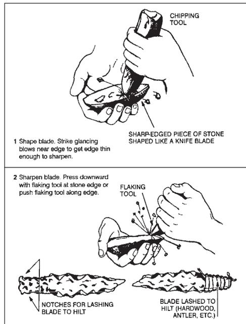
Figure 12-3 Making a stone knife.
