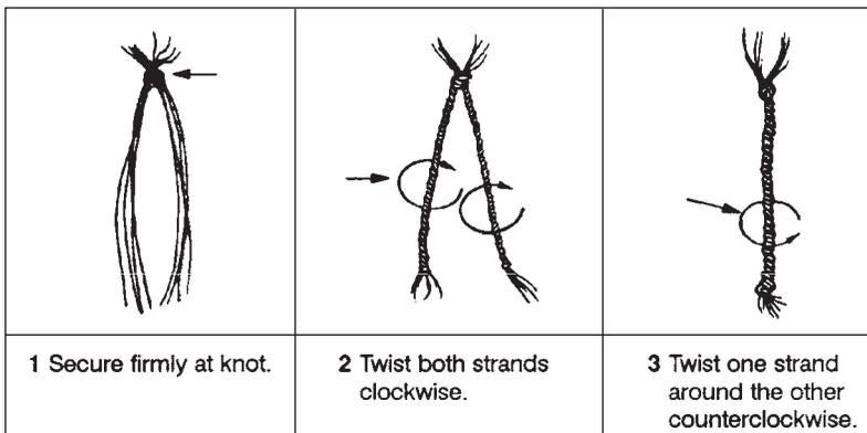
Figure 12-8 Making lines from plant fibers.
