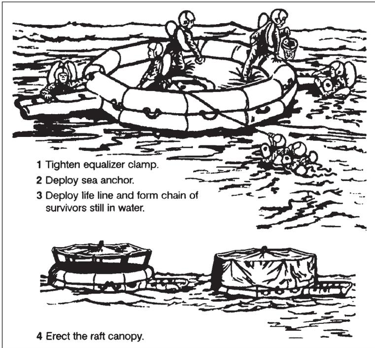
**Figure 16-18** Immediate action—multiplace raft.
