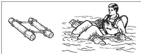
**Figure 17-8** Log flotation.
