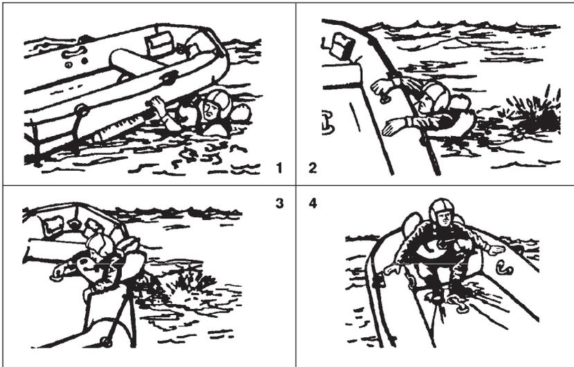
Figure 16-14 Method of boarding seven-man raft.
