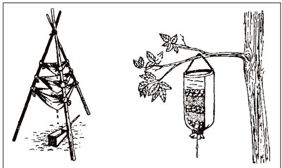
**Figure 6-9** Water filtering systems.
