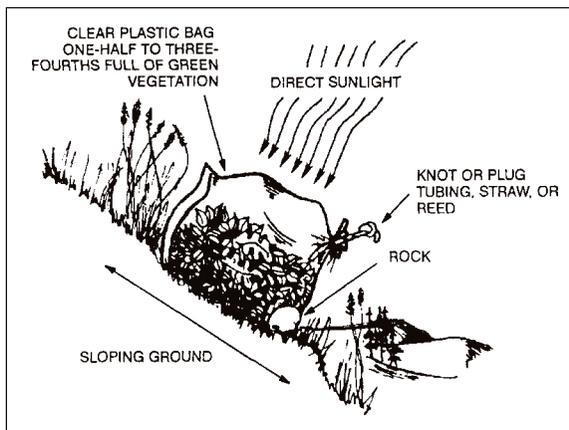
Figure 6-6 Aboveground solar water still.
