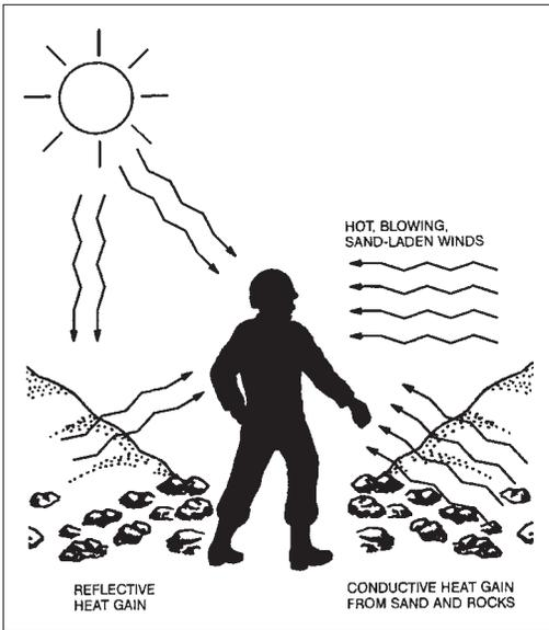
**Figure 13-1** Types of heat gain.
