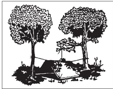
**Figure 5-2** Poncho tent using overhanging branch.
