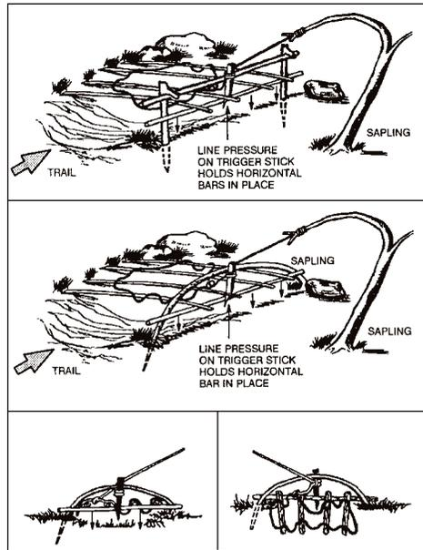
Figure 8-11 Treadle spring snare.
