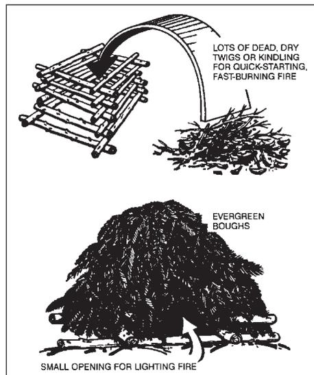
**Figure 19-2** Smoke generator—ground.
