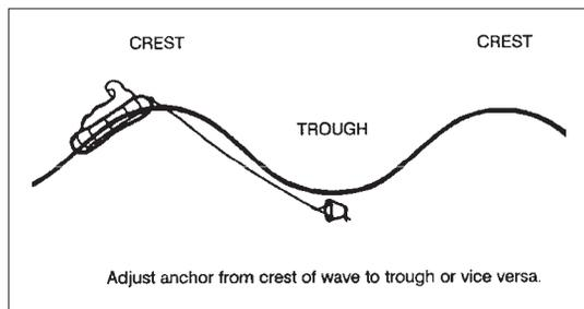
**Figure 16-6** Deployment of the sea anchor.
