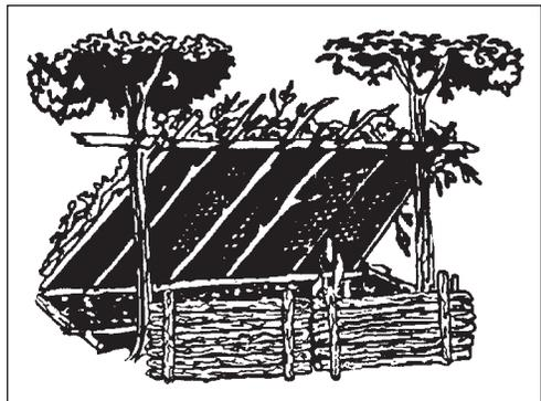
Figure 5-5 Field-expedient lean-to and fire reflector.
