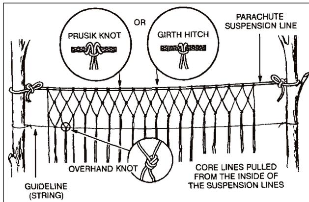
Figure 8-19 Making a gill net.
