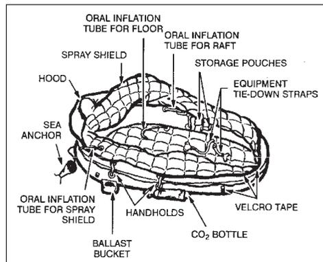
**Figure 16-8** One-man raft with spray shield.
