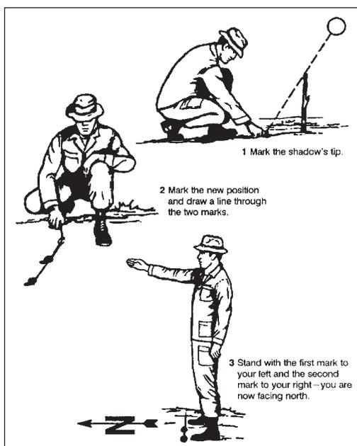
Figure 18-1 Shadow-tip method.
