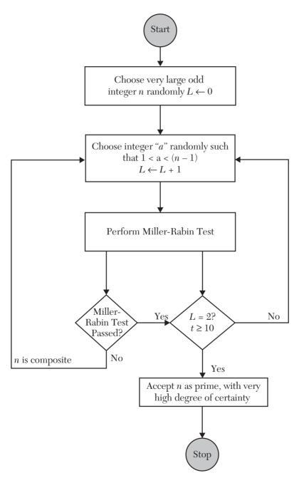
**FIGURE** 4.1 Flow chart for the procedure to determine a Prime Number with very high degree of certainty (using Miller-Rabin Algorithm repeatedly).
