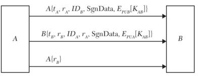
FIGURE 10.6 A schematic diagram of a Three-Way Authentication Procedure.
