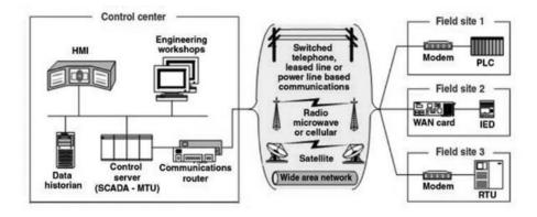
FIGURE 14.10 SCADA concept topology
