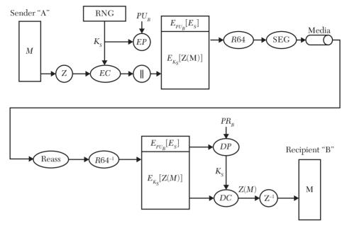
FIGURE 11.2 A schematic diagram depicting "Confidentiality Only" service.
