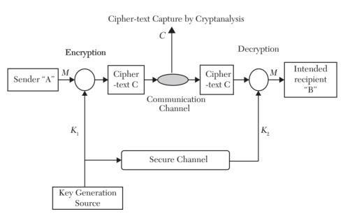
FIGURE 3.2 Conventional encryption model.
