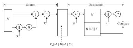
**FIGURE 8.10** A schematic diagram of Symmetric Encryption of a Signed Message (using a Secret Value to make the Hash Value secure).
