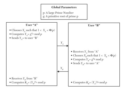
FIGURE 7.1 A schematic diagram of the Diffie-Hellman Algorithm.
