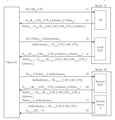
FIGURE 9.3 A schematic diagram of the Inner-Kerber Authentication Sequence.
