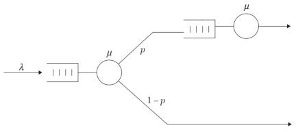
FIGURE 2.33 A queueing system with Splitting.
