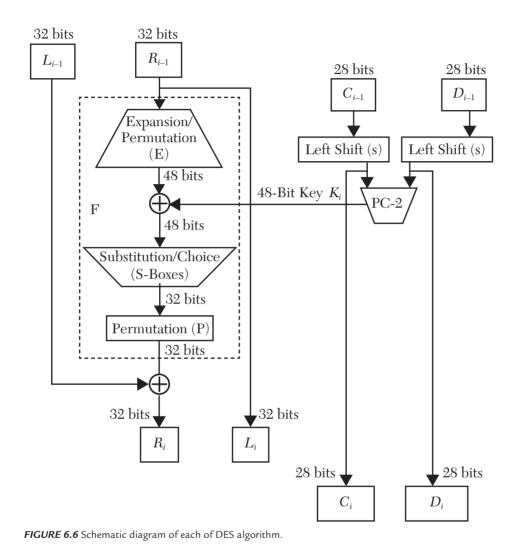
**1. Expansion Permutation (E):** This performs permutation on the 32-bit input and also expands it to a 48-bit output as follows:
