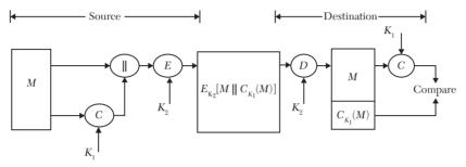
**FIGURE 8.6** A schematic diagram of the Message Authentication and Confidentiality (MAC linked to plaintext).
