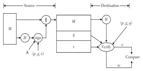
FIGURE 8.18 A schematic diagram of ElGamal's Digital Signature Scheme.
