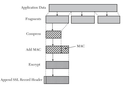
FIGURE 12.13 Overall operation of SSL Record Protocol.
