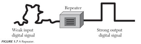
Repeaters operate at the Physical layer (Layer 1) of the OSI model. They cannot connect different network architectures. Also, they can't reformat, resize, or manipulate the data signal. A repeater is used to re-time, re-shape, and re-amplify the data signal to its original shape. A repeater receives data on one port and repeats them on the other port. It can be used as a connection device on a network. Figure 1.8 shows a repeater on a network.
