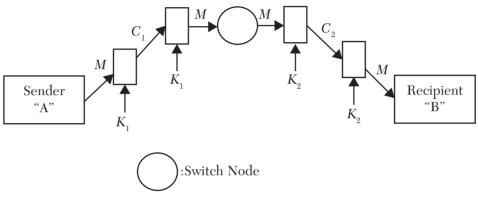
FIGURE 3.4 Schematic diagram showing link encryption.
