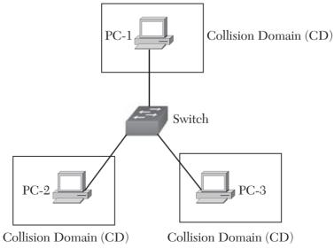
FIGURE 1.12 The switch divides the collision domain.
