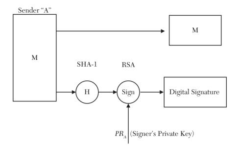
FIGURE 10.16 A schematic diagram showing integrity of data.
