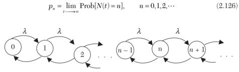
FIGURE 2.21 State diagram for M/M/1 queue.
