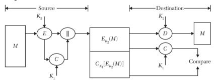
**FIGURE 8.7** A schematic diagram of the Message Authentication and Confidentiality (MAC linked to cipher-text).
