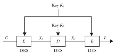
**FIGURE 6.14** Three blocks of DES with two 56-bit keys  $K_1$  and  $K_2$  are used for decryption.
