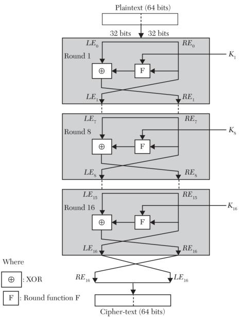
FIGURE 6.4 Feistel encryption algorithm (for DES).
