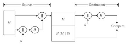
FIGURE 8.8 A schematic diagram of the Hash Function.
