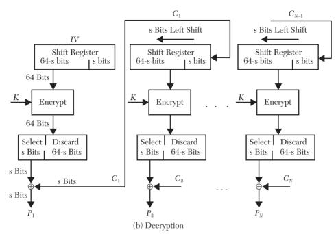
FIGURE 6.19 s-Bit Cipher Feedback (CFB) Mode encryption/decryption.
