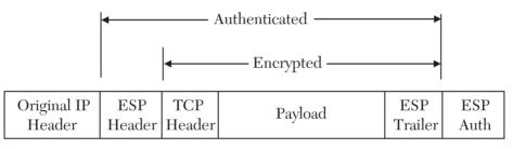
(Transport Mode IP-V4 Packet with ESP)
