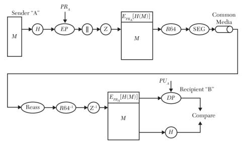
FIGURE 11.1 A schematic diagram depicting "Authentication Only" service.
