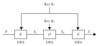
**FIGURE 6.13** Three blocks of DES with two 56-bit keys  $K_1$  and  $K_2$  are used for encryption.
