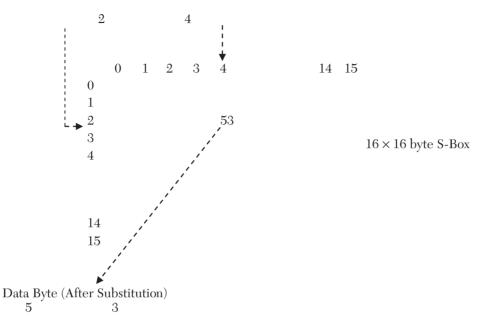
FIGURE 6.25 The AES defines a 16 × 16 byte S-Box.
