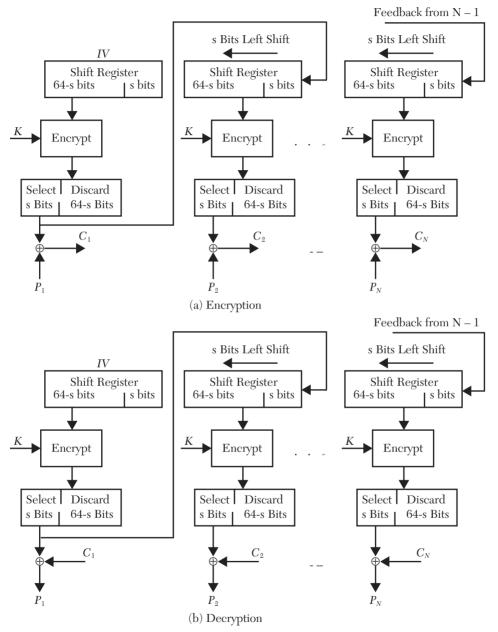
FIGURE 6.20 s-Bit Output Feedback (OFB) Mode encryption/decryption.
