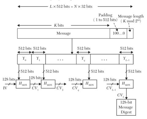
FIGURE 8.12 A schematic diagram of the overall processing of an MD5 algorithm.
