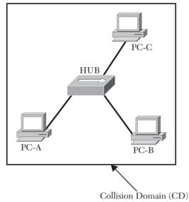
FIGURE 1.11 A Hub does not divide the collision domain.
