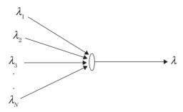
FIGURE 2.15 Superposition of Poisson streams.
