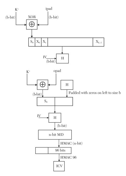
FIGURE 12.3 A schematic diagram of an ICV-generating algorithm.
