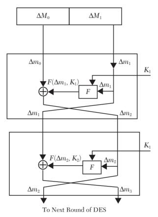
FIGURE 6.10 A Schematic of transformation of the XOR differences at the outputs of various rounds of DES.
