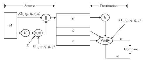
FIGURE 8.19 A schematic diagram depicting DSA.
