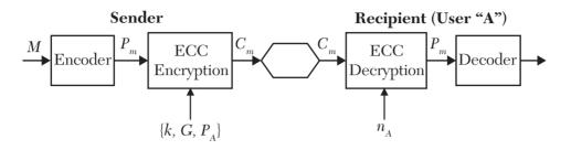
Figure 7.5 illustrates the ECC-based Encryption/Decryption Chain.
