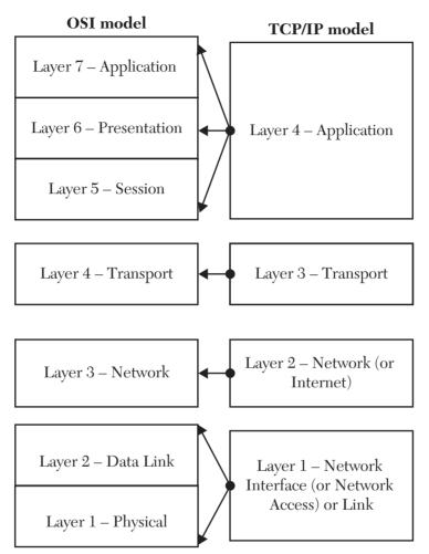
FIGURE 1.4 The TCP/IP model Mapped to the OSI model.
