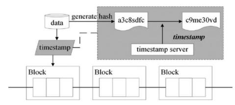
FIGURE 14.16. Tamper-proofing mechanism of blockchain
