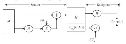
FIGURE 8.3 A schematic diagram of digital signatures using Public-Key Cryptography.
