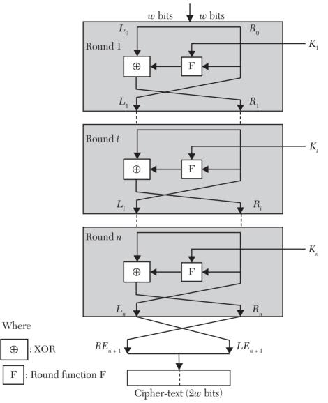
FIGURE 6.2 Feistel Cipher Structure (Encryption).
