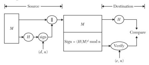
FIGURE 8.17 A schematic diagram of the Signature verification.
