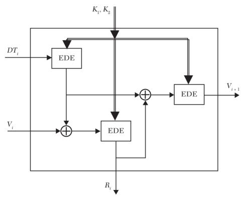
FIGURE 6.29 Schematic diagram of the Random Number Generator.
