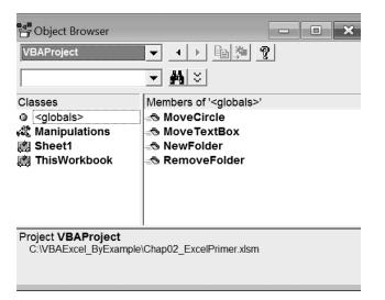
*FIGURE 2.14.* The Object Browser lists all the procedures available in a particular VBA project.
