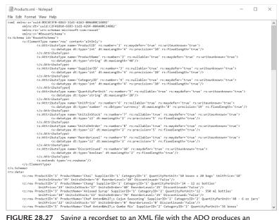
FIGURE 28.27 Saving a recordset to an XML file with the ADO produces an attribute-based XML file.
