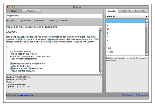
Figure 4-1. Using alternation in RegExr desktop version
