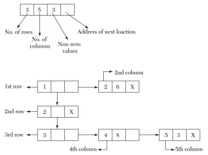
Figure 3.12. Linked representation of a sparse matrix.
