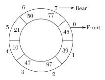
Figure 5.13. Initial circular queue without deletion.
