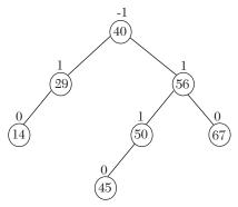
Figure 8.22. AVL tree before insertion.
