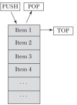
Figure 7.2. Representation of a stack.
