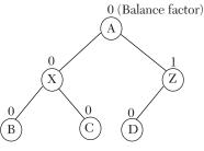
Figure 8.21. Balanced AVL tree.
