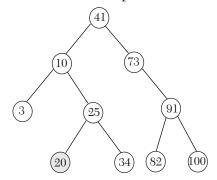
Figure 8.15. Searching a node with value 20 in the binary search tree.
