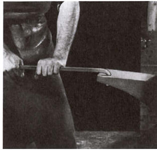
2. Use pritchel hole to bend pegs 90° in opposite directions.
