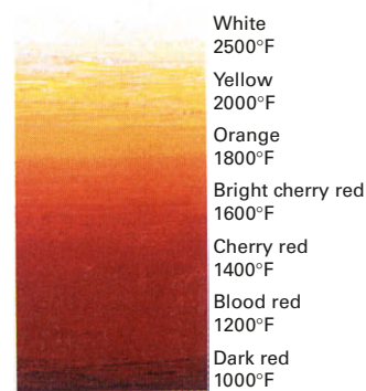
Incandescent color spectrum for forging iron and steel is best seen in semidarkness.
