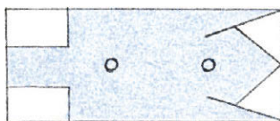
Mark pattern of doorplate with soapstone or chalk on 4- by 10-in. piece of 1/4-in. mild steel.
