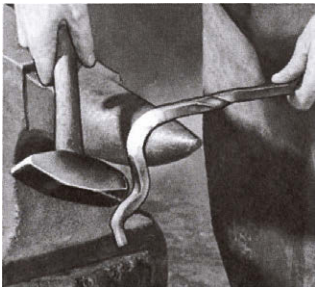
5. Forge arc over horn, quenching existing bends as you proceed.
