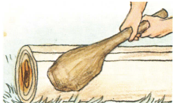
2. Pound log end vigorously with wooden club until strip ends separate, then pound between score lines all along log.
