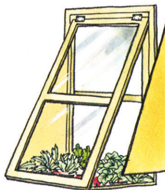
Secure corners of sash with glue and dowels or with nails; reinforce with corner braces.
