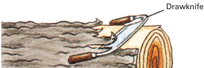
Drawknife is used to peel bark from whole log or from sections of a log that have been split into eighths.
