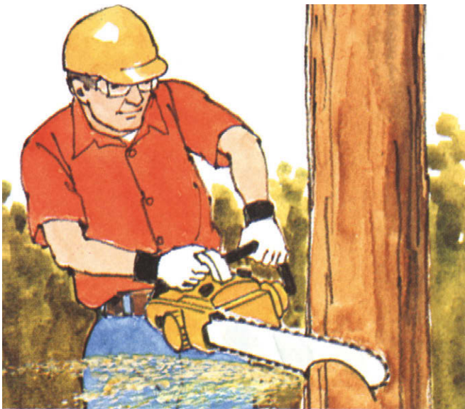
Chain-saw operator is in process of making a 45° angle face cut, the second of three cuts made when felling a tree.
