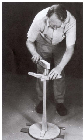
7. Insert stem pin into center hole in feet, and drive 3-in. wedge (Page 363). Trim excess with taped hacksaw blade and spokeshave. Chamfer top of stand slightly. Finish with scraper.
