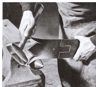
8. Forge flares outward at cherry-red heat. Quench. Cut top and punch.
