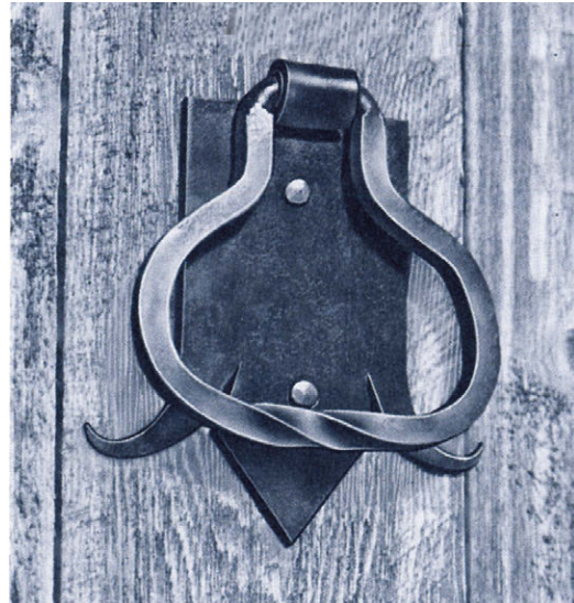
Handmade knocker can be attached to door with handmade nails, which are shown on Page 405.
