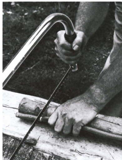
Set up shop in the woods around a solid improvised workbench. The crossed poles at end, one secured to a post driven into the ground and anchored by rocks, make an adjustable sawbuck.
