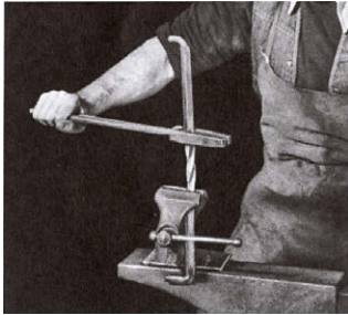
3. Heat 3-in. section in center of bar and apply half-twist (Page 408).
