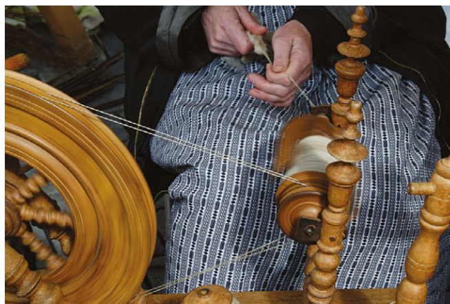
Low wheel twists fleece into yarn and winds it onto spindle in a continuous sequence. Many spinners enjoy the relaxed rhythm of treadling almost as much as the yarn that results.
