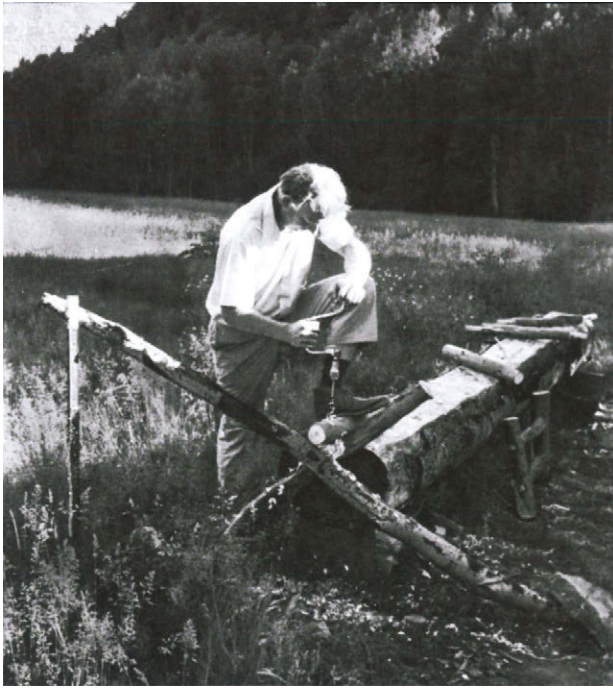
Set up shop in the woods around a solid improvised workbench. The crossed poles at end, one secured to a post driven into the ground and anchored by rocks, make an adjustable sawbuck.
