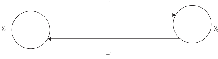
Figure 11.51 A network with asymmetric weights ( w_{12} \neq w_{21} ).
