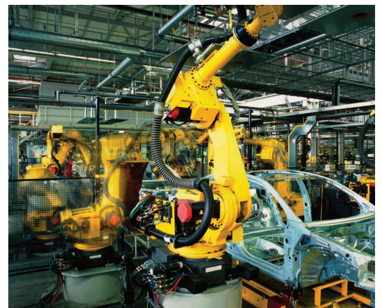
Figure 14.7 Robot arms assisting manufacture of assembly line automobiles.
