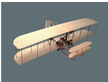
Figure 17.1 Wright brothers' airplane. This early model presented a two-tiered wing.
