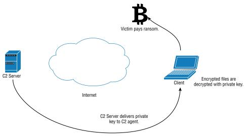
Figure 5-4: Decryption process flow.
