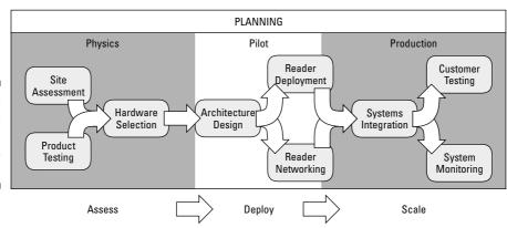
Figure 1-3: The Four Ps of an RFID Network Deployment.
