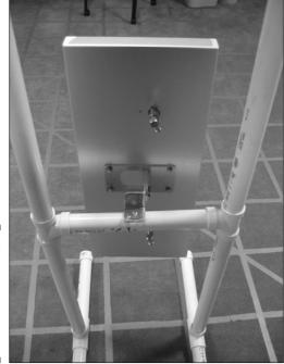
Figure 8-4: A homemade, freestanding PVC antenna rack.
