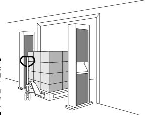
Figure 6-1: A typical dock door setup using a premade RFID rack.
