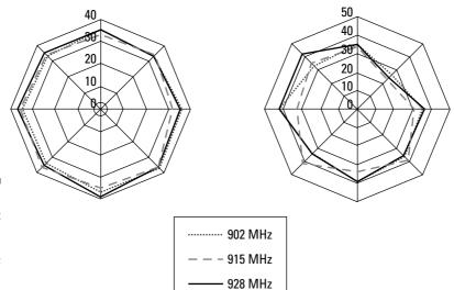
Figure 7-5: The perfect RF field graph and a typical RF test graph.
