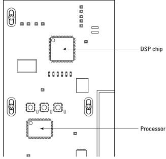
Figure 5-3: Inside an RFID reader, with the DSP and processor chip noted.
