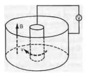
Fig. 5.1b. Faraday later discovered that a conductor moving through a magnetic field will produce a current between the outside and axis of the disk.
