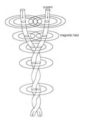
Fig. 1.11. An electrical current creates a magnetic field around it, while a magnetic field bends an electrical current. These effects permit parallel currents in a plasma to attract each other and twist into a plasma vortex filament with magnetic fields and electrical currents in the same helical pattern.
