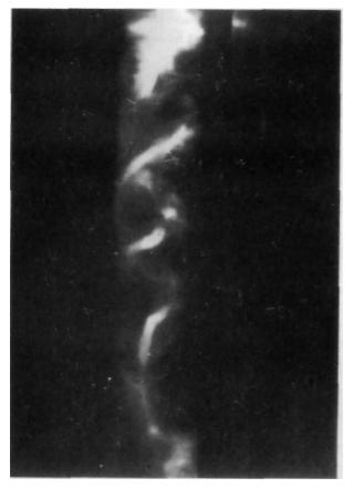
Fig. 6.6. In the Blackjack V experiments, current flowing through wire filaments creates a plasma, which twists itself up into a spiral form. In this photograph the plasma is seen by the X-rays it emits.
