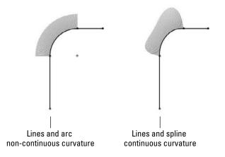
Notice how in Figure 7.46, the curvature comb immediately jumps from no curvature to the constant arc radius, but the spline image ramps up to a curvature that varies.
