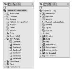
The most notable difference is that the Insert Bends part starts off with non-sheet metal features. The Rip feature also stands out, but the Rip feature is not exclusive to sheet metal. Although you can use Rip on any model, it is found only on the Sheet Metal toolbar.
