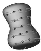
Using a Direction 2 for a curve-driven pattern creates a result similar to that in Figure 8.17. This is another situation that, although rare, is good to know about.
