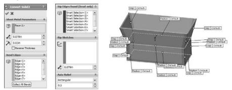
This tool is very useful for imported geometry and for parts with tricky shapes. Although the PropertyManager interface looks busy, it is fairly straight forward to use. Your first selection in the top Fixed Entity box should be a stable face, preferably an outer face on the bottom or the top. Inner faces generally do not work.
