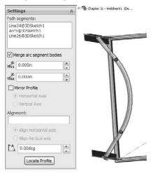
If the Merge arc segment bodies option is not selected, then a separate body is created for arc segments. The Merge arc segment bodies option applies to the whole feature, and cannot be set selectively for individual arc segments within the selected sketch entities; it is either on for all or off for all. If some arc segment bodies should be merged and others should not, then you should create separate Structural Member features.
