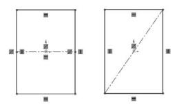
TO make a rectangle work like a square, use an Equal sketch relation on two adjacent sides. This only requires a single dimension to drive the size of the square.
