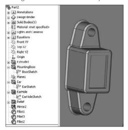
Notice that a plane has been added. The plane is made to only reference geometry that is internal to the library feature; it is perpendicular to an edge at the midpoint, which simultaneously locates and orients the plane correctly to enable it to be used to mirror the Ear feature.
