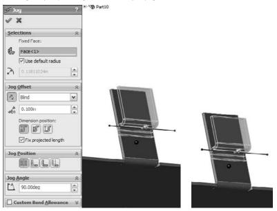
The Jog feature is created from a single sketch line on the face of a sheet metal part. The geometry to be jogged should not have any side bends; it should be a simple tab-like flange, as shown in Figure 29.19. The line to create the jog can be drawn at an angle, causing the jog to also be angled.
