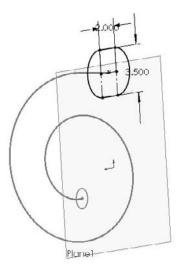
**13.** One of the goals of these edits is to smooth out the part. Remember that the Deviation Analysis told you that the edges created between the lines and arcs in Sketch3 were not very tangent. For this reason, it would be a good idea to replace the lines and arcs in Sketch3 with another Fit Spline.
