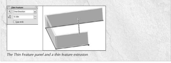
The Cap Ends option is available only when you specify a Thin Feature to be created from a closed loop sketch. This creates a hollow, solid body in a single step. You can also use Thin Features with cuts, and they are very useful for creating slots or grooves.
