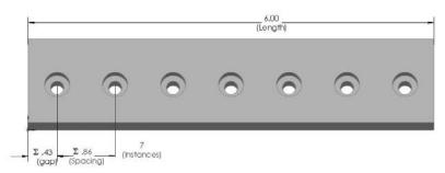
In this case, more sophistication has not been implemented to account for the diameter of the holes possibly interfering with one another when there are a large number of holes. In other words, because there are two values that need to be calculated (the spacing and the gap), you need to create two equations. Because the gap dimension is always half of the spacing, the spacing needs to be calculated first, as follows:
