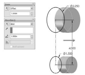
These steps produce multiple bodies that will be merged in a later step. Multiplebody parts are covered in more detail in Chapter 26. You can tell that there are multiple bodies by looking at the Solid Bodies folder near the top of the tree, and expanding the folder. The bodies are listed in the folder.
