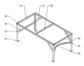
Also shown in Figure 31.18 is an auto-ballooned isometric view of the entire weldment. This works the same way that assembly auto-ballooning works, and it also corresponds to the Cut list in the same way as the assembly corresponds to the BOM.
