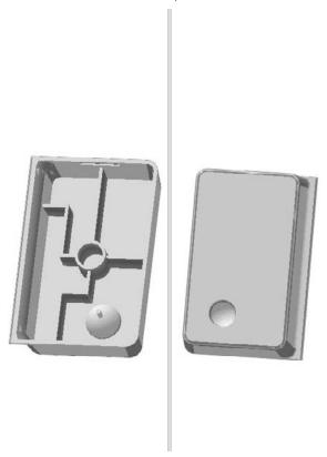
The Treat corners as zero thickness option should always be on. I have never seen a situation where turning it off improved the results; in fact, I have found that turning it off has always made corners and fillets behave worse.
