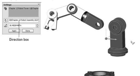
To explode the subassembly as a single part and then reuse its explode steps from the subassembly file, ensure that the Select sub-assembly's parts option is off, as shown in Figure 14.16.
