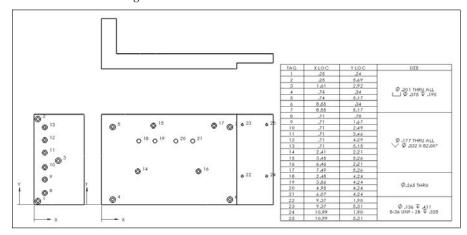
To initiate the Hole Table function, you must first select a view. You can access the Hole Table function through Insert
