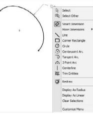
Diameter. You can create the dimension by selecting a complete circle and placing the dimension. If you want a diameter dimension for an arc, use the right-mouse button menu or Dimension Properties dialog box and select the Diameter Dimension option.
