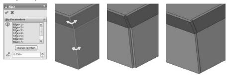
Notice also in Figure 30.3 that after the Rip, the edges of the material are still sheared at an angle. Because the top of the part was shelled, the thickness of the part is not normal to the main face of the sheet metal. You can fix this by using the Flatten Bends feature, which lays the entire part out flat, calculates the bend areas, and corrects any discrepancies at the edges of the part.
