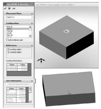
After the locating edges have been identified, the Locating Dimensions box becomes active, and you can change the values of the dimensions to locate the feature. Further, in the Size Dimensions pane at the bottom of the PropertyManager, clicking the Override dimension values option allows you to change dimensions of the feature itself.
