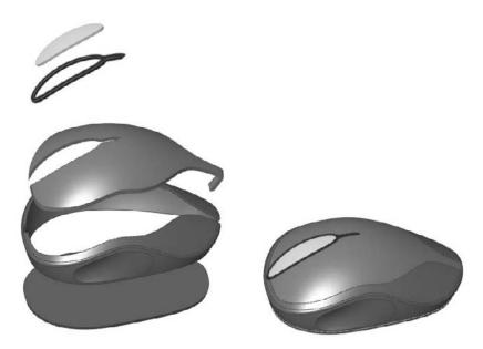
The part shown in Figure 26.1 is not complete, but the starting point for each part has been formed. This part was created from surface features that are discussed in detail in Chapter 27. The part is named Chapter 26 – Mouse Base Part.SLDPRT and is located on the CD-ROM. You may find it interesting to open the part to see how it has been modeled.
