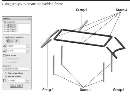
The main advantage of the new groups functionality is that each member within the group is automatically trimmed to other members of the group, and the control of gaps within or between groups. The only trimming you need to take care of separately is the trimming between members of different groups.
