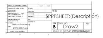
The syntax \$PRP or \$PRPSHEET indicates that the property that follows the syntax is to be pulled from either the current document (drawing) or from the model specified in the Sheet Properties, respectively. This is an important distinction to make. Most of the time, custom properties are typed in at the part or assembly level so that the data can be reused by drawing properties, BOM, or even design tables.
