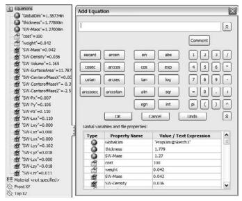
In the equation editor shown on the right in Figure 9.12, you can expand the list of global, custom and default properties for easy selection and placement into equations. Any custom properties you add that are of the type "number" are automatically added to this list, and can also be used in equations. Notice that the custom property "cost" is a property saved in my template and gets picked up for use here.
