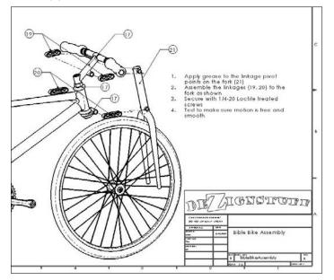
This is certainly a task that is different from the initial design or modeling of the assembly, and it may require an entirely separate model. Generally, you can perform the different steps by using a separate configuration for each process step, with exploded views for each configuration.
