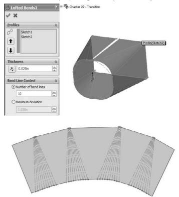
Like the forming tools, you can also use Lofted Bends in situations for which they were probably not intended. Figure 29.31 shows how lofting between 3D curves can also create shapes that can be flattened in SolidWorks. In this case, a couple of intermediate steps were required to get to the 3D curves, which involve surface features.
