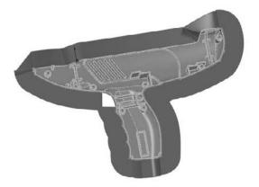
From this you can learn that the SolidWorks Mold Tools are not reliable for concave parting lines or non-planar parting lines. Flat parting line disks and boxes work well. Beyond that, expect to need to do some manual surface modeling.
