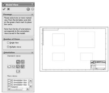
This is really useful functionality. It makes view selection and placement very easy and is visually clear. Unfortunately, the Single View setting is the default setting, and the PropertyManager does not remember the last setting that was used. Still, the combination of Multiple Views and Orientation is far better, in my opinion, than the View Palette, which I find visually confusing and non-intuitive.
