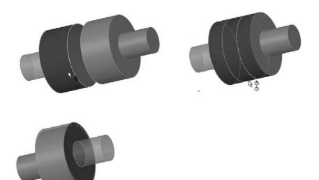
When you drop the face or edge onto the mating face or edge to complete the mate, you must use the popup Mate toolbar to accept or alter the mate. In the examples in Figure 13.6, a face is being dragged onto another face. However, you can also drag edges and vertices. Mates are limited to being either Coincident or Concentric.
