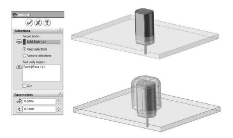
In this case, the small motor is placed where it needs to be, but there is a wall in the way. Indent is used to create an indentation in the wall using the same wall thickness, and placing a gap of .010 inches around the motor. The motor is brought into the wall part using the Insert  $\Rightarrow$  Part command. This is a multibody technique. Multibodies are examined in detail in Chapter 26.
