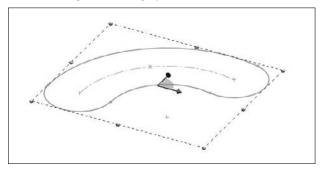
When Instant 3D is activated, double-clicking a sketch in either the FeatureManager or on a sketch element in the graphics window opens that sketch. While you are in a sketch, if you double-click with the Select cursor in blank space in the graphics window, you close the sketch. This only works for 2D sketches; 3D sketches can be opened, but not closed this way.
