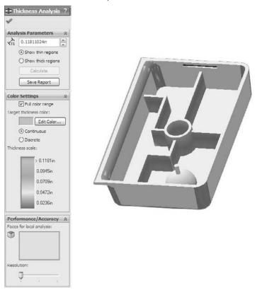
One of the things to watch out for here is that some anomalies occur when you apply this analysis to filleted faces. The faces shown as colored were created by the Shell feature and should be exactly .100 inches thick. However, it does correctly represent the undercut on the end of the part and the thickness of the ribs. A nice addition to this tool would be the identification of minimum thickness faces. Perhaps you can submit another enhancement request.
