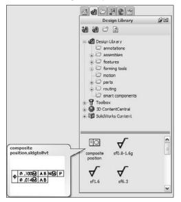
Each block has an insertion point, which snaps to any sketch entity point, even if it is in another block. This makes schematics easy to snap together. If the default insertion point is not the point that you need to snap to the other geometry, then you can place the block anywhere on the drawing and drag the point that needs to snap.
