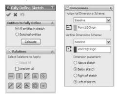
If you are familiar with older versions, the Fully Define Sketch function was formerly called Auto Dimension, and has absorbed the functionality of Scan Equal and Add Relations. This function is very useful when used with imported data. If you do not like the automatic dimensioning scheme, you can at least take advantage of the automatic sketch relations.
