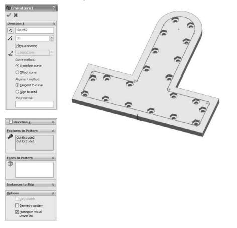
Figure 8.15 shows the same part using the Transform Curve positioning option and Tangent to Curve alignment option.
