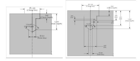
Remember that to get the diameter dimensions shown in Figure 18.15 (instead of radius dimensions), you must use the dimension tool to select the centerline (construction line) and the line or endpoint on one side, and then move the cursor to the other side of the centerline to place the dimension (the order of selection does not matter). When the cursor crosses the centerline, the dimension will display as a diameter instead of a radius.
