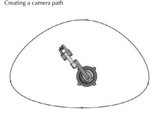
**NOTE** To greatly simplify this task, you can create an offset plane, and sketch an ellipse or circle on the plane rather than using the 3D spline. The 3D spline is intended to give you the most control and flexibility.
