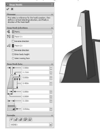
This feature uses a 3D sketch point where you made the selection in Step 1. You cannot dimension this point while setting up the feature, only by creating the feature and then going back and editing the 3D sketch absorbed under the feature. This is also the arrangement with the Lip/Groove. Remember that you cannot dimension 3D sketches the same way that you dimension 2D sketches. You may need to dimension to planes rather than edges or points to get the dimensions you really intend.
