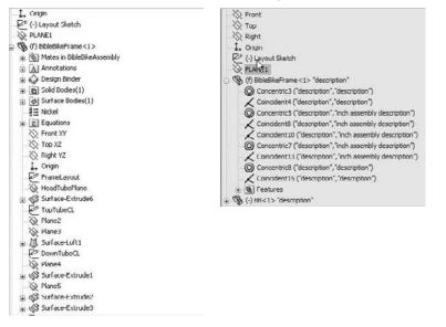
Another technique for displaying mates is to split the FeatureManager and to show the PropertyManager in one pane. As a result, any parts that are selected show their mates in the PropertyManager pane. If two selected parts have mates in common, then the common mates appear in bold type, as shown in Figure 12.16. This is an extremely useful method for looking at mates.
