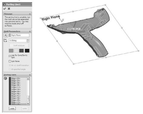
The Parting Lines feature can also split faces if need be. You might need to split a face that straddles the parting line. For example, a filleted face might bridge across the parting line and need to be split.
