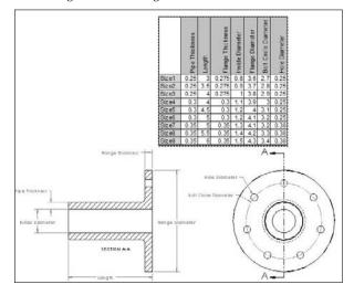
This drawing uses a part Design Table, but you can also place assembly Design Tables onto the drawing. This type of drawing is often called a tabulated drawing.
