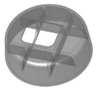
The Indent feature can be problematic if it breaks into multiple areas as it does in this part, due to the ribbing on the underside of the target body. Notice that in the PropertyManager in Figure 26.4, two selections were made in the Tool Body Region selection box. The tool body is selected on either side of the rib that bisects the tool. This concept is not very intuitive, and you may have to play with the part and the options to understand what it is doing.
