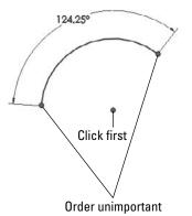
• Arc Length. You can create the dimension by selecting an arc and its endpoints with the Smart Dimension tool.
