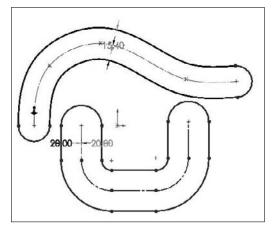
In addition to the bi-directional offset with capped ends, SolidWorks also has slot sketch entities for straight and curved slots, which you can find covered later in this chapter. Composite slots (made of a combination of straight and curved sections) still require the offset method.
