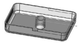
**To create a Step Draft, initiate a Draft feature.** Use the Step draft option. Select Perpendicular Steps. The draft angle should be 2 degrees. The direction of pull is the top thickness face of the box. Parting lines are the six edges of the split. Make sure all the yellow arrows are pointing to the same side of the split edges. Figure 32.33 shows the Step Draft in action.
