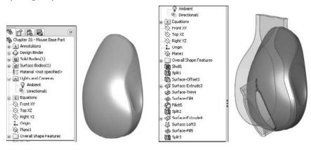
To go from the multi-body part created here to a set of separate parts uses a Master Model function, which is described in Chapter 28.
