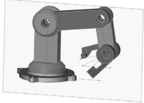
This particular assembly is driven by two sketches on different planes to govern the position of the parts. Keep in mind that this assembly has been used for all of the other techniques as well, and so all of these techniques can exist together simultaneously, being controlled by configurations.
