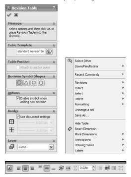
You can add a revision to the table by right-clicking the table and selecting Revisions Add Revision. This includes control over whether the revision uses numerical or alphabetical revision levels, but does not provide for more complex revisioning schemes.
