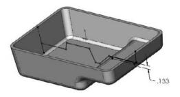
At the ends of the shell, the intersection curves serve to give the sketch a reference point to be fully defined. Under the right end of the rib sketch, the intersection curve gives you a reference to dimension the height of the rib in the shallower section of the part. The part shown in Figure 32.7 is on the CD-ROM as Chapter 32 - skyline.sldprt.
