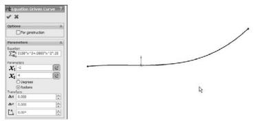
Use regular mathematical notation and order of operations to write the equation. X1 and X2 are for the beginning and end of the curve. Use the transform options at the bottom of the PropertyManager to move the entire curve in X, Y or rotation. To specify X = f(Y) (instead of Y = f(X)), use a 90 degree transform.
