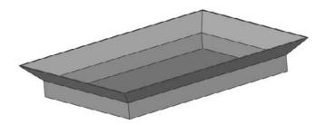
**5.** Use the Rip feature to rip out the four corners. Allow the Rip to rip all corners in both directions. The part should now look like Figure 30.9.
