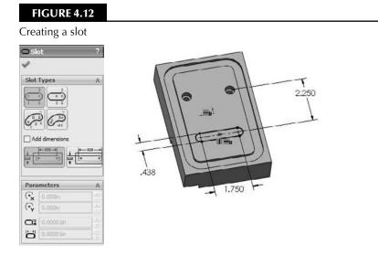
**3.** Open a sketch on the bottom of the previous slot, and draw a straight slot. You can create a cut using the Through All end condition.
