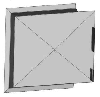
**18.** Create a new configuration named Flat. In this configuration, suppress the forming tool that you just placed, and unsuppress the Flat Pattern feature at the bottom of the tree.
