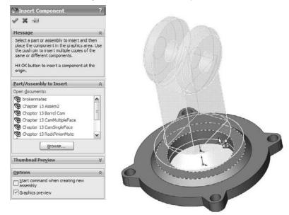
A Mate reference being used to SmartMate a component
