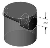
To force a 3D dimension to have a certain orientation, dimension from a plane or planar face rather than from an edge, vertex, or sketch entity. A dimension from a plane is always measured in a direction perpendicular to the plane, but a dimension from a line or point is always measured by the shortest distance between the entities. Two-dimensional sketches can force dimensions to be horizontal or vertical, but 3D sketches cannot.
