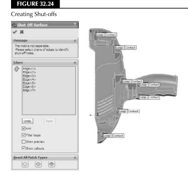
When all appropriate edges around all of the holes and slots are selected, the Shut-off Surfaces PropertyManager message window turns green and says "The mold is separable into core and cavity."
