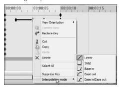
The icons for the modes should be self-explanatory. My only complaint is that the Ease out icon seems upside down. In any case, curves make smoother motion than lines. Ease in/Ease out create the smoothest motion; Ease in works best at the beginning of a change, and Ease out works best at the end of a change. Snap and Linear should be self-explanatory.
