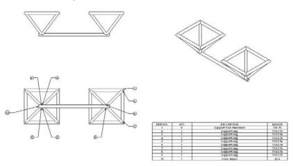
**NOTE** Relative views are difficult to create with round pipe rather than rectangular tube, although starting with 2007, planes can be used as references for relative views.
