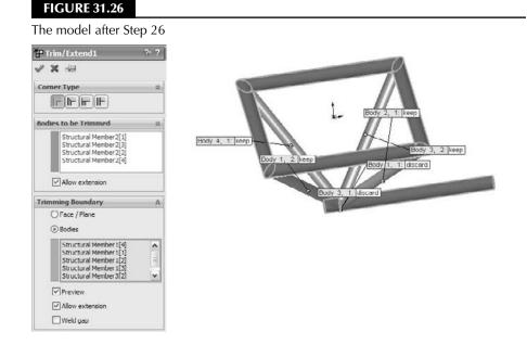
**28.** Half of the support structure has been modeled to this point. You can create the rest of it by mirroring the existing bodies. Create a Mirror feature, using the free end of the 10-foot-long member as the mirror plane, and selecting all of the bodies in the Bodies to Mirror selection box. Do not use the Merge Solids option, as you will need to do this manually. Click OK to accept the feature when it is set up properly. The PropertyManager for the Mirror feature is shown in Figure 31.27.
