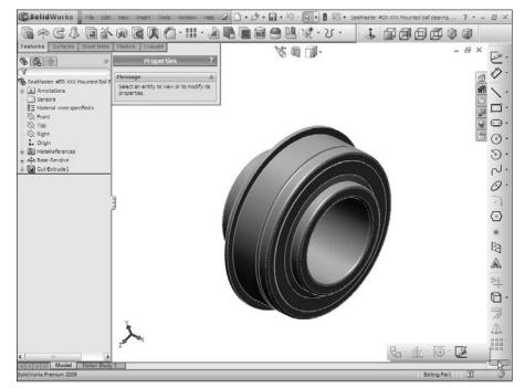
The small flyout in the lower-right corner of Figure 2.44 is the remainder of the Sketch toolbar that does not fit on the screen. This screen shot was taken on a 12-inch monitor with large icons at  $1024 \times 768$  resolution. At such a low resolution, long toolbars do not fit on the screen, and the remaining icons are activated by the two small arrows at the end of the toolbar.
