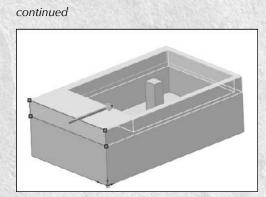
The Up to Next end condition used with a Cut extrude
