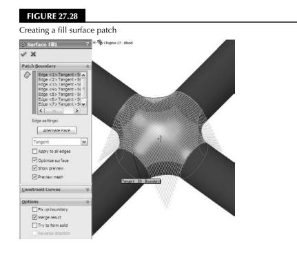
The Optimize Surface option is ignored for this part because the opening is eightsided rather than four-sided. Also note that you may have to change the resolution control slider to get the surface to remain convex instead of going concave in the center.
