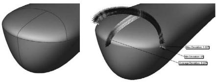
While Deviation Analysis helps to quantitatively measure how close to tangent the faces on either side of the selected edge are, you must still run Zebra Stripes to get the complete picture of the flow between faces. Both tests have to return good results to have an acceptable face transition.
