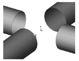
**6.** Initiate the Lofted Surface feature, and select the nearest edge segments from adjacent tubes. If the loft preview twists, then use the light-blue handles to straighten it out, or deselect and reselect one of the edges in approximately the same location as the other edge was selected. Expand the End Conditions panel and set each edge to use the Curvature setting. You may adjust the End Tangent Length option if you want, but keep in mind that this may make the part asymmetrical.
