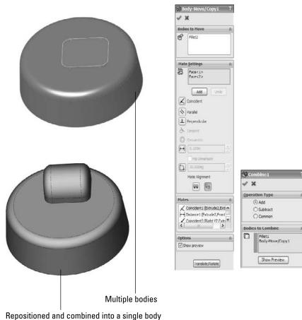
In this case, the Move/Copy Bodies feature uses mates. These mates enable you to locate bodies in a way similar to the way they are used in assemblies. One important difference is that with bodies, you must use the actual body geometry of the body that is moving; you cannot use reference geometry such as planes. By clicking the Translate/Rotate button at the bottom of the PropertyManager, you can also position bodies using distances and angles.
