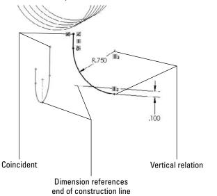
**6.** Exit the sketch and create a projected curve. The Projected Curve function is found at Insert +> Curve +> Projected Curve. Use the Sketch on Sketch option.
