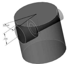
**12.** Create an AlongY sketch relation between the points indicated in Figure 17.7. The hole centerpoint on the cylindrical face is one of the points, as well as the endpoint of the angled line. Change the angle dimension to ensure that it is controlling the sketch point as expected.
