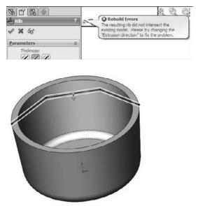
The reason for the error shown in Figure 32.10 is that even though the rib sketch intersects the edge of the part, the width of the top of the rib would go past the edge and not intersect anything. One way to deal with this is to make the sketch intersect the part a little closer to the center of the part from the edge. Another way would be to put a short vertical line at the end of the rib.
