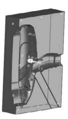
Again, you can save out these core pins as individual part files. You can use similar techniques to create side cores or lifters or other types of side actions.
