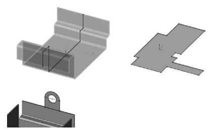
Notice that the sketch of the part at the upper left of Figure 29.1 shown in preview has all sharp corners, and that the bend radius is automatically added to each corner by the software. SolidWorks automatically adjusts when bend directions are combined to make sure that the inside radius is always the same, regardless of bend direction.
