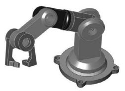
Through the course of this chapter, the robot arm assembly has greatly increased in complexity, but it has retained the original information that was in the first version. Maintaining valid assembly data through manually managed configurations is difficult, and all it takes is a simple mistake to wipe out a lot of assembly configuration data. Appropriately, the next section discusses assembly design tables.
