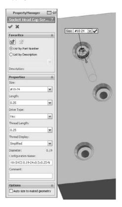
Toolbox parts will even automatically size themselves based on the hole. It is best to use Hole Wizard holes if you are going to use this function of Toolbox parts. Hole Wizard and Toolbox are meant to work together.
