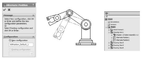
To create an Alternate Position view, ensure that you have an assembly on the active drawing that can have multiple positions, and click the Alternate Position View button from the Drawings toolbar, or select the same tool at Insert r Drawing View r Alternate Position.
