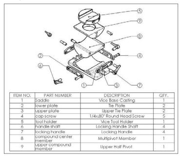
BOMs are made in one of two ways. The default BOM is made from a special SolidWorks table, while an Excel-based BOM is driven by Excel. While Excel has advantages and disadvantages, many users appear to prefer the default BOM. The reason is that little is perceived to be given up, except for the stability (crash-worthiness) compared to Excel and the options to keep manual edits.
