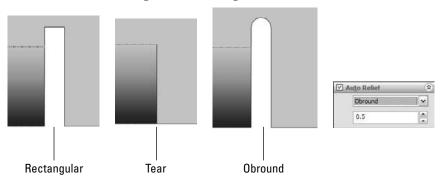
For the Rectangular and Obround types, you can control the width and the distance past the tangent line of the bend through the Relief Ratio selection box, which is immediately below the type selection box in the Sheet Metal PropertyManager. This ratio is the width of the relief divided by the part thickness. For the Rectangular relief, a ratio of .5 and a thickness of .050 inches means that the relief is .025 inches wide and that it goes .025 inches deeper into the part
