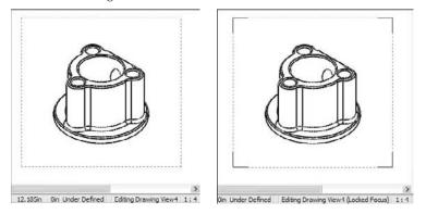
If a view is not activated or the focus is not locked on the view, then any sketch elements that you draw will be placed on the drawing sheet. While sketching in a drawing view, it is a good practice to watch the status bar.
