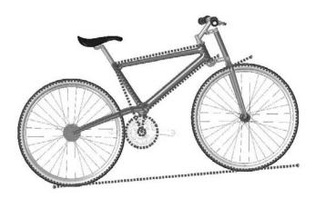
One of the drawbacks of this technique is that you give up dynamic assembly motion. To move the parts, you have to move the sketch. The part does not move until the sketch is updated. If you need to combine layout functionality with dynamic assembly motion, see the Layout feature in Chapter 16.
