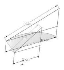
From this point, you can calculate the flat pattern again, using SolidWorks' sketch-solving capabilities as the calculator. Think of the auger as being the cardboard tube inside a roll of paper towels. If you examine one of these tubes closely, you see that it is simply a straight and flat strip of cardboard that has been wound around a cylinder. What was the flat, straight edge of the original board is wound into a helix. This method is simply reversing that process.
