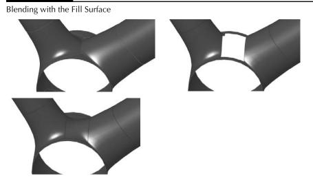
In Figure 27.19, a solid starts with a Split line on the surface. A sketch is then added, and a fill surface is created using the sketch as a constraint and the Split line as the boundary. The Merge Result option in the Fill PropertyManager has a different significance than it does in a solid feature PropertyManager, but the end result is the same. Remember that this is a surface function, and if it does not merge, then it is left as a surface feature.
