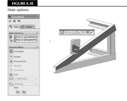
**5.** Select the Coincident mate, and then the faces as shown in the figure. If the machined part is turned as it is in Figure 4.18 (so that it interferes with the welded frame if the selected surfaces touch), then click the Flip Mate Alignment button on the popup toolbar or toggle the Mate Alignment buttons in the PropertyManager. Close the popup toolbar by clicking the green check mark icon.
