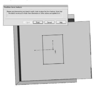
**17.** Double-click the new feature in the FeatureManager; a set of dimensions appear on the screen. Change the 4-inch dimension to 13.9 inches, and the 6-inch dimension to 11.9 inches. The cross break should now look like Figure 29.39.
