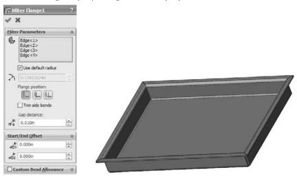
A Miter Flange feature starts off with a sketch that is perpendicular to the starting edge of the Miter Flange feature.
