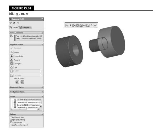
To edit multiple mates consecutively without exiting the Mate PropertyManager, it is best if you pre-select the mates. Pre-selected mates are shown in the Mates panel, as shown in Figure 13.20. You can switch from editing one mate to another by simply selecting the new mate in the Mates panel. If you select only one mate before clicking Edit Feature, but realize later that you want to edit multiple mates, you can select more mates through the FeatureManager.
