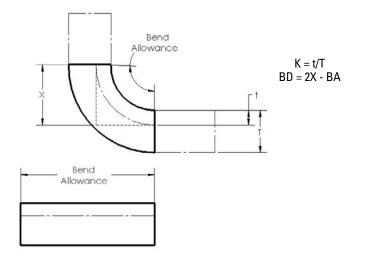
The three values are related, as shown in Figure 29.6. The dark rectangle represents the bend area. Material outside of the bend area really does not matter, although it is usually shown and used in the generally accepted formulas about bend calculations for sheet metal.
