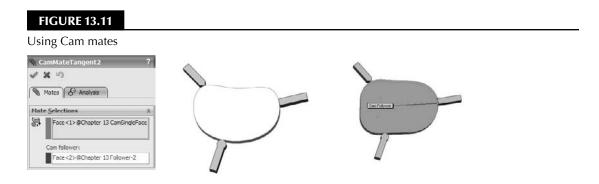
If you open the assemblies and spin the cam plate, you will notice that in both cases, the flat follower does not work very well. In fact, in the single face cam assembly, it does not work at all.
