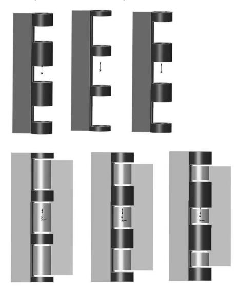
The problem here is that you can only show the size of the second hinge plate that corresponds to the configuration of the first plate that is active in the assembly. If you had two instances of the hinge assembly in a top-level assembly, then you would be able to show only one size for the second plate.
