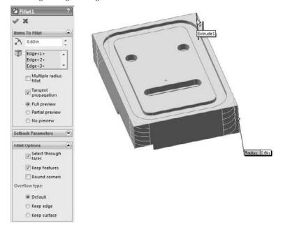
Feature order is important with features like chamfers and fillets because of how they both tend to propagate around tangent edges. Although you can turn this setting off for both types of feature, it is best to get the correct geometry by applying the features in order.
