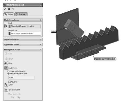
Applying a Rack and Pinion mate
