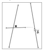
Construction Geometry toggles between regular sketch entities and construction entities. Construction sketch entities are not used to create solid or surface faces directly; they are only used for reference for example, revolve centerlines, extrude and pattern directions, and so forth. Be careful with the icon for this function, because it looks almost identical to the No Solve Move icon, especially as printed here in gray scale.
