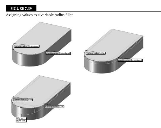
By default, the variable radius fillet puts five points on an edge, one at each endpoint, one at the midpoint, and one each halfway between the ends and middle. If you want to create an additional control point, there are three ways to do this:
