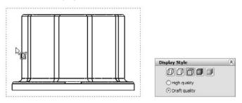
You can access the Cosmetic Thread Display setting in both the Step 1 PropertyManager and the Step 2 PropertyManager. However, you need to be careful not to misread the interface, by thinking that either of these interfaces controls the View Quality. The best advice for using the view quality settings is to forget about them. It looks like this function is being phased out or at least discouraged.
