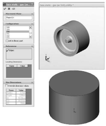
Next, in the Design Library, browse to features, then inch, and then the fluid power ports folder, and drag the sae j1926-1 feature onto the end of the extruded rectangle. Select the 38-24 size from the configurations list. A window appears, prompting you for reference selections, as shown in Figure 18.4.
