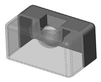
Another familiar situation is when you have a feature to place and you want to use an Offset from Surface end condition, but the feature spans two faces. In that situation, you can knit the necessary faces together (or use offset), and then extrude offset from that surface body.
