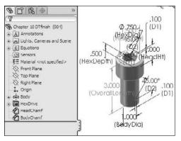
You can use one of the following three techniques to add a design table to a SolidWorks part through the menu selection Insert (> Tables (> Design Tables:
