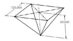
**12.** Rotate the view slightly. Notice that the first line that you drew in Step 10 and one other line are on a plane. Drag a right to left selection box around the point where the four lines converge, and assign an Equal relation to all of the lines. This makes the shape into an upside-down pyramid shape.
