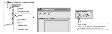
To initiate the Explode Line Sketch function, you can select Insert > Explode Line Sketch. This displays the Explode Sketch toolbar and the Route Line PropertyManager interface. Creating nice
