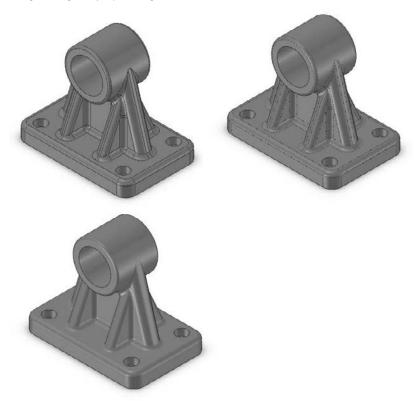
Using the Tangent Edges as Phantom setting is a quick and easy way to look at a model to determine whether or not face transitions are tangent. It does not help to distinguish between tangency and curvature continuity; you need to use Zebra Stripes for that.
