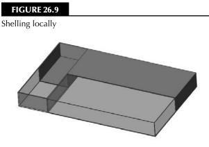
To shell the part this way with feature order, you create one block and shell it, and then create the other block and shell that. In order for this technique to work, the second shell needs to be as big as, or bigger than, the first shell. If it is smaller, then it will (or may) hollow out areas that are not intended to be hollow.
