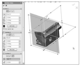
Clicking the check mark icon in the Section View PropertyManager enables you to continue working with the sectioned model, although you may not be able to reference edges or faces that are created by the section view. It is only a displayed section; the actual geometry is not cut.
