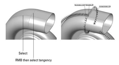
The maximum deviation is about ten degrees, which is far too much. This part needs to be smoothed out, which you can do using splines in place of lines and arcs.
