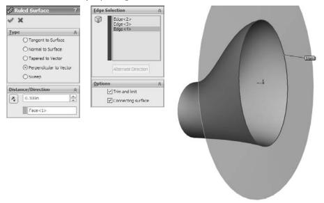
The Ruled Surface works from the edge of a solid or surface body. The feature has five basic types of operation that it can perform:
