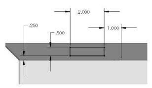
**8.** Use the sketch to create a Through All cut in one direction. Notice that the Normal cut option is on by default. Examine the finished cut closely; notice that it is different from the default type of cut because it is not made in a direction normal to the sketch, but rather in a direction normal to the face of the part. Details of this are shown in Figure 30.11.
