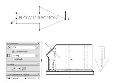
**6.** Place the block using the Insert Block function, so that the block is to the right of the right view. Once you place it, press Esc to cancel the placement of more blocks. Then select the block to activate the PropertyManager. Deselect the Lock Angle option, and set the angle to 270 degrees.
