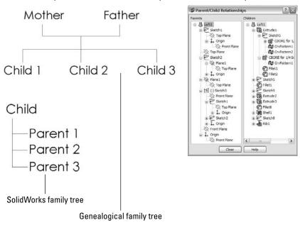
You can display the parent-child relations between SolidWorks features as shown in Figure 11.2 by opening the right-mouse button menu on any feature, and selecting Parent/Child. This helps you to determine relationships before editing or deleting, so that you can see which features will be removed or go dangling.
