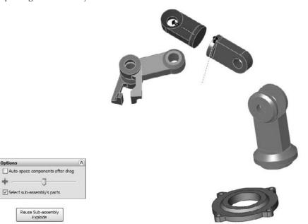
Turn on the Select sub-assembly's parts option, select one gripper, Alt+drag the triad to set the direction, and then drag the distance of the explode. If you are in the mood to submit an enhancement request to SolidWorks, then you may want to request a Symmetrical Explode function for situations such as this. Figure 14.17 shows the finished result of the explode.
