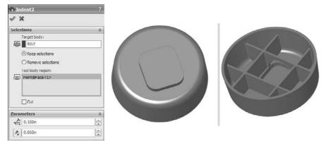
Also notice that toggling the Keep and Remove selections options means that only one region of the tool body would need to be selected to create the original result shown in Figure 26.4.
