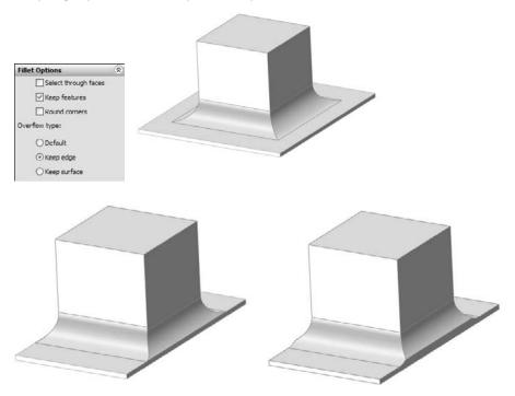
The Default option chooses the best option for a particular situation. As a result, it seems to use the Keep Edge option unless it does not work, in which case it changes to the Keep Surface option.
