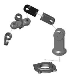
You can animate the explode or collapse from the right-mouse button menu. To do this, right-click the exploded view, and select Animate Explode or Animate Collapse. This method does not offer recording or Photoworks rendering like Animator software, but it is fast and easy. You cannot see explode lines during an animation.
