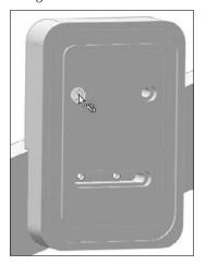
**14.** Now click the underside of the screw head and the counterbored surface of the slot, make sure that they will be coincident, and click OK. Repeat the process for the other screw.
