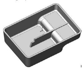
A final termination situation that I want to mention is one that can sometimes happen at curved edges. If the extension of the rib can not be contained by the model, the rib will fail. This is not always as obvious a situation as you might think. When a non-horizontal rib intersects a curved edge, it usually forces you to fake something a little. Figure 32.10 shows an example of why this is.
