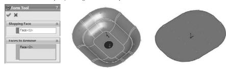
The Stopping Face turns a special color, and so do any faces that are selected in the Faces to Remove selection box. Faces to Remove means that those faces will be cutouts in the sheet metal part.
