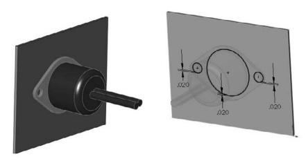
**4.** Next, edit the dummy part in context (right-click the dummy part in the assembly and select Edit Part), and offset edges of the connector part to extrude a cut, as shown in Figure 19.8 in the image to the right. Offset the two mounting holes and the area around where the connector will stick through the sheet metal by about .02 inches.
