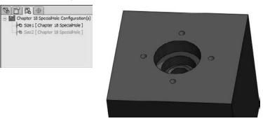
**17.** Auto-create a design table by selecting Insert → Design Table, and then selecting the Auto-Create option. Edit the design table to look like Figure 18.18. Hide or delete extra columns that don't match the data shown.
