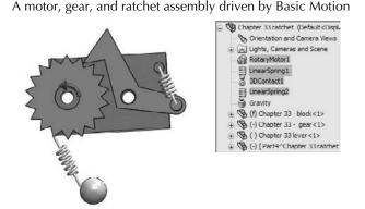
To set up this example, apply a counterclockwise motor to the inside circular edge of the gear, and select the block as the part to move relative to. In this case, I started the motor with a slow rpm (revolutions per minute), moved the time bar out a few seconds, and assigned a faster speed, so the motor speeds up over time.
