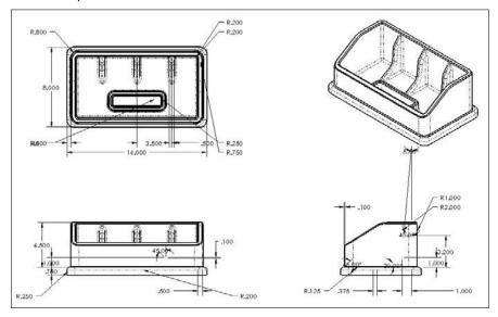
To move a dimension to another view, you can Shift-drag it from one view to the other (make sure that the dimension is appropriate in the destination view). To copy a dimension, you can Ctrl-drag it. If you cannot place the dimension in the view that you have dragged it to, then the cursor will indicate this with a special cursor symbol.
