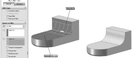
Face fillets are sometimes amazing at covering over a mess of geometry that you might think you could never fillet. The main limitation on fillets of this type is that the fillet must be *big* enough to bridge the gap. That's right, I said *big* enough. Face fillets can fail if they are either too small or too large. Figure 7.44 shows a complex fillet situation that is completely covered by a face fillet.
