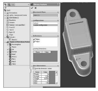
Once you place a library feature on a part, it can be edited, unless you select the Link to library part option in the Configuration pane, in which case the feature is driven externally from the \*.sldlfp file. Link to library part is only available when the feature is first placed; it is not available when you edit an existing library feature in a part.
