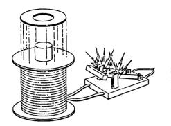
Figure 5.2. Faraday stresses at work. When the electromagnet is connected to an alternating current, the aluminum ring flies into the air.
