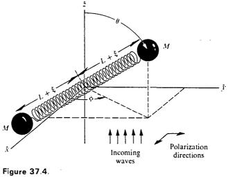
An idealized detector (vibrator) responding to linearly polarized gravitational waves,
