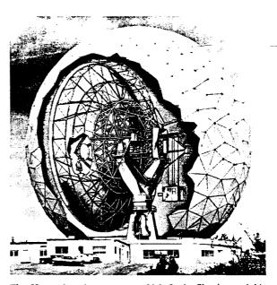
The Haystack radar antenna, which Irwin Shapiro and his group have used to collect extensive data on the systematics of the inner part of the solar system. Those data are rapidly becoming the most important source of information about perihelion shifts. (Picture courtesy of Lincoln Laboratories, MIT.)
