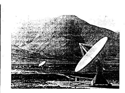
The 90-foot (background) and 130-foot (foreground) radio interferometer system at Caltech's Owens Valley Radio Observatory. These were used by Seielstadt, Sramek, and Weiler (1970) in their pioneering measurement of the deflection of quasar radio waves by the sun. During the experiment the two antennas were separated by 1.07 kilometers. (Photo by Alan Moffet.)
