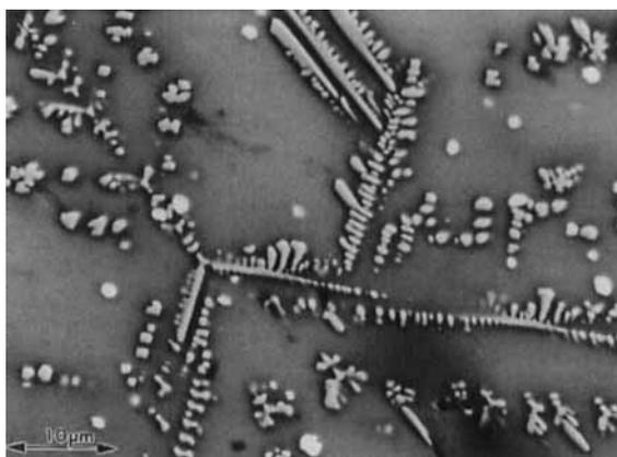
**Figure 8.** BSE Z-contrast image of Assyrian glass showing Cu<sub>2</sub>O dendrites. Recorded on Cambridge S250 SEM at 10 keV.
