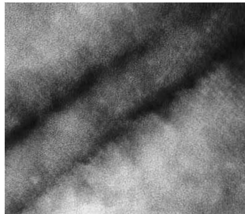
**Figure 31.** Image of a dissociated  $60^\circ$  dislocation in silicon. In between the  $30^\circ$  and  $90^\circ$  partials, different sets of 0.33 nm fringes are visible. These fringes are caused by forbidden  $(\bar{4}22)/3$  reflections and contain high-resolution information about the dislocation cores. (Courtesy of J. C. H. Spence.)
