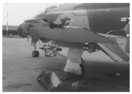
**P-12** Another view of aircraft 68-8789 damage (photo taken at Ubon). Extensive damage to the wing can be seen. Notice that the ADSIDs carried by the aircraft are gone from the racks visible in the bottom photo. The crew completed the mission and returned safely to base, a testament to the dedication of aircrews supporting Igloo White.
