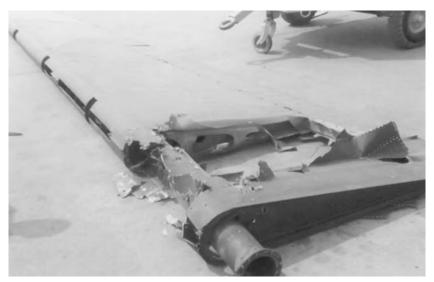
**P-24** Photo (taken in Ubon, 1969) of the same AC-130 showing the removed left-hand elevator. It was damaged by antiaircraft fire while on an Igloo White support mission. All AC-130 aircraft at Ubon were painted flat black, with flat red military lettering.
