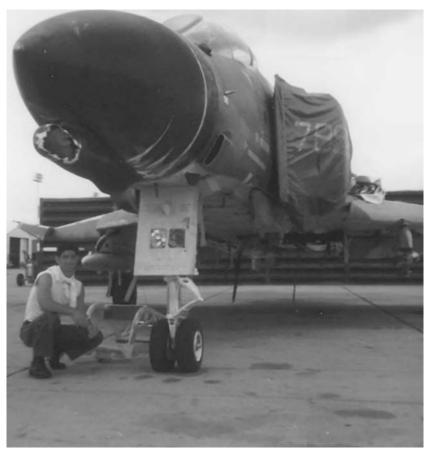
**P-11** Front view of the aircraft previously described. The crew chief is in front of the aircraft, and the damaged radome is evident in the photo.
