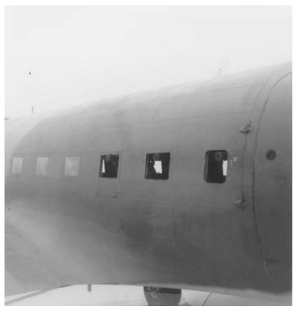
**P-22** Close-up view of the gun ports on the AC-47. The windows of the original C-47 were removed so that the three 7.62-mm mini-guns could fire through the openings. A rudimentary optical sight was mounted on the instrument panel in front of the pilot.
