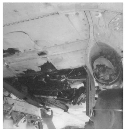
**P-10** This 25th Tactical Fighter Squadron F-4D, serial number 68-8789, flew into trees over Laos during a high-speed, low-altitude sensor drop mission in early 1969. The aircraft is seen parked on the ramp at Ubon Royal Thai Air Base, Thailand. Although the aircraft was heavily damaged, the aircrew was able to fly it back to base. Notice the damaged AIM-7 missile radome at the right-hand side of the photo.
