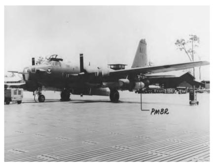
Two Wright R-3350-32W turbocompound radial engines, producing in excess of 3,000 takeoff-rated horsepower each, powered the OP-2E.
