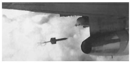
**P-19** Sensor drop from the left wing of an OP-2E over Laos, courtesy USAF. The sensor has just been released, and its antenna retaining rings are still in place as the sensor falls to the earth.
