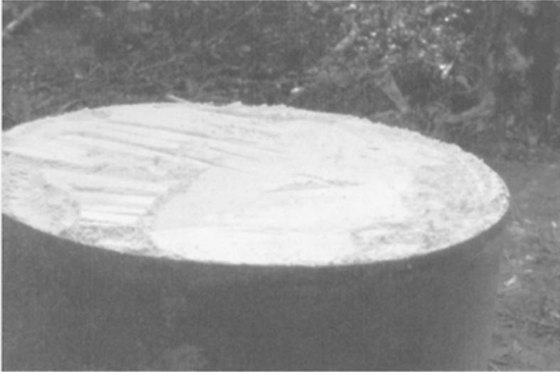
**FIGURE 9.22** Suction cups are embedded in the diatomaceous clay.
