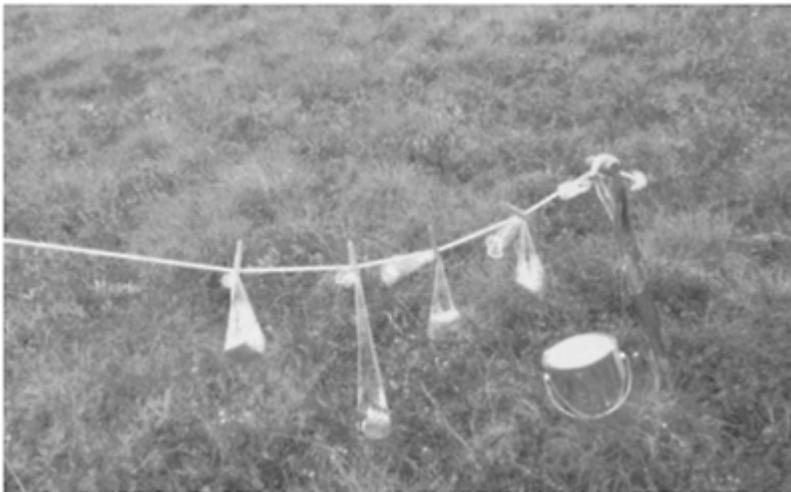
**FIGURE 7.7** The cold method is a useful technique to determine soil bulk density under field conditions. The
