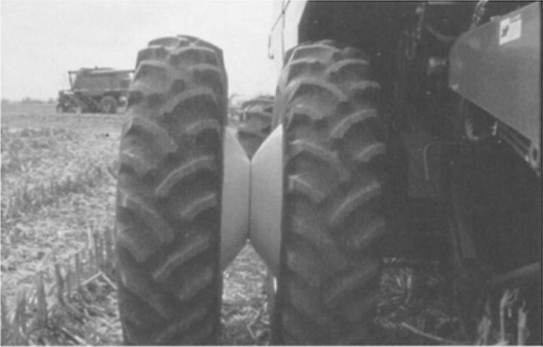
**FIGURE 7.13** The vehicle load can be distributed over a large area by using dual tires. The soil compaction hazard is less when the load is distributed over a large area.
