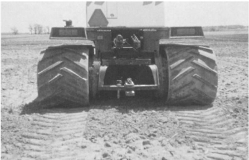
**FIGURE 7.14** Similar to dual tires, wide tires can also distribute the load over a large area. Nonetheless, the
