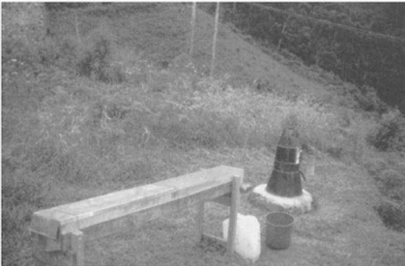
**FIGURE 9.11** Recording and non-recording rain gauges.
