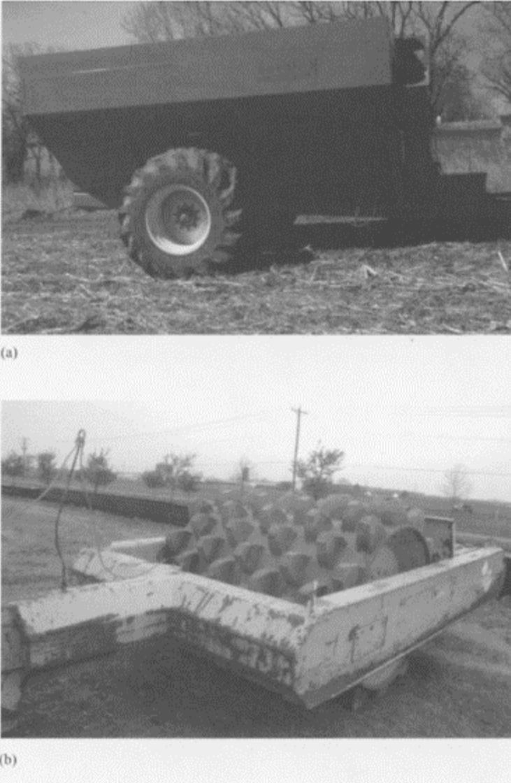
**FIGURE 7.5** (a) A single-axle grain cart with capacity of 10 or 20 Mg can cause severe compaction during harvest in the fall, (b) A kneading roller is used to create a compact road bed. Spikes cause more compaction than a smooth roller.
