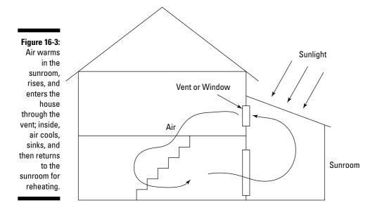
Vent fans can enhance the chimney effect. Solar-powered ceiling fans work well because they don't need to be hard-wired (no code problems or expenses associated with electricians), plus they work hardest when the sun is hottest, which is usually what you want.
