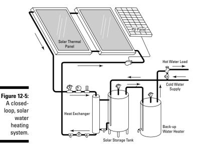
The flat-plate collectors can be mounted in almost any configuration, at great distances from the exchanger. The closed loop is always full of fluid, so the pump pressure requirements are much easier than those for a drainback system.
