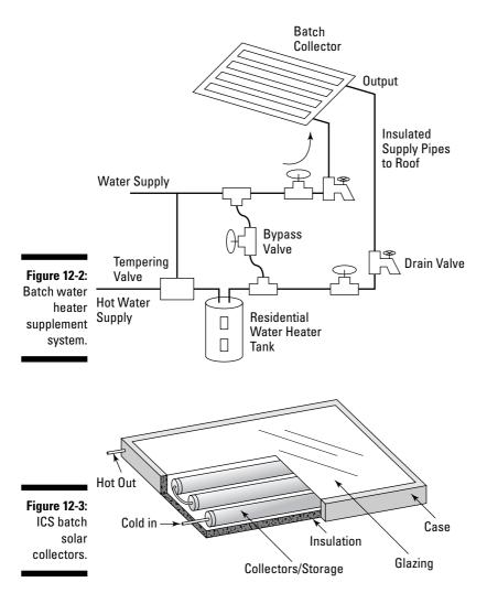
Complete kits include all the valves, plus the collector and its associated mounting hardware. If you do opt to do it yourself, give some serious consideration to how you'll lift the collector (even empty, they weight a lot) wherever you plan on mounting it. The collector can weigh upwards of 500 pounds when full of water (which means the units can withstand winds of up to 180 mph!). Make sure that your roof can take this weight. You don't want to find out the hard way that it can't.
