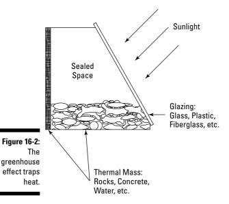
Sunlight enters the enclosed space through the glazing (window) and then gets absorbed and stored as heat energy. The heat is then constrained to stay in the enclosed space via the same glazing's insulation properties, plus insulation in the walls. You can enhance the greenhouse effect by increasing the amount of radiation the window allows to enter while maximizing the glass's insulation against heat.
