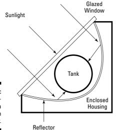
**Figure 10-2:** A crosssection of a batch collector.
