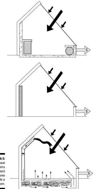
Figure 16-5: Storing heat maintains consistent temperatures inside a solar room.
