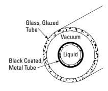
Figure 10-4: Construction details of an evacuated tube collector.
