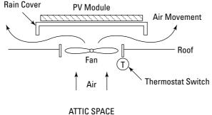
One-piece attic vent fans are very simple to install; you don't even need to go into the attic space. Simply cut a round hole in your roof, pull the shingles back, slide the unit up under the shingles, and drop it into the hole. Seal for weatherproofing, and you're done.
