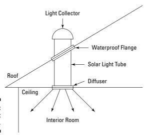
Figure 9-2: A solar light tube system.
