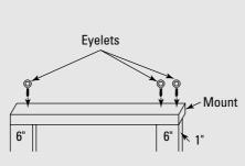
Drill 3 holes, attach eyelets
