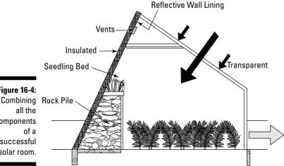
Figure 16-4: all the components of a successful solar room.
