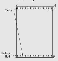
Tack screen onto roll-up rod and mount
