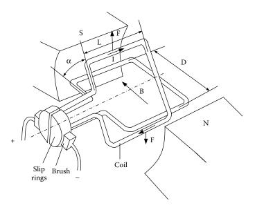
FIGURE 6.3 Operation principle of a DC motor.
