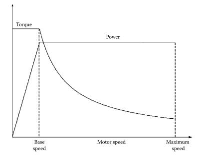
FIGURE 16.5 Typical torque and power profiles of traction motor versus motor speed.
