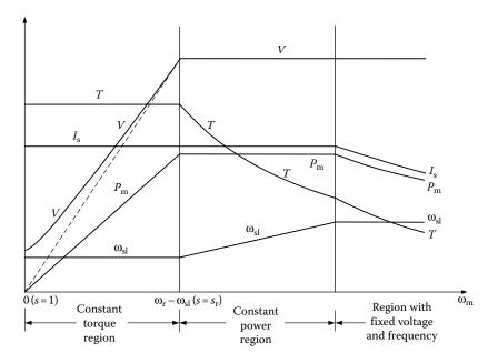
FIGURE 6.19 Operating variables varying with motor speed.
