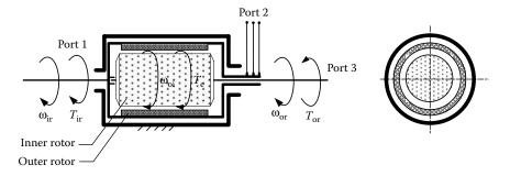
FIGURE 5.17 Transmotor used as a speed coupler.
