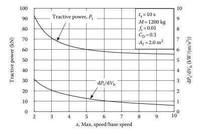
FIGURE 4.9 Power rating versus speed factor.
