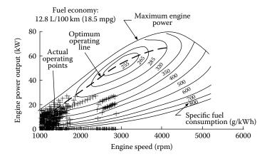
**FIGURE 2.34** Fuel economy and engine operating points in EPA FTP75 urban drive cycle overlapped on engine fuel consumption characteristics map.
