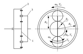
FIGURE 5.15 Planetary gear unit used as a speed-coupling device.
