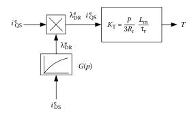
FIGURE 6.26 Block diagram of a field-orientated induction motor.
