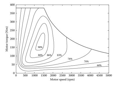
FIGURE 4.14 Typical electric motor efficiency characteristics.
