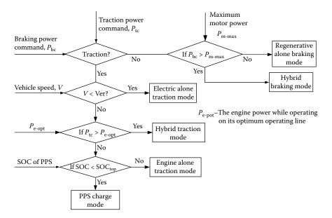
FIGURE 8.4 Flowchart of Max. SOC-of-PPS control strategy.
