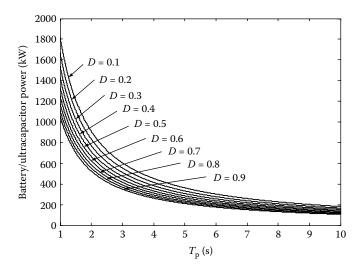
**FIGURE 16.16** Peaking power of the batteries for pulsed power load varying with *D* and *T*<sub>p</sub>.
