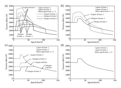
**FIGURE 5.9** Tractive effort along with vehicle speed with different transmission schemes: (a) two multigear transmissions, (b) multigear engine transmission and single-gear motor transmission, (c) single-gear engine transmission and multigear motor transmission, and (d) both single-gear transmissions.
