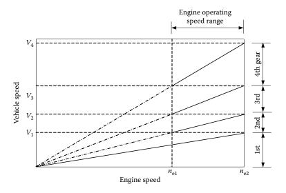
FIGURE 2.18 Demonstration of vehicle and speed ranges for each gear.
