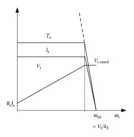
FIGURE 6.50 Speed-torque curve in the steady state with variable voltage supply.
