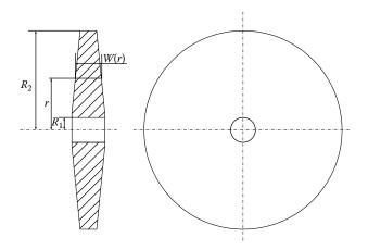
FIGURE 12.15 Geometry of a typical flywheel.
