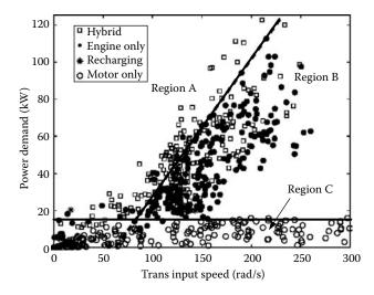
**FIGURE 8.10** Operating points of dynamic programming optimization over UDDSHDC cycle.<sup>12</sup>
