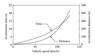
**FIGURE 2.29** Acceleration time and distance along with vehicle speed for an electric-machinepowered passenger car with single-gear transmission.
