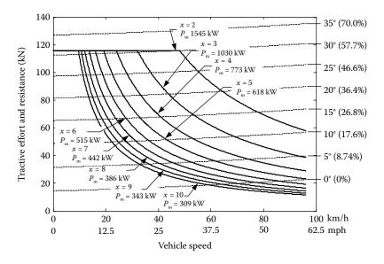
FIGURE 16.8 Tractive effort versus vehicle speed with different *x* and motor power.
