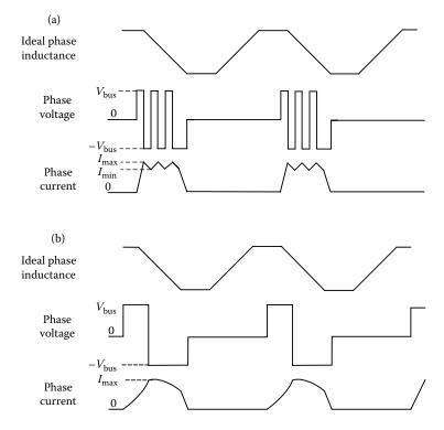
**FIGURE 6.67** Low- and high-speed operation in generating mode: (a) low speed operation and (b) high speed operation.
