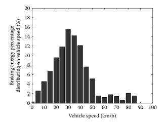
FIGURE 13.4 Braking energy distribution over vehicle speed in an FTP75 urban driving cycle.
