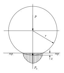
FIGURE 2.2 Pressure distribution in contact area.
