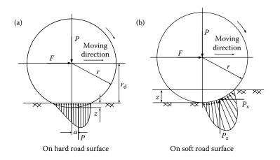
FIGURE 2.4 Tire deflection and rolling resistance on a (a) hard and (b) soft road surface.
