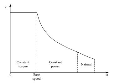
FIGURE 6.66 Torque-speed characteristic of SRM.
