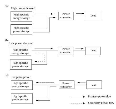
**FIGURE 12.18** Concept of a hybrid energy storage operation. (a) Hybrid powering, (b) power split, and (c) hybrid charging.
