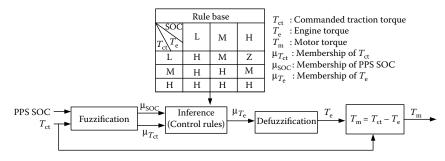
FIGURE 8.8 Block diagram of fuzzy logic control.
