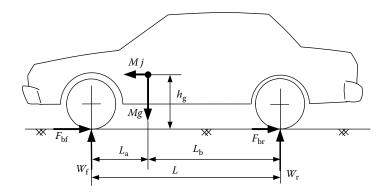
FIGURE 13.3 Forces acting on a vehicle in braking.
