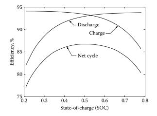
FIGURE 12.7 Typical battery charge and discharge efficiency.
