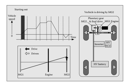
FIGURE A.14 Operation mode of starting out.
