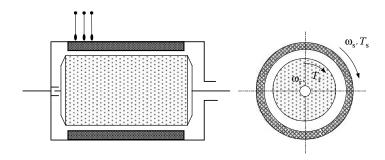
FIGURE 11.18 An electric motor with a floating stator.
