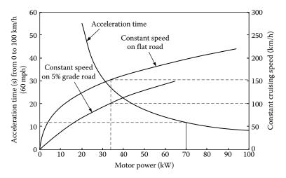
FIGURE 15.4 Motor power versus acceleration time and vehicle cruising speed.
