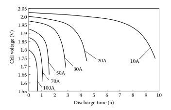
FIGURE 11.7 Discharge characteristics of the lead-acid battery.
