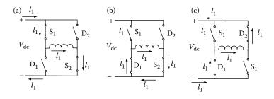
**FIGURE 6.63** Modes of operation for the classic converter: (a) turn-on mode, (b) zero voltage mode, and (c) turn-off mode.
