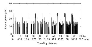
**FIGURE 10.17** Engine power versus traveling distance in FTP75 urban driving cycle with CD mode.
