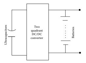
FIGURE 12.22 Actively controlled hybrid battery/ultracapacitor energy storage.
