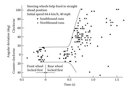
FIGURE 2.42 Angular deviation of a car when all four wheels do not lock at the same instant.
