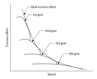
FIGURE 2.17 Tractive effort characteristics of a gasoline-engine-powered vehicle.
