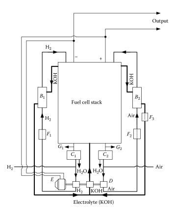
**FIGURE 14.7** Circulating electrolyte and supplies of hydrogen and air in an AFC;  $B_1$ ,  $B_2$ , heater exchangers;  $C_1$ ,  $C_2$ , condensers; D, pampers; E, motor;  $F_1$ ,  $F_2$ ,  $F_3$ , controls; and  $G_1$ ,  $G_2$ , outlets.<sup>8</sup>
