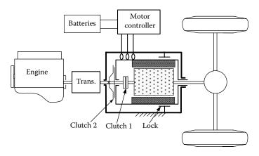
**FIGURE 5.22** Alternative torque- and speed-coupling hybrid electric drive train with a transmotor.
