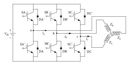
FIGURE 6.34 Circuit diagram of a three-phase voltage source inverter.
