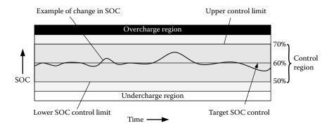
FIGURE A.3 Battery SOC control region.
