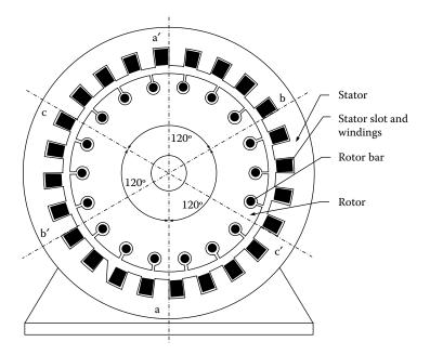
FIGURE 6.14 Cross section of an induction motor.
