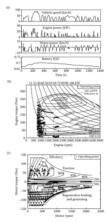
**FIGURE 11.11** Simulation in an FTP75 urban drive cycle: (a) vehicle speed, engine power, motor power, and battery SOC, (b) engine fuel consumption map and operating points, and (c) motor efficiency map and operating points.
