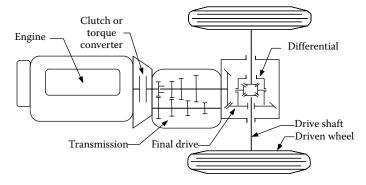
FIGURE 2.10 Conceptual illustration of an automobile power train.
