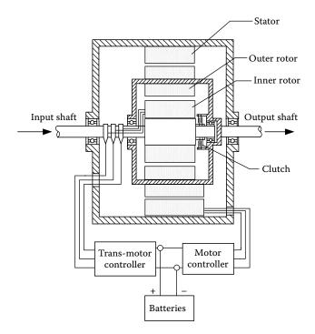
FIGURE 5.26 Integrated transmotor and traction motor.
