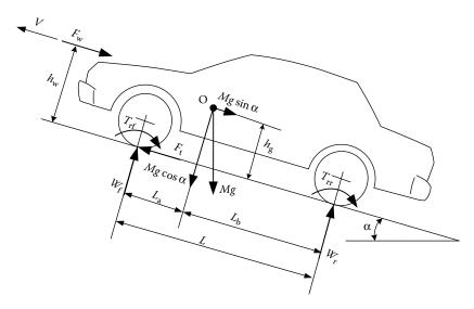
FIGURE 2.1 Forces acting on a vehicle moving uphill.
