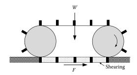
FIGURE 16.3 Shearing action of a track.
