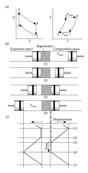
**FIGURE 3.17** Ideal Stirling cycle: (a) P-V and T-S diagram, (b) piston arrangement at the terminal points of the cycle, and (c) time-displacement diagram.
