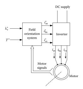
FIGURE 6.27 General block diagram of a vector control system for an induction motor.
