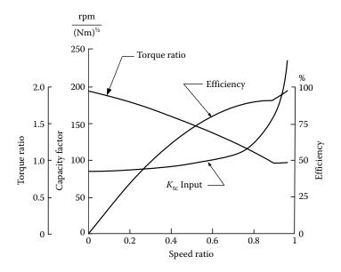
FIGURE 2.21 Performance characteristics of a torque converter.
