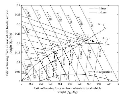
FIGURE 2.44 Braking process analysis on roads with different adhesive coefficients.
