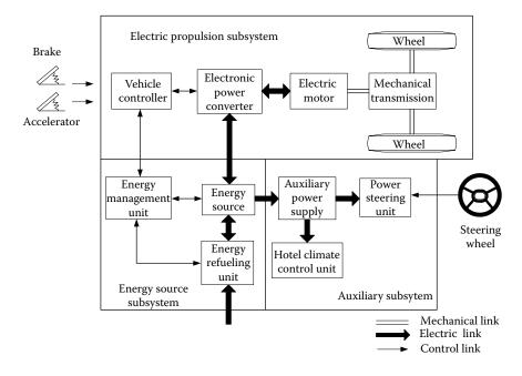
FIGURE 4.2 Conceptual illustration of a general EV configuration.<sup>1</sup>
