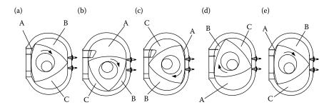
**FIGURE 3.15** The Wankle rotary engine cycle: (a) three separate working chambers and air/fuel intake into chamber A, (b) starting compression in chamber A, (c) ignition and starting expansion in chamber A, (d) starting exhaust in chamber A, and (e) starting intake in chamber A.
