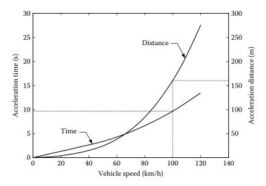
FIGURE 7.24 Acceleration time and distance versus vehicle speed.
