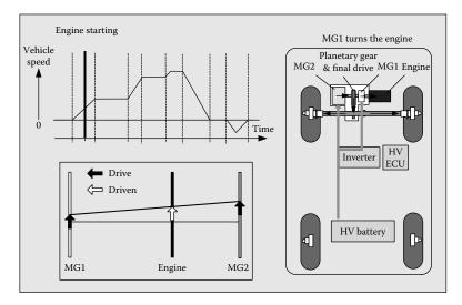
FIGURE A.15 Operation mode of engine starting.
