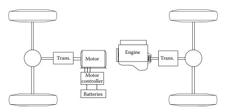
FIGURE 5.13 Separated axle torque combination parallel hybrid electric drive train.
