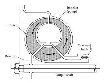
FIGURE 2.20 Schematic view of a torque converter.
