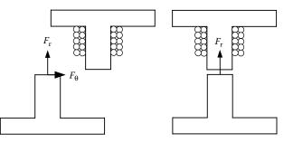
FIGURE 6.75 Static profile of the radial component of the force.
