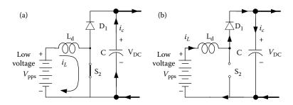
**FIGURE 7.11** Current flow during the on and off periods of  $S_2$  in the PPS discharging mode: (a) in  $S_2$  on period and (b) in  $S_2$  off period.
