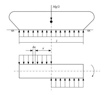
FIGURE 16.11 Moment of turning resistance of a track.
