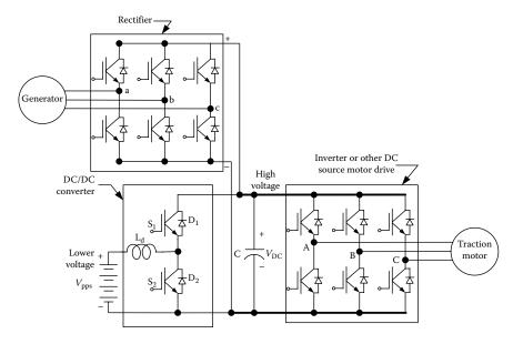
FIGURE 7.13 A boost/buck DC/DC converter.
