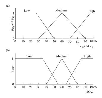
**FIGURE 8.9** Membership functions of (a)  $T_{ct}$ ,  $T_e$  and (b) SOC.
