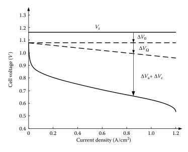
**FIGURE 14.3** Current–voltage curves for a hydrogen–oxygen fuel cell at  $T = 80^{\circ}$ C.
