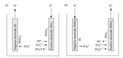
**FIGURE 12.4** Electrochemical processes of a lead–acid battery cell: (a) discharging and (b) charging.
