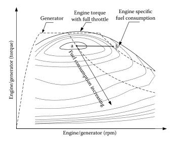
FIGURE 7.21 Operating point of the engine/generator.
