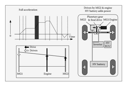
FIGURE A.18 Operation mode in full acceleration.
