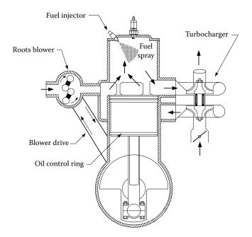
FIGURE 3.14 A supercharged and turbocharged fuel-injection 2S engine.
