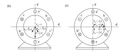
**FIGURE 6.16** Stator mmf vectors: (a) positive direction of each phase mmf; (b) stator mmf vectors at  $\omega t = 0$ ; (c) stator mmf vectors at  $\omega t = 90^{\circ}$ .
