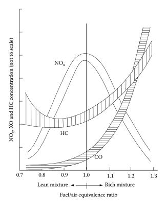
FIGURE 3.9 Fuel/air ratio effect on emissions.
