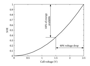
FIGURE 12.13 SOE versus cell voltage.
