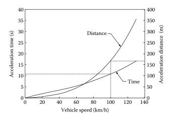
FIGURE 8.18 Acceleration time and distance versus vehicle speed.
