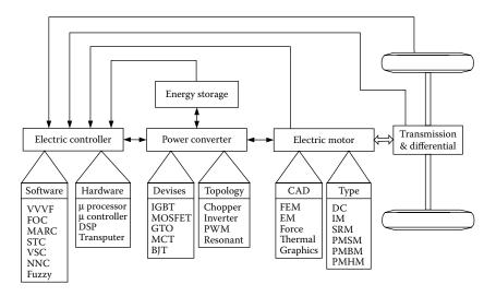
FIGURE 6.1 Functional block diagram of a typical electric propulsion system.<sup>1</sup>
