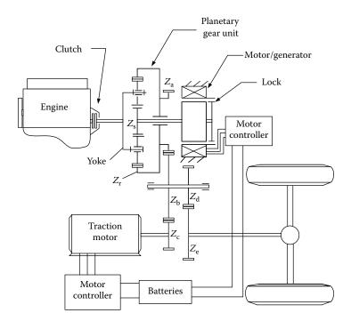
FIGURE 5.23 Integrated speed- and torque-coupling hybrid electric drive train.
