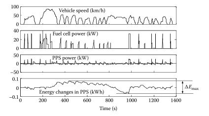
FIGURE 15.6 Vehicle speed, fuel cell power, power of the PPS, and energy changes in the PPS.
