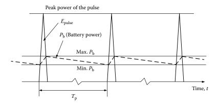
FIGURE 16.15 Conceptual illustration of the time profiles of pulsed power and battery power.
