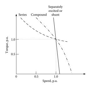
FIGURE 6.6 Speed characteristics of DC motors.
