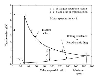
**FIGURE 4.7** Tractive effort versus vehicle speed with a traction motor of x = 4 and two-gear transmission.
