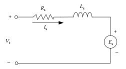
FIGURE 6.48 Simplified equivalent circuit of the BLDC motor.
