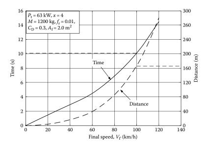
FIGURE 4.10 Acceleration time and distance versus final speed.
