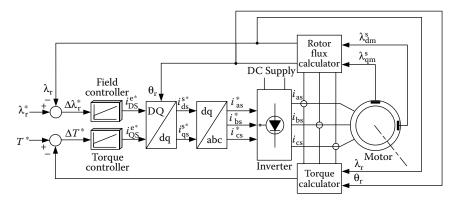
FIGURE 6.32 Vector control system for an induction motor with direct rotor flux orientation.
