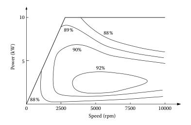
FIGURE 6.53 Optimal efficiency profiles of a PM hybrid motor drive.<sup>1</sup>
