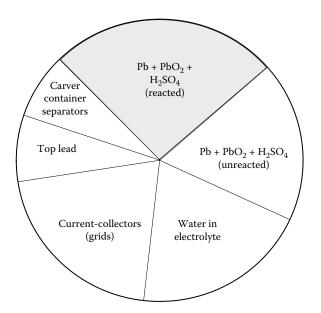
**FIGURE 12.5** Weight distribution of the components of a lead–acid EV battery with a specific energy of 45 Wh/kg at the C5/5 rate.<sup>1</sup>
