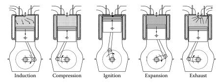
FIGURE 3.2 Four strokes of a spark-ignition engine.
