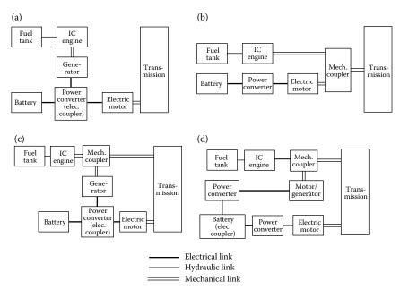
**FIGURE 5.3** Classifications of hybrid EVs. (a) Series (electrically coupling), (b) parallel (mechanical coupling), (c) series–parallel (mechanical and electrical coupling), and (d) complex (mechanical and electrical coupling).
