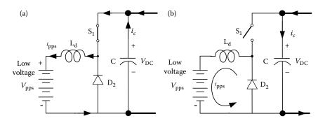
FIGURE 7.12 Current flow during the on and off periods of  $S_1$  in PPS charging mode: (a) in  $S_1$  on period and (b) in  $S_2$  off period.
