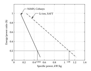
FIGURE 10.30 Typical energy/power ratios versus specific power.
