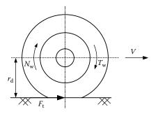
FIGURE 2.11 Tractive effort and torque on a driven wheel.
