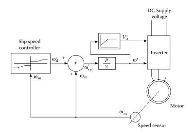
**FIGURE 6.20** General configuration of constant *V*/*f* control.
