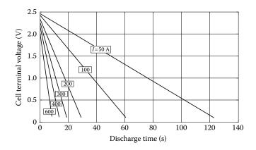
FIGURE 12.11 Discharge characteristics of the 2600F Maxwell Technologies ultracapacitor.
