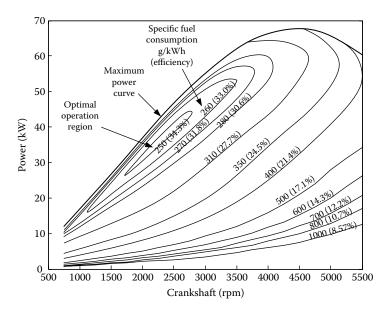
FIGURE 7.2 Example of engine characteristics and optimal operating region.
