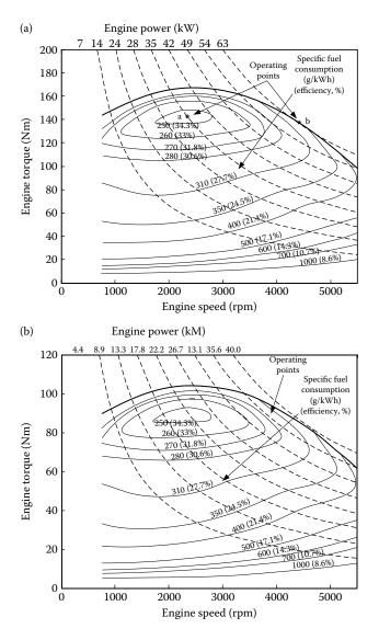
**FIGURE 7.27** Engine characteristics and operating points: (a) operating with best efficiency and (b) operating with close maximum power.
