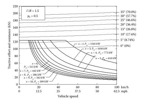
**FIGURE 16.13** Vehicle gradeability with steering versus vehicle speed with respect to various *x* and motor powers.
