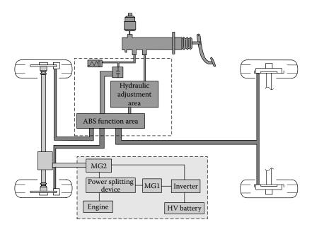
FIGURE A.8 The hybrid brake system.
