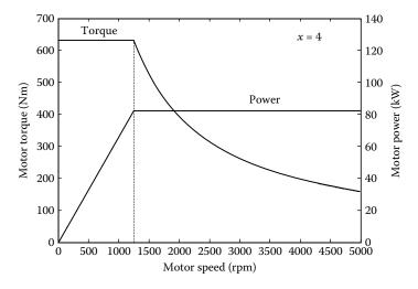
FIGURE 7.23 Characteristics of traction motor versus motor rpm.
