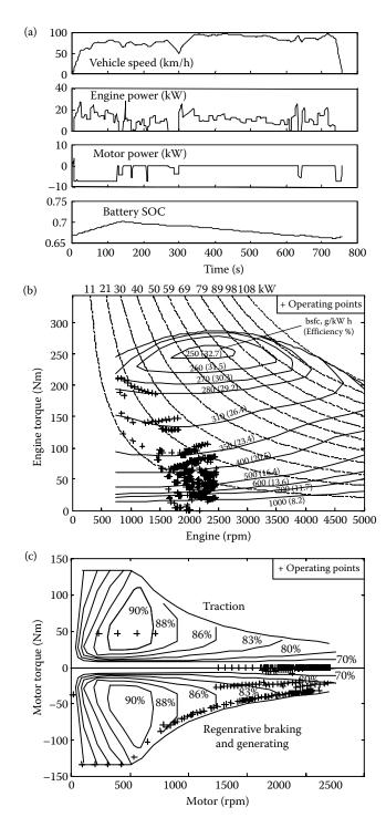
**FIGURE 11.12** Simulation in an FTP75 highway drive cycle: (a) vehicle speed, engine power, motor power, and battery SOC, (b) engine fuel consumption map and operating points, and (c) motor efficiency map and operating points.
