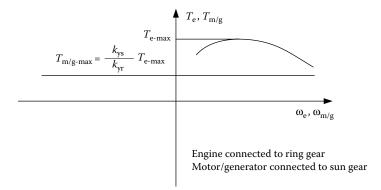
FIGURE 9.5 Operating areas of the engine and motor/generator.
