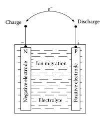
FIGURE 12.1 A typical electrochemical battery cell.
