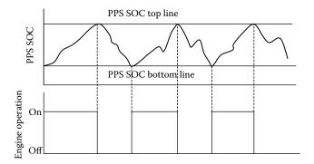
FIGURE 7.5 Illustration of thermostat control.
