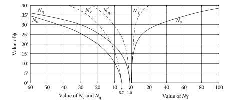
**FIGURE 16.2** Variation of terrain bearing capacity factors with angle of internal shearing resistance.<sup>1</sup>
