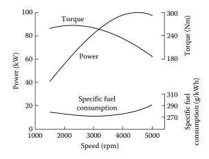
FIGURE 2.13 Typical performance characteristics of gasoline engines.
