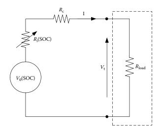
FIGURE 11.8 Battery model.
