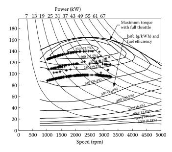
**FIGURE 10.13** Engine operating points overlapping its fuel consumption map in LA92 driving cycle with AER mode.
