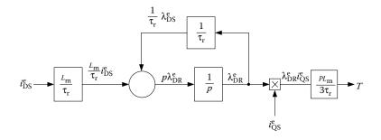
**FIGURE 6.25** Block diagram of an induction motor with  $\lambda_{OR}^{e} = 0$ .
