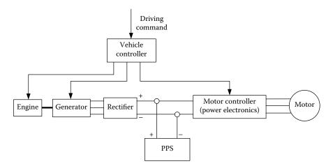
FIGURE 7.6 Directly connected power source and sink.
