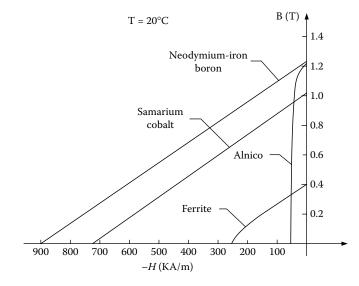
FIGURE 6.47 Demagnetization curves for different PM materials.
