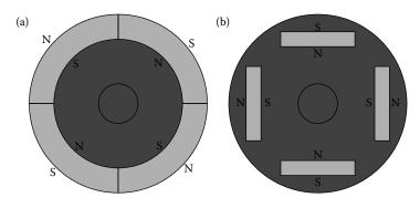
**FIGURE 6.43** Cross sectional view of the PM rotor: (a) surface-mounted PM rotor; and (b) interior-mounted PM rotor.
