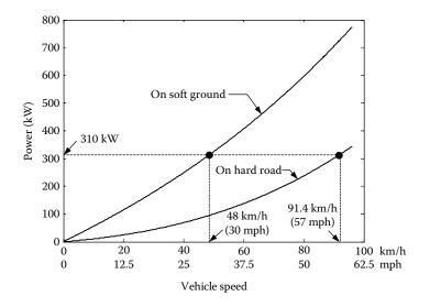
FIGURE 16.14 Traction power on hard road and soft ground at constant speeds.
