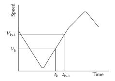
FIGURE 4.11 Acceleration being assumed constant with a short time period.
