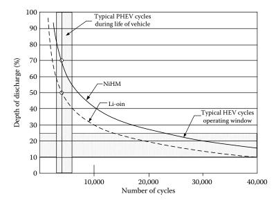
FIGURE 10.29 Cycle life characteristics of Varta energy storage technologies.<sup>5</sup>
