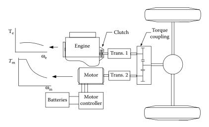
FIGURE 5.8 Two-shaft configuration.
