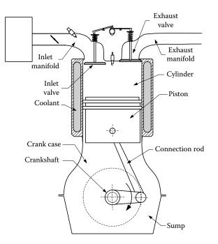
FIGURE 3.1 4S, SI gasoline engine.
