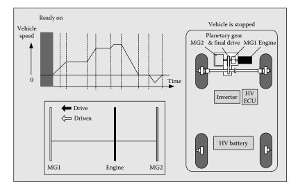
FIGURE A.13 Operation with stopped vehicle.
