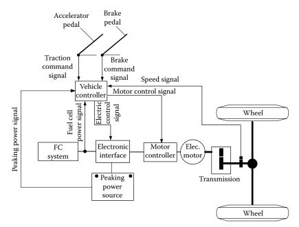
FIGURE 15.2 Configuration of a typical fuel cell hybrid drive train.
