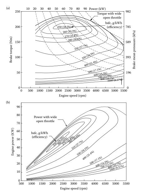
**FIGURE 3.6** Fuel consumption characteristics of a typical SI engine: (a) along with engine speed and torque and (b) along with engine speed and power.
