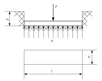
FIGURE 16.1 Terrain penetration test.
