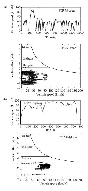
**FIGURE 4.12** Speed profile and tractive effort in different representative drive cycles; operating points are marked by '+': (a) FTP75 urban, (b) FTP75 highway, (c) US06, (d) J227a schedule B, (e) J227a schedule C, and (f) J227a schedule D.
