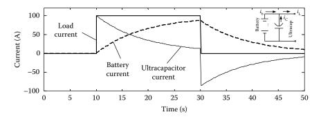
FIGURE 16.19 Current profiles of the battery/ultracapacitor energy storage.
