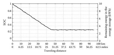
**FIGURE 10.6** SOC and the remaining energy in the energy storage versus traveling distance in FTP75 urban driving cycle with AER mode.
