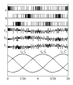
FIGURE 6.41 Current-controlled voltage source inverter (5% tolerance bandwidth).
