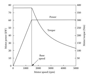
FIGURE 4.4 Typical variable-speed electric motor characteristics.
