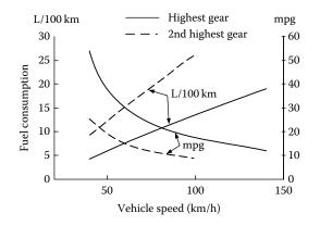
FIGURE 2.31 Fuel economy characteristics of a typical vehicle at constant speed.
