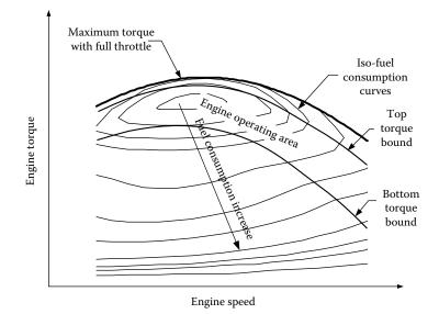
**FIGURE 10.16** Operation area of the engine in the CD mode.
