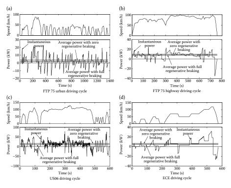
**FIGURE 7.20** Instantaneous power and average power with full and zero regenerative braking in typical drive cycles. (a) FTP75 urban, (b) FTP75 highway, (c) US06, and (d) ECE-15.
