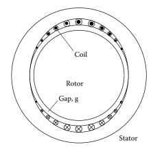
FIGURE 6.46 Winding configuration of sinusoidal-shaped back EMF BLDC.
