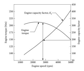
FIGURE 2.22 Capacity factor of a typical engine.
