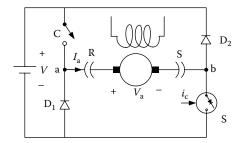
FIGURE 6.11 Forward motoring and regenerative braking control with a single chopper.
