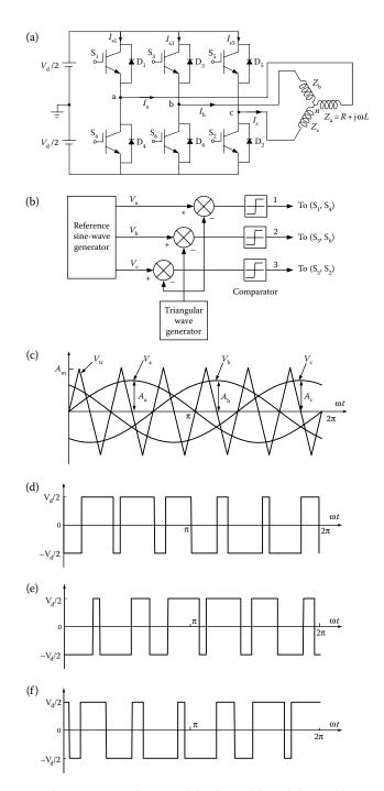
**FIGURE 6.21** DC/AC inverter with sinusoidal pulse-width modulation: (a) inverter topology; (b) control signals; (c) three phase reference voltage and triangular carrier waveforms; (d) voltage of phase a; (e) voltage of phase b; and (f) voltage of phase c.
