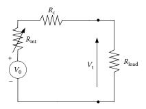
FIGURE 12.6 Battery circuit model.
