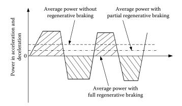
**FIGURE 7.19** Average power consumed in acceleration and deceleration with full, partial, and zero regenerative braking.
