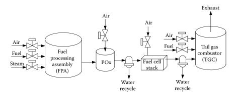
FIGURE 14.11 Fuel processing diagram.<sup>13</sup>
