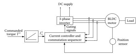
FIGURE 6.51 Block diagram of the torque control of the BLDC motor.
