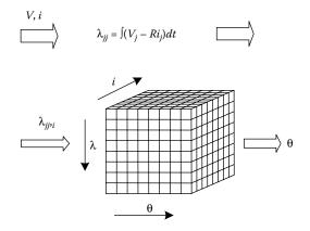
FIGURE 6.70 Flux linkage-based rotor position estimation method.
