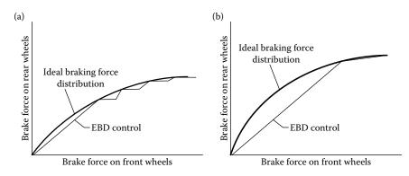
**FIGURE A.9** Braking force on the front and rear wheels: (a) without load on the rear wheels and (b) with load in the rear wheels.
