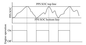
FIGURE 8.5 Illustration of engine on-off control strategy.
