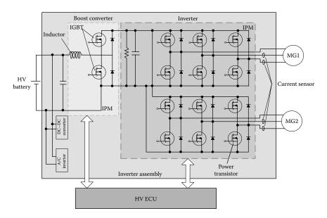
FIGURE A.5 Inverter assembly.
