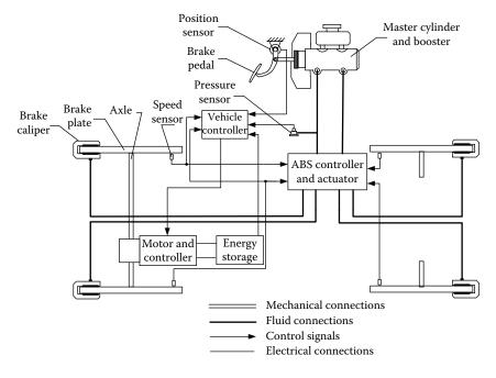
FIGURE 13.9 Schematic structure of the parallel hybrid brake system.
