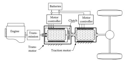
**FIGURE 5.25** Hybrid electric drive train with speed and torque coupling of a transmotor and single shaft.
