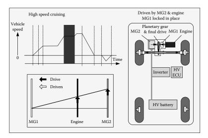
FIGURE A.19 Operation mode at high-speed cruising.
