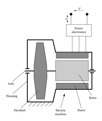
FIGURE 12.14 Basic structure of a typical flywheel system (mechanical battery).
