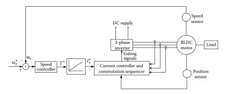
FIGURE 6.52 Block diagram of the speed control of the BLDC motor.
