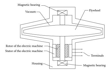
FIGURE 12.17 Basic structure of a typical flywheel system.
