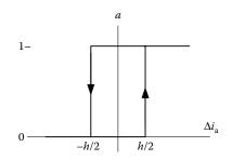
FIGURE 6.39 Input-output characteristics of a hysteresis current controller.
