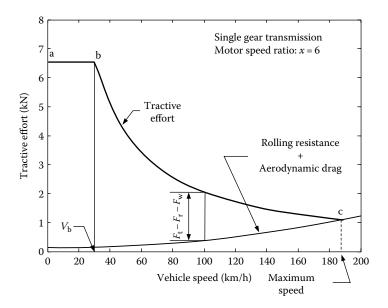
**FIGURE 4.8** Tractive effort versus vehicle speed with a traction motor of x = 6 and single-gear transmission.
