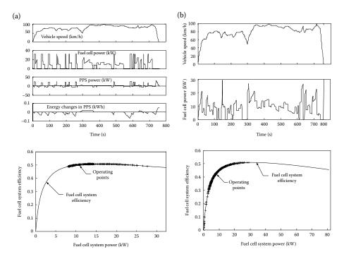
**FIGURE 15.9** Operating simulation of the fuel cell hybrid and fuel-cell-alone-powered passenger car in an FTP75 highway drive cycle: (a) hybrid drive train and (b) fuel-cell-alone-powered drive train.
