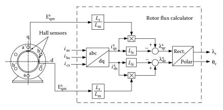
**FIGURE 6.30** Determination of the magnitude and position of the rotor flux vector using a Hall sensor and a rotor flux calculator.<sup>3</sup>
