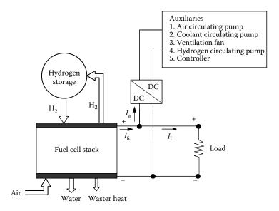
FIGURE 14.5 A hydrogen-air fuel cell system.
