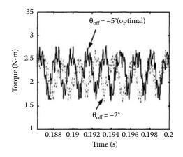
FIGURE 6.74 Developed torque before and after optimization.
