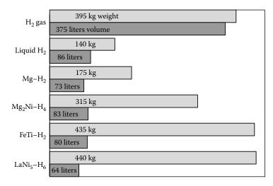
**FIGURE 14.10** Current mass and volume needed to store 6 kg of hydrogen (22 L of gasoline equivalent) in various hydrogen storage devices.<sup>14</sup>
