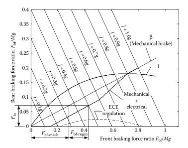
FIGURE 13.10 Braking forces varying with deceleration rate.
