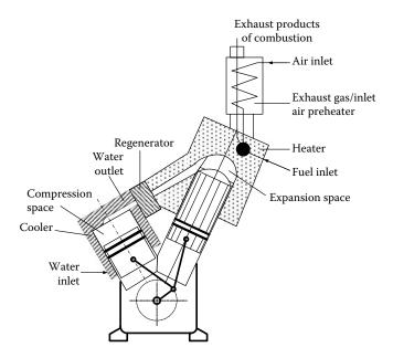
FIGURE 3.16 Diagram of a practical opposed-piston Stirling engine.
