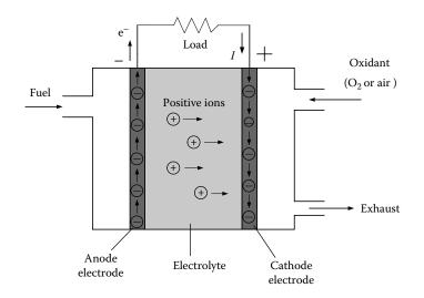
FIGURE 14.1 Basic operation of a fuel cell.
