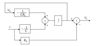
FIGURE 12.10 Block diagram of the ultracapacitor model.
