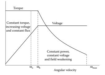
FIGURE 12.16 Typical torque and voltage profile versus rotational speed.
