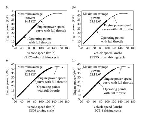
**FIGURE 8.14** Maximum possible operating points of the engine and maximum average power in typical drive cycles: (a) FTP75 urban, (b) FTP75 highway, (c) US06, and (d) ECE-15.
