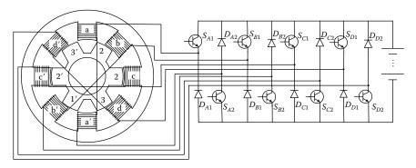
FIGURE 6.55 SRM and its power supply.
