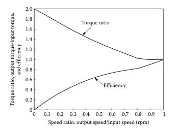
FIGURE 11.1 Characteristics of a typical dynamic hydraulic torque converter.
