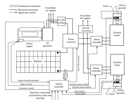
FIGURE 16.4 Tracked series hybrid off-road vehicle architecture.
