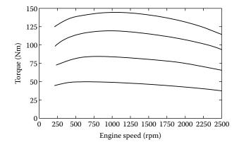
FIGURE 3.18 Torque/speed characteristics of typical Stirling engines.
