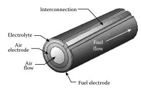
FIGURE 14.8 Tubular SOFC.
