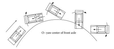
FIGURE 2.41 Loss of directional stability due to the lockup of rear wheels.
