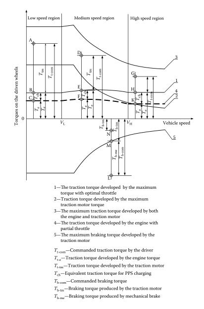
FIGURE 9.19 Schematic illustration of the MAX. SOC control strategy.
