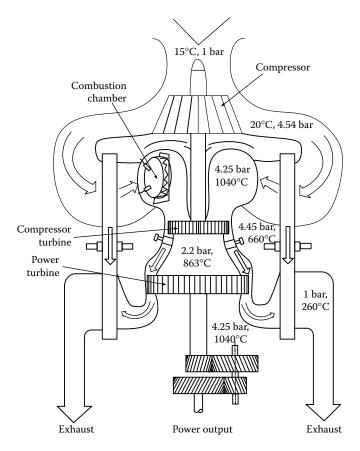
FIGURE 3.20 Gas turbine engine with heat exchanger.
