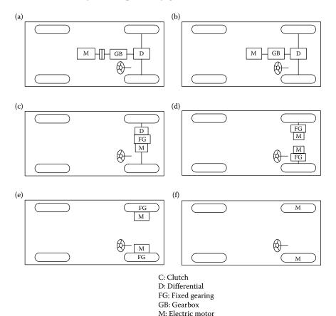
**FIGURE 4.3** Possible EV configuration: (a) conventional driveline with multigear transmission and clutch, (b) single-gear transmission without need of a clutch, (c) integrated fixed gearing and differential, (d) two separate motors and fixed gearing with their driveshaft, (e) direct drive with two separate motors and fixed gearing, and (f) two separate in-wheel motor drives.<sup>1</sup>
