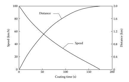
FIGURE 13.1 Coasting speed and distance.
