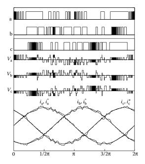
FIGURE 6.40 Current-controlled voltage source inverter (10% tolerance bandwidth).
