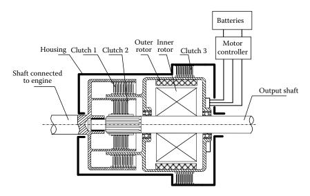
FIGURE 5.20 Implementation of speed coupling with a transmotor.
