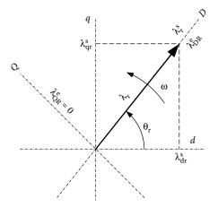
FIGURE 6.28 Orientation of the excitation reference frame along the rotor flux vector.
