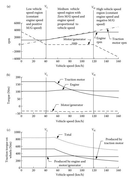
**FIGURE 9.18** Torques and speeds of the engine, traction motor, motor/generator, and driven wheels with full engine throttle opening and full loading of the traction motor along vehicle speed: (a) speeds, (b) torques of the power plants, and (c) torques on the driven wheels.
