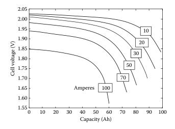
FIGURE 12.3 Discharge characteristics of a lead-acid battery.
