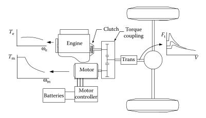
FIGURE 5.10 Two-shaft configuration.
