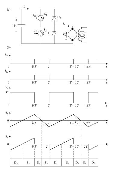
**FIGURE 6.12** Forward motoring and regenerative braking control using class C two-quadrant chopper: (a) chopper circuit; (b) waveforms.
