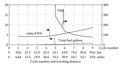
**FIGURE 10.9** Fuel and electric energy consumption versus the number of FTP75 urban driving cycle and traveling distance with AER mode in English unit.
