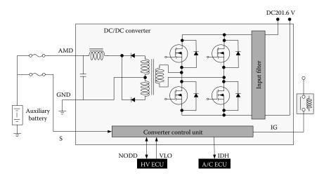
FIGURE A.6 DC–DC converter.
