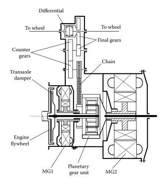
FIGURE A.2 Schematic illustration of the hybrid transaxle.
