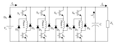
FIGURE 6.68 A driving circuit example for the SRG.
