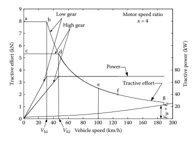
FIGURE 7.14 Speed-torque (power) characteristics of an electric motor.
