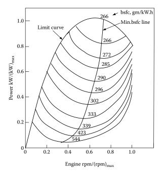
FIGURE 3.22 Fuel consumption characteristics of a Chrysler upgraded turbine.
