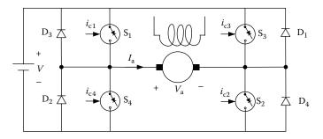
FIGURE 6.13 Class E four-quadrant chopper.
