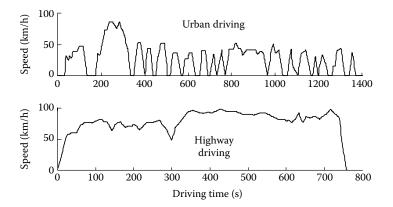
FIGURE 2.33 EPA FTP75 urban and highway drive cycles.
