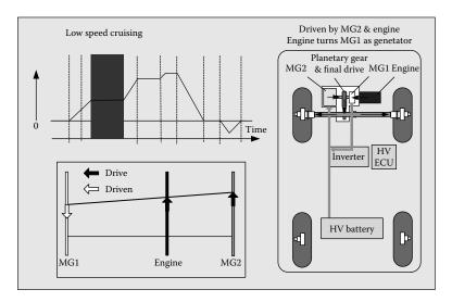
FIGURE A.17 Operation mode of low-speed cruising.
