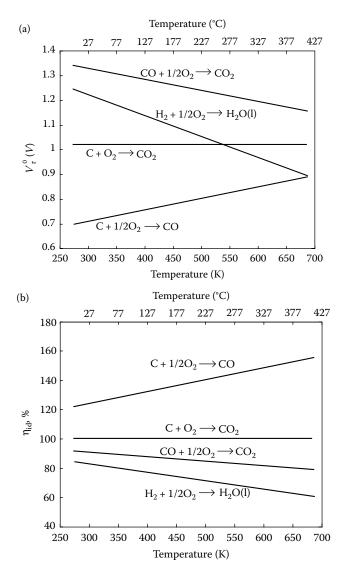
FIGURE 14.2 Temperature dependence of cell voltage (a) and reversible efficiency (b).
