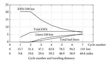
**FIGURE 10.14** Fuel and electric energy consumption versus the number of LA92 driving cycle and traveling distance with AER mode in metric unit.
