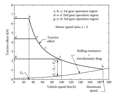
**FIGURE 4.6** Tractive effort versus vehicle speed with a traction motor of x = 2 and three-gear transmission.
