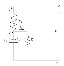
FIGURE 12.9 Ultracapacitor equivalent circuit.
