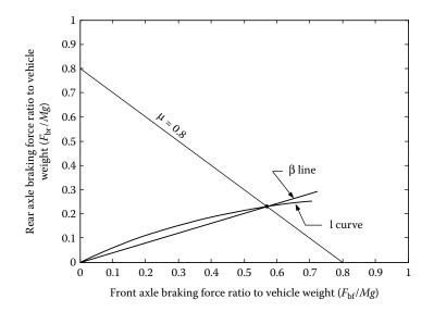
FIGURE 2.40 Ideal and actual braking force distribution curves.
