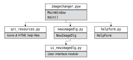
Figure 6.2 The Image Changer's modules, classes, and functions
