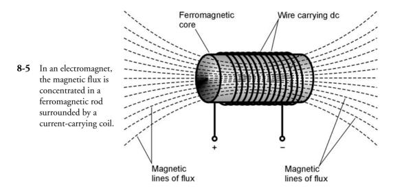
Direct-current electromagnets have defined north and south poles, just like permanent magnets. The main difference is that an electromagnet can get much stronger than any permanent magnet. You will see evidence of this if you do the preceding experiment with a large enough bolt and enough turns of wire.
