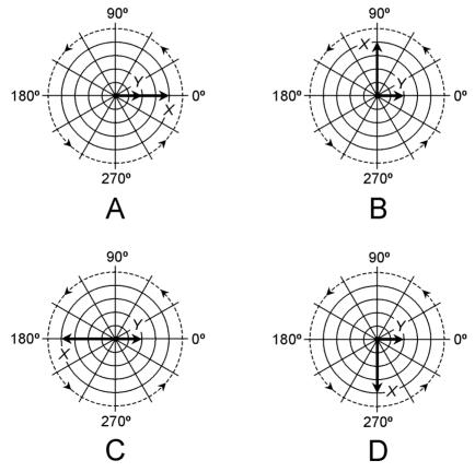
12-11 Vector representations of phase difference. At A, waves X and Y are in phase. At B, X leads Y by 90°. At C, X and Y are 180° out of phase. At D, X lags Y by 90°. Time is represented by counterclockwise motion of both vectors at a constant angular speed.
