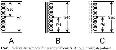
At B, laminated iron core, step-up. At C, ferrite or powdered iron core, step-up.
