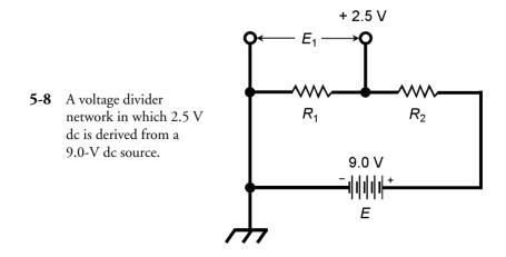
make *R* equal to 1000  $\Omega$ . This means *R*<sub>1</sub> must be 280  $\Omega$  in order to get the ratio *R*<sub>1</sub>:*R* = 0.28. The value of *R*<sub>2</sub> is the difference between *R* and *R*<sub>1</sub>. That is 1000 – 280 = 720  $\Omega$ .
