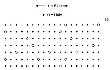
**19-2** Pictorial representation of hole flow. Solid black dots represent electrons, moving in one direction. Open circles represent holes, moving in the opposite direction.
