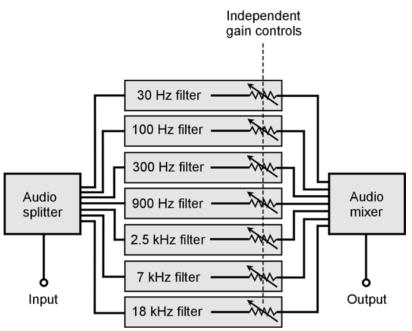
**31-4** A graphic equalizer consists of an audio splitter, several bandstop filters, several gain controls, and an audio mixer.
