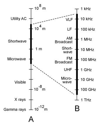
**25-10** At A, the EM spectrum from  $10^8$  m to  $10^{-12}$  m, with each vertical division representing two orders of magnitude (an increase or decrease of the wavelength by a factor of 100). At B, the RF spectrum, with each vertical division representing one order of magnitude (an increase or decrease of the frequency by a factor of 10).
