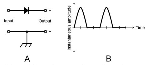
**20-1** At A, a half-wave rectifier circuit. At B, the output of the circuit shown at A when an ac sine wave is applied to the input.
