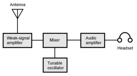
25-11 Block diagram of a direct-conversion receiver.
