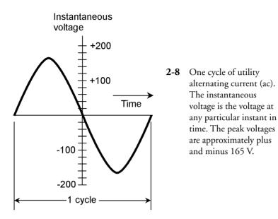
Because the whole cycle repeats itself every 1/60 second, the *frequency* of the utility ac wave is said to be 60 *hertz*, abbreviated 60 Hz. The German word *hertz* literally translates to "cycles per second." In the United States, this is the standard frequency for ac. In some places it is 50 Hz.
