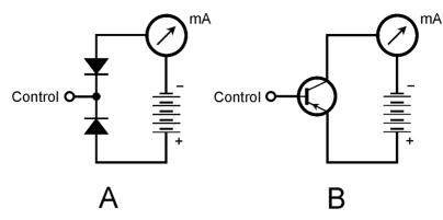
**22-5** At A, the dual-diode model of a simple PNP circuit. At B, the actual transistor circuit.
