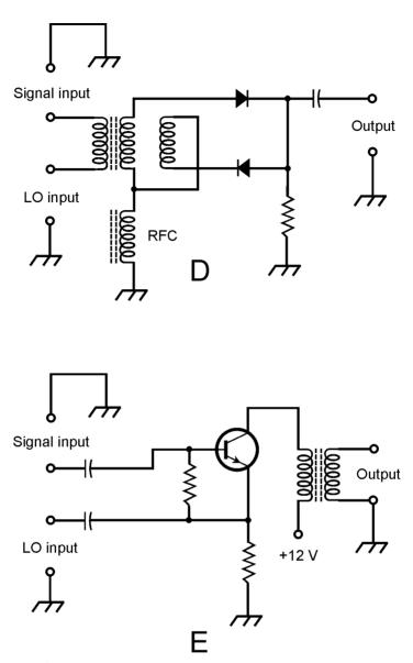
**25-14** At D, a product detector using diodes. At E, a product detector using an NPN bipolar transistor biased as a class B amplifier. Both of these circuits can also be used as signal mixers.
