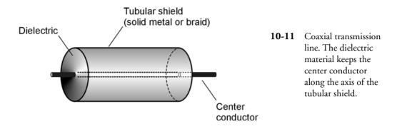
tervals to the wires, or by a solid web of polyethylene. The substance separating the wires is called the *dielectric* of the transmission line. A coaxial transmission line has a wire conductor surrounded by a tubular braid or pipe (Fig. 10-11). The wire is kept at the center of this tubular *shield* by means of polyethylene beads, or more often, by solid or foamed polyethylene, all along the length of the line.
