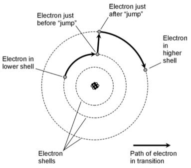
**1-2** Electrons move around the nucleus of an atom at defined levels, called *shells*, which correspond to discrete energy states. This is a simplified illustration of an electron gaining energy within an atom.
