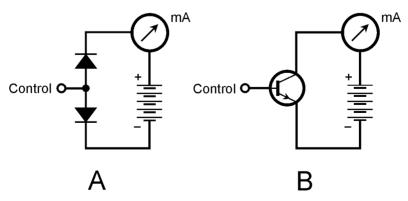
**22-3** At A, the dual-diode model of a simple NPN circuit. At B, the actual transistor circuit.
