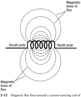
wire. The flux lines converge at the magnetic poles.
