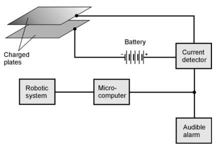
34-1 Simplified functional diagram of a smoke detector.
