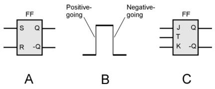
**26-3** At A, the symbol for an R-S flip-flop. At B, pulse edges are either negative-going or positive-going. At C, the symbol for a J-K flip-flop.
