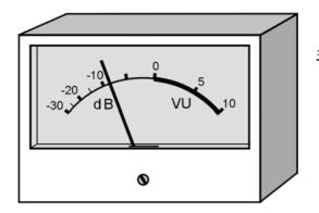
**3-12** A VU (volume-unit) meter. The heavy portion of the scale (to the right of 0) is usually red, indicating the risk of audio distortion.
