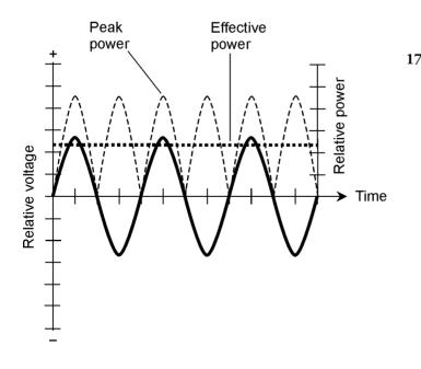
17-2 Peak versus effective power for a sine wave. The left-hand vertical scale shows relative voltage. The righthand vertical scale shows relative power. The solid curve represents the voltage as a function of time. The light and heavy dashed waves show peak and effective power, respectively, as functions of time.
