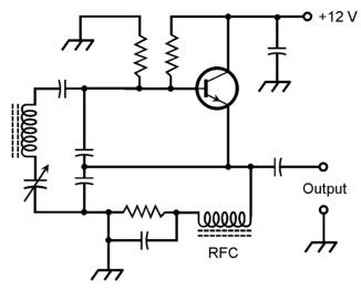
**24-15** A series-tuned Colpitts oscillator, also known as a Clapp oscillator. This circuit uses an NPN bipolar transistor.
