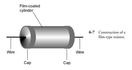
The cylindrical form is made of an insulating substance, such as porcelain. The film is deposited on this form by various methods, and the value tailored as desired. Metal-film resistors can be made to have nearly exact values. Film-type resistors usually have low to medium-high resistance.
