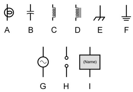
**4-4** Schematic symbols for incandescent lamp (A), fixed capacitor (B), fixed inductor with air core (C), fixed inductor with laminated-iron core (D), chassis ground (E), earth ground (F), signal generator or source of alternating current (G), pair of terminals (H), and specialized component or device (I).
