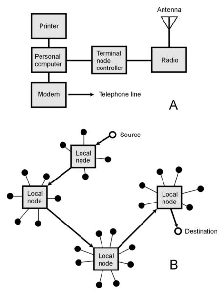
**26-6** At A, a packet-wireless station. At B, passage of a packet through nodes in a wireless communications circuit.
