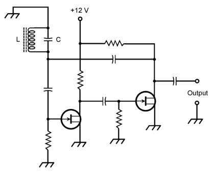
**24-19** A multivibrator audio oscillator using two N-channel JFETs. The frequency is determined by the value of the inductor L and the capacitor C.
