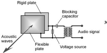
**30-2** Functional diagram of an electrostatic sound transducer.
