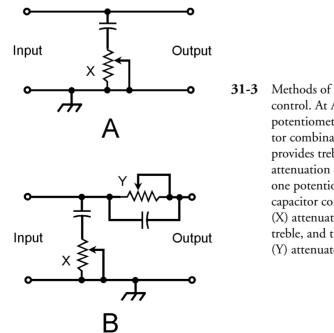
Methods of tone control. At A, a single potentiometer/capacitor combination (X) provides treble attenuation only. At B, one potentiometer/ capacitor combination (X) attenuates the treble, and the other (Y) attenuates the bass.
