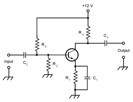
**22-9** Common emitter configuration. This diagram shows an NPN transistor circuit.
