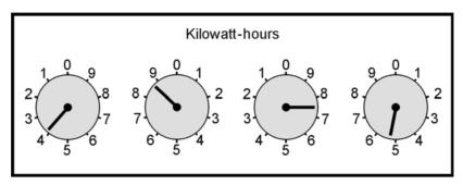
**3-11** A utility meter with four rotary analog dials. In this example, the reading is a little more than 3875 kWh.
