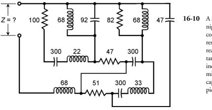
A series-parallel nightmare circuit containing multiple resistances and reactances. Resistances are in ohms; inductances are in microhenrys (µH); capacitances are in picofarads (pF).
