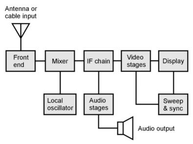
**25-15** Block diagram of a conventional FSTV receiver.
