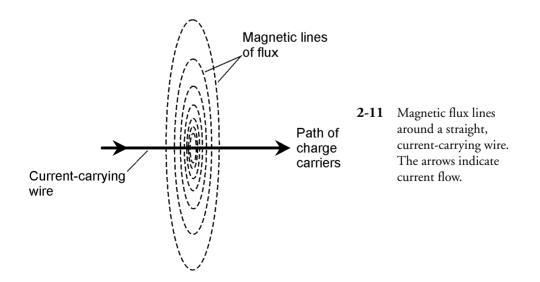
resent the magnetic field.) You'll sometimes hear or read about a certain number of flux lines per unit cross-sectional area, such as 100 lines per square centimeter. This is a relative way of talking about the intensity of the magnetic field.
