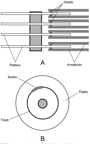
**33-2** At A, an edgewise view of a hard drive, showing four platters. At B, a broadside view of a platter, showing one track and one sector.
