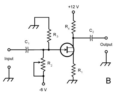
**23-4** Two methods of biasing an N-channel JFET. At A, fixed gate bias; at B, variable gate bias.
