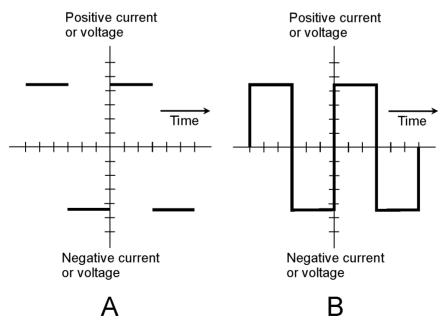
**9-2** At A, a perfect square wave; the transitions are instantaneous and therefore do not show up on the graph. At B, the more common rendition of a square wave, showing the transitions as vertical lines.
