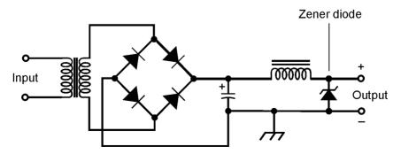
**21-8** A power supply with a Zener-diode voltage regulator in the output.
