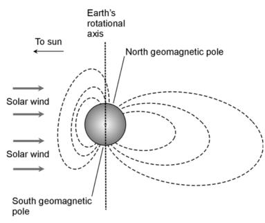
**8-1** Geomagnetic flux lines (dashed curves) are distorted by the solar wind, so the geomagnetic field is not symmetrical with respect to the earth.
