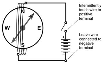
3-1 A simple galvanometer. The compass must lie flat.
