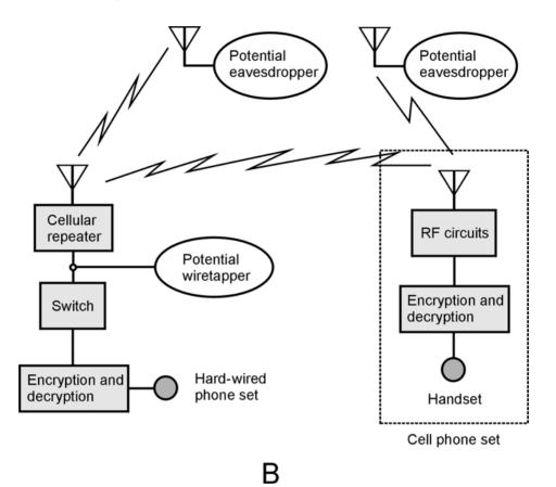
**32-7B** End-to-end encryption. Heavy, straight lines represent wires or cables; zigzag lines represent RF signals.
