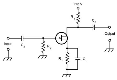
**23-11** Common source configuration. This diagram shows an N-channel JFET circuit.
