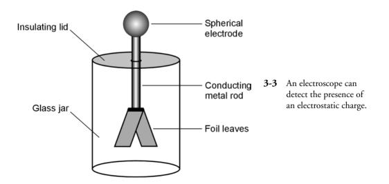
If you have access to a laboratory electroscope, try charging it up with a glass rod that has been rubbed against a cloth. When the rod is pulled away from the electroscope, the foil leaves remain standing apart. The charge just sits there! If the electroscope drew any current, the leaves would fall back together again, just as the galvanometer compass needle returns to magnetic north the instant you take the wire from the battery.
