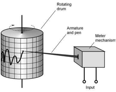
**3-15** A functional drawing of a pen recorder.
