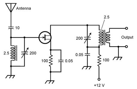
24-9 A tuned RF amplifier for use at about 10 MHz. Resistances are in ohms. Capacitances are in microfarads (μF) if less than 1, and in picofarads (pF) if more than 1. Inductances are in microhenrys (μH).
