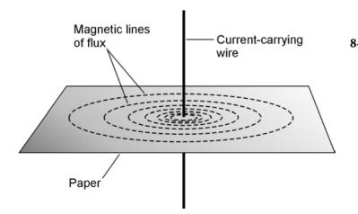
8-3 The pattern of magnetic flux lines (dashed curves) around a straight, currentcarrying wire can be seen when the wire passes through a horizontal sheet of paper sprinkled with iron filings.
