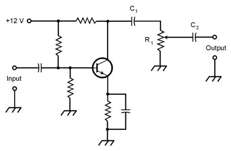
24-7 A basic volume control (potentiometer  $R_1$ ) can be used to vary the gain in a low-power audio amplifier.
