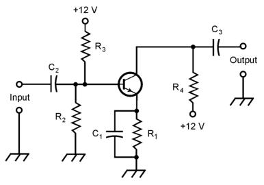
**24-1** An amplifier circuit with a bipolar transistor. Component designators are discussed in the text.
