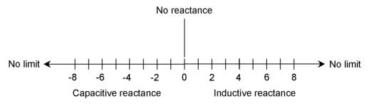
**14-1** Inductive and capacitive reactance can be represented as numerical values (corresponding to ohms multiplied by *j*) along a number line.
