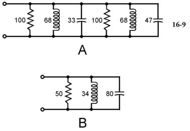
At A, a complicated parallel circuit containing multiple resistances and reactances. At B, the same circuit simplified. Resistances are in ohms; inductances are in microhenrys (μH); capacitances are in picofarads (pF).
