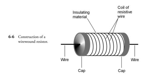
Wirewound resistors can be manufactured to have values within a very close range. They are *precision components*. Also, wirewound resistors can be made to handle large amounts of power. A disadvantage of wirewound resistors, in some applications, is that they act like inductors. This makes them unsuitable for use in most radio-frequency circuits. Wirewound resistors usually have low to moderate values of resistance.
