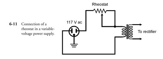
Rheostats are used in high-voltage, high-power applications. A good example is in a variablevoltage power supply. This kind of supply uses a transformer that steps up the voltage from the 117-V utility mains, and diodes to change the ac to dc. The rheostat can be placed between the utility outlet and the transformer (Fig. 6-11). This results in a variable voltage at the power-supply output.
