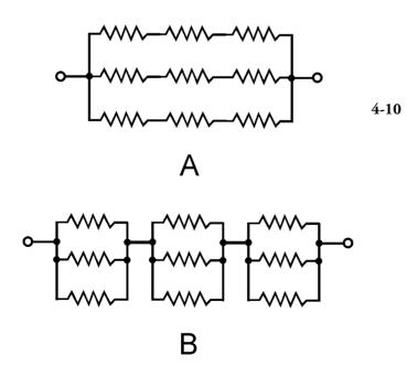
Series-parallel resistances. At A, sets of series resistors are connected in parallel. At B, sets of parallel resistances are connected in series. These examples show symmetrical *n*-by-*n* matrices with *n* = 3.
