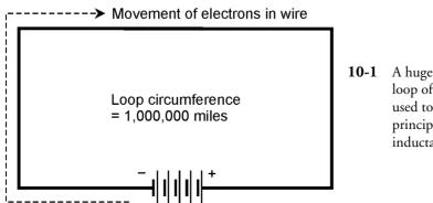
A huge, imaginary loop of wire can be used to illustrate the principle of inductance.
