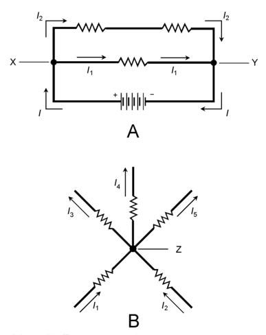
5-5 Kirchhoff's First Law. At A, the current into point X or point Y is the same as the current out of that point. That is,  $I = I_1 + I_2$ . At B, the current into point Z equals the current flowing out of point Z. That is,  $I_1 + I_2 = I_3 + I_4 + I_5$ . Illustration for Quiz Questions 13 and 14.
