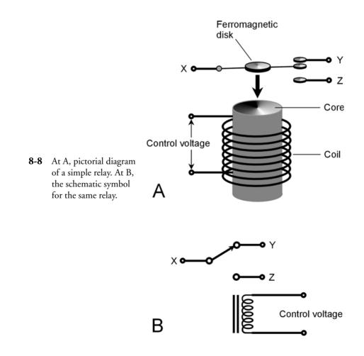
Some relays have several sets of contacts. Some relays are meant to remain in one state (either with current or without) for a long time, while others are meant to switch several times per second. The fastest relays can operate several dozen times per second. In recent years, relays have been largely supplanted by switching transistors and diodes, except in applications where extremely high current or high voltage is involved.
