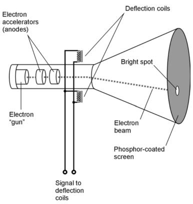
**29-6** Simplified cross-sectional rendition of an electromagnetic CRT.
