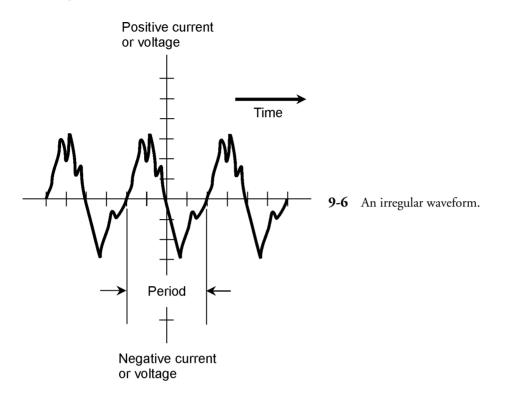
pens, the *frequency spectrum* of the wave is multifaceted. That means the wave energy is split up more or less equally among multiple frequencies.
