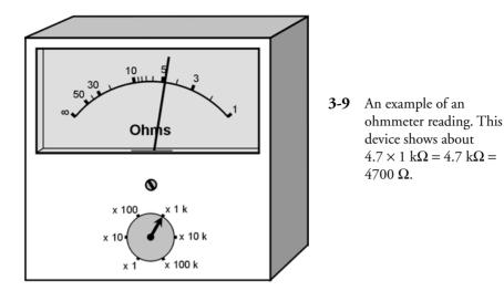
"more than infinity" ohms! The needle will hit the pin at the left end of the scale. Therefore, when using an ohmmeter to measure resistance, you must always be sure that there is no voltage between the points under test. The best way to do this is to switch off the equipment in question.
