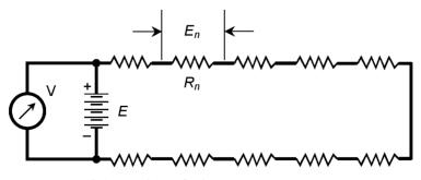
**5-2** Analysis of voltages in a series circuit.
