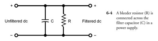
It's a good idea to short out all filter capacitors, using a screwdriver with an insulated handle and wearing heavy, insulated gloves, before working on a dc power supply. Even if the supply has bleeder resistors, they might take a while to get rid of the residual charge. In addition, bleeder resistors can, and sometimes do, fail.
