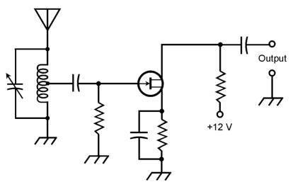
25-13 A tunable FET preamplifier for use in a radio receiver.
