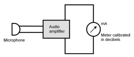
**3-13** A meter for measuring sound levels. The output of the audio amplifier is rectified to produce dc that the meter can detect.
