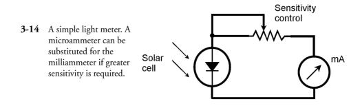
One problem with this design is that solar cells are not sensitive to light at exactly the same wavelengths as human eyes. This can be overcome by placing a colored filter in front of the solar cell, so that the solar cell becomes sensitive to the same wavelengths, in the same proportions, as human eyes. Another problem is calibrating the meter. This must usually be done at the factory, in standard illumination units such as *lumens* or *candela*.
