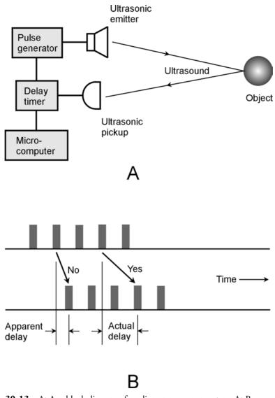
**30-13** At A, a block diagram of medium-range sonar system. At B, a sonar system can be confused by long delays.
