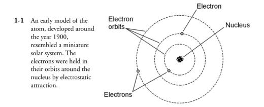
Electrons can move rather easily from one atom to another in some materials. In other substances, it is difficult to get electrons to move. But in any case, it is far easier to move electrons than it is to move protons. Electricity almost always results, in some way, from the motion of electrons in a material. Electrons are much lighter than protons or neutrons. In fact, compared to the nucleus of an atom, the electrons weigh practically nothing.
