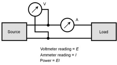
**17-9** Power measurement in a transmission line. Ideally, the voltage and the current should be measured at the same physical point on the line.
