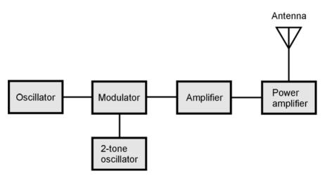
25-1 Simplified block diagram of an AFSK transmitter.
