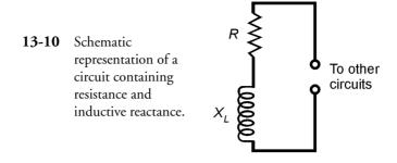
decreases until it is comparable to the loss resistance R in the coil winding. In either case, the situation can be schematically represented by an inductance in series with a resistance (Fig. 13-10).
