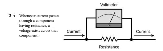
Just as there is no such thing as a perfectly resistance-free substance, there isn't a truly infinite resistance, either. Even air conducts to some extent, although the effect is usually so small that it can be ignored. In some electronic applications, materials are selected on the basis of how "nearly infinite" their resistance is.
