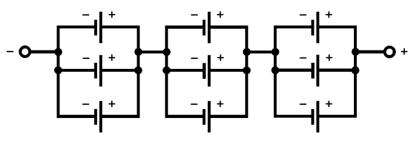
7-6 Connection of cells in series-parallel.
