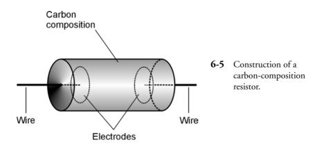
of carbon to the nonconducting material, and also on the physical distance between the wire leads. This results in a *carbon-composition resistor*.
