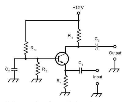
**22-10** Common base configuration. This diagram shows an NPN transistor circuit.
